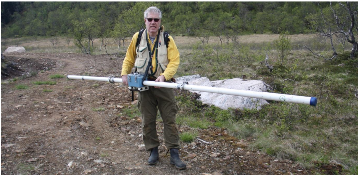
Figure 4.2: Geonics EM31 used in graphite investigations in Vesterålen.
