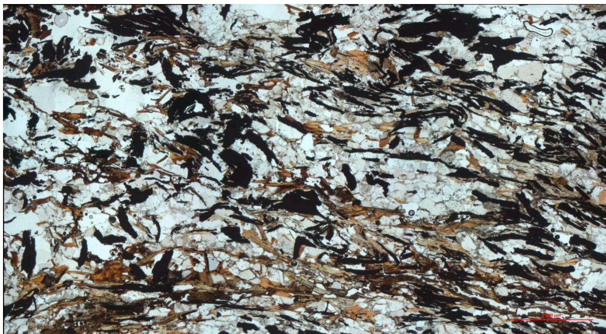
Figure 6.7: Example of thin section from Hesten (Sample HG39-16), with typical flake graphite flake size from about 0.01 mm up to about 0.5 cm
