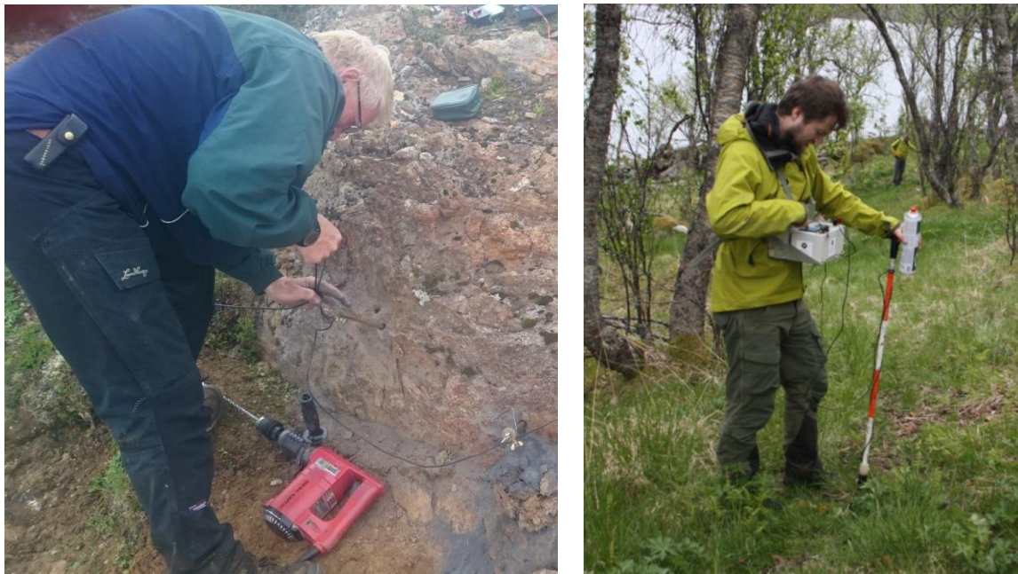
Figure 4.4: Establishing CP ore grounding point and data acquisition in combined CP and SP measurements.
