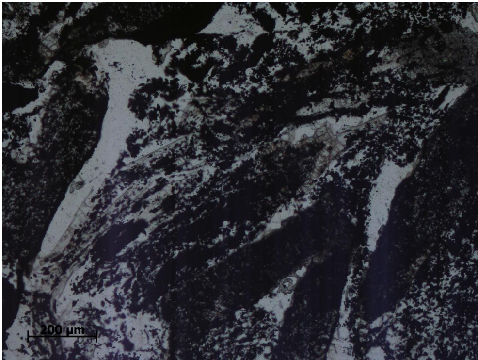
Figure 11.7: Micro-photo of thin section from Finngammen (BD Kvæ1813, 21.1 % TC, 21.0% TOC), show the fine-grained nature of the graphite flakes, typical for graphite that the industry classifies as amorphous.
