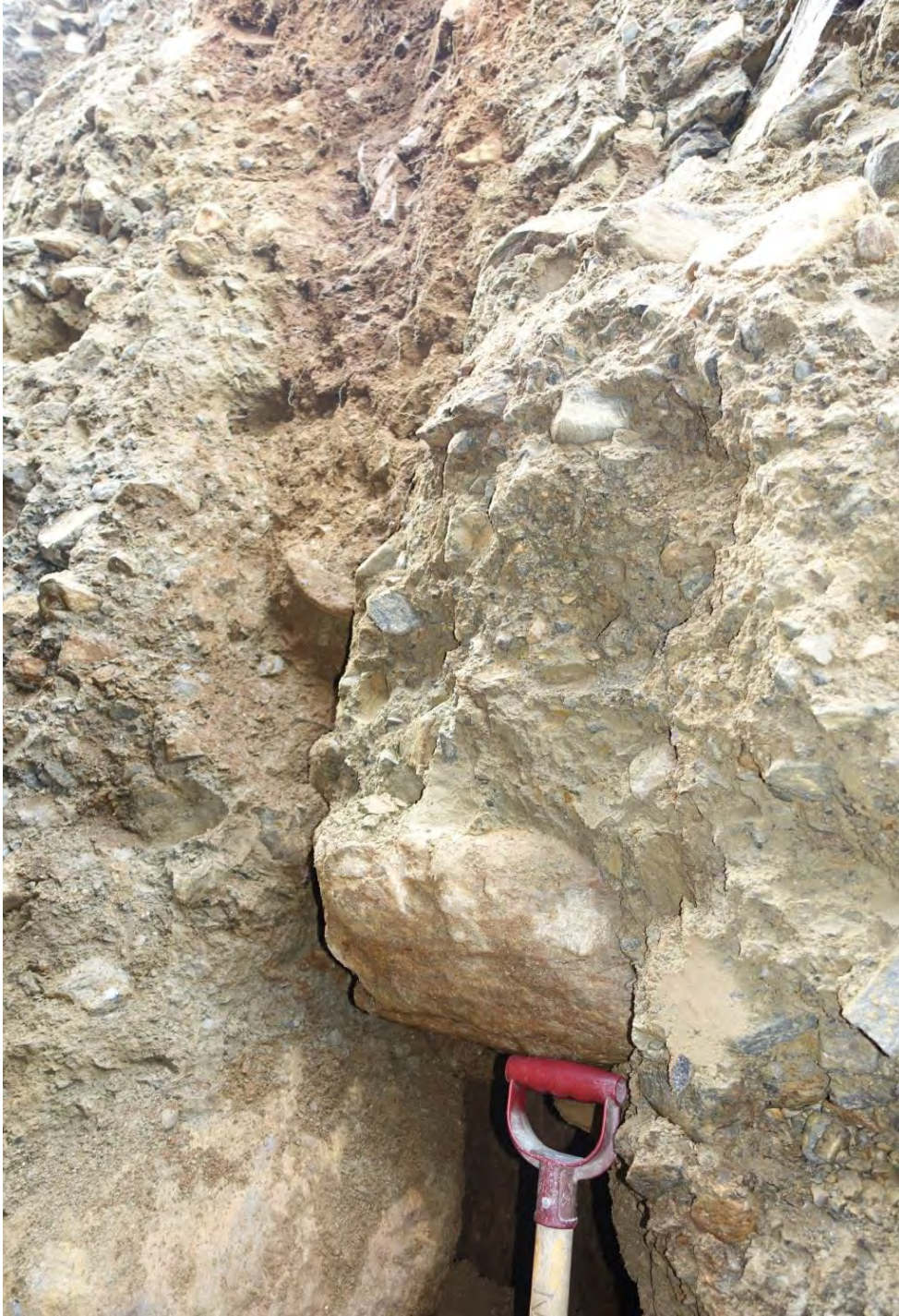
Figure 8. Cavity under coarse clast material at depth in sediment wedge filling the fault crevice recorded in trench 1.
