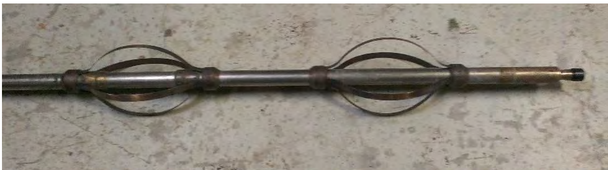
Figure 11. Two non-magnetic centralizers were manufactured at LTU before testing, here mounted on the Geovista BHTV (cf. 4).
