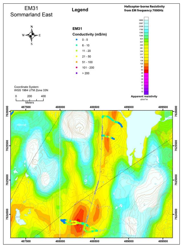
Figure 6.17: Sommarland East. Results from EM31 measurements overlain on top of helicopterborne measurements of apparent resistivity from EM 7000 Hz coaxial coil configuration.
