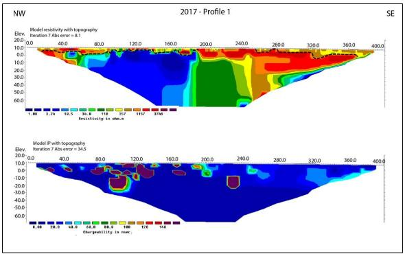
Figure 10.4: The Vikeid area. The results of the 2D Resistivity and Induced Polarisation measurements along profile 2017-1. The interpreted soil-bedrock interface as dotted black line.
