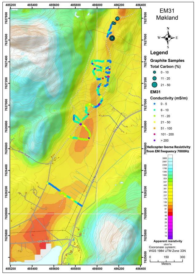
Figure 8.2: The southern part of the Møkland area. Results from EM31 measurements overlain on top of helicopter-borne measurements of apparent resistivity from EM 7000 Hz coaxial coil configuration.
