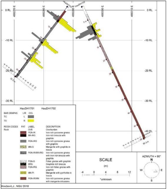
Figure 7.6: Lithological log and a graphical display of Total Carbon (TC in %) and Total Sulphur (TS in %) for the two drill holes at Haugsnes undertaken in 2017 (Haug1701 and Haug1702). View from the south.
