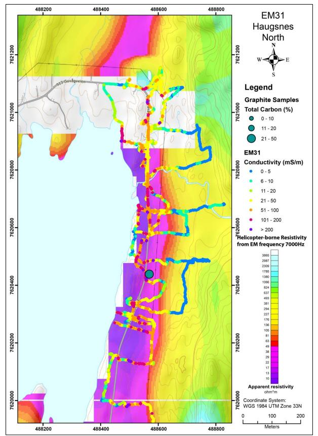
Figure 7.1: The northern part of Haugsnes. Results from EM31 measurements overlain on top of helicopter-borne measurements of apparent resistivity from EM 7000 Hz coaxial coil configuration.
