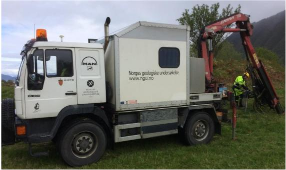
Figure 4.6: NGUs truck mounted drilling gear in operation.
