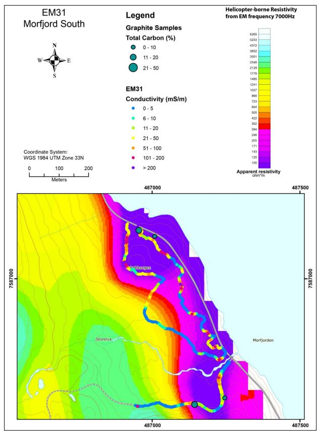
Figure 11.1: The Morfjord abandoned graphite mine. The results from the EM31 measurements and graphite showings overlain on top of helicopter-borne measurements of apparent resistivity from EM 7000 Hz coaxial coil configuration.
