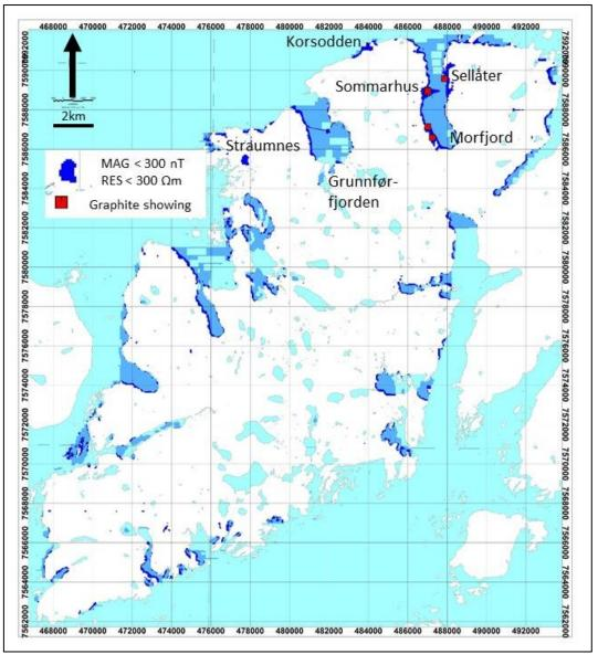
Figure 5.10: The blue colour shows areas at Austvågøya where apparent resistivity from EM 7000 Hz coaxial coils are < 300  $\Omega$ m and magnetic total field is < IGRF + 300 nT. The red squares are samples of graphite bearing rock.
