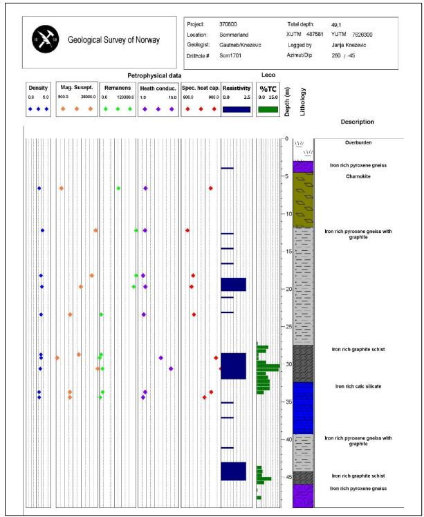
Figure 12.8: The petrophysical data and lithological log of the SOM1701 drill cores.
