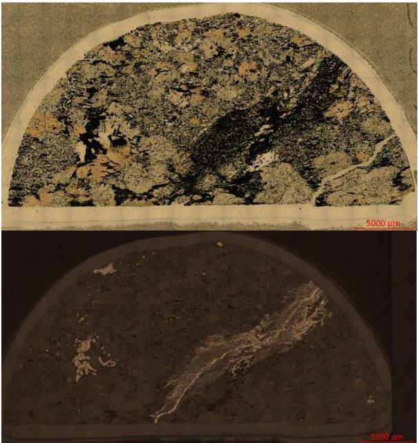
Figure 6.14: Thin section (JK-DhSom1-29.15) showing disseminated graphite with pyrrhotite vein, TC = 1,31% and TS = 2,32% (29-29,5m)
