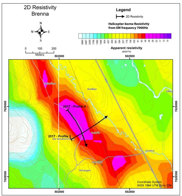
Figure 10.8: The Brenna area. The location of the 2D Resistivity/IP profile overlain on top of helicopter-borne measurements of apparent resistivity from EM 7000 Hz coaxial coil configuration.
