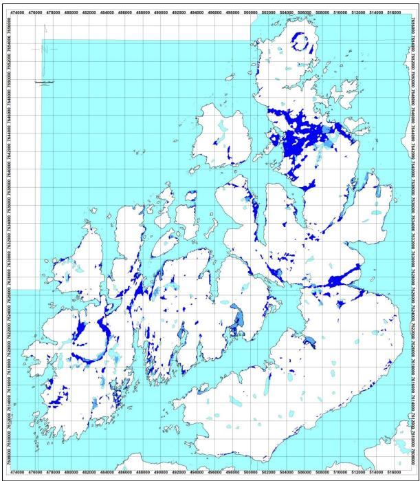
Figure 5.5: Blue colour show areas at Langøya where apparent resistivity from EM 7000 Hz coaxial coils is < 300  $\Omega$ m and magnetic total field is < IGRF + 300 nT.
