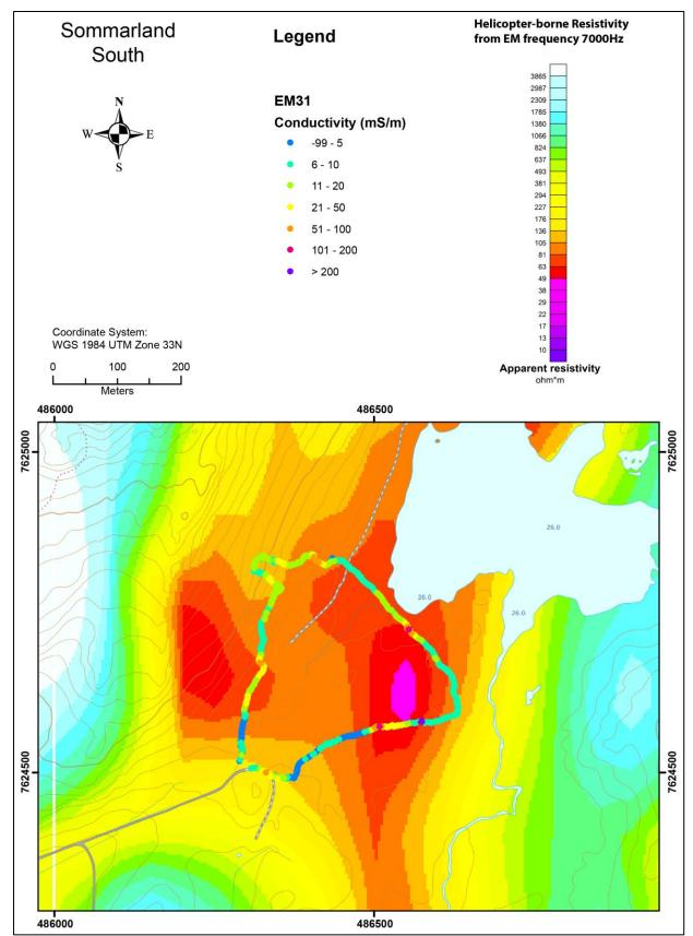
Figure 6.18: Sommarland South. Results from EM31 measurements overlain on top of helicopter-borne measurements of apparent resistivity from EM 7000 Hz coaxial coil configuration.
