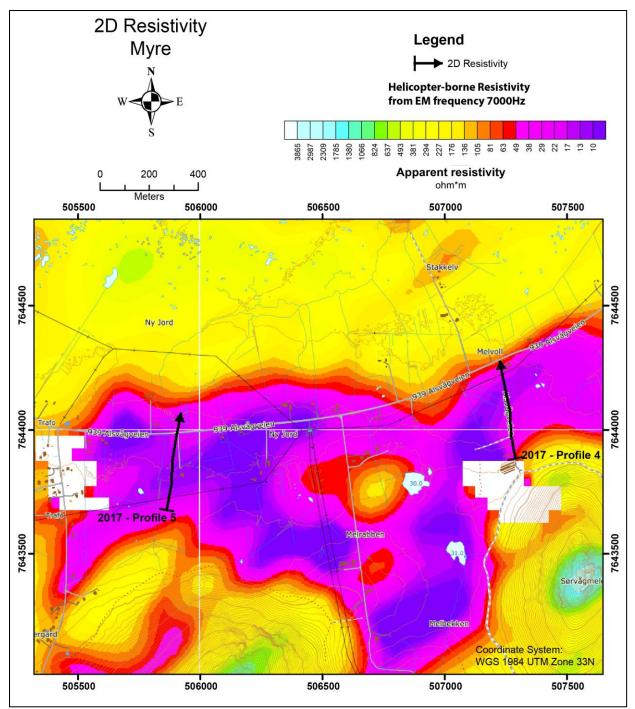
Figure 9.3: The area east of Myre. The location of 2D Resistivity/IP profiles overlain on top of helicopter-borne measurements of apparent resistivity from EM 7000 Hz coaxial coil configuration.
