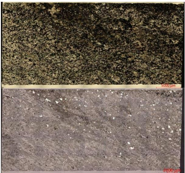
Figure 6.15: Thin section (Hg-DhSom1702-15.22) of the richest graphite interval, iron rich graphite schist with TC12,4%, TS 3,83% (15-15,5m).
