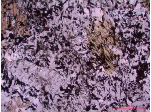
Figure 12.1: Thin section of graphite schist with a large crystal of clinozoisite in the lower left corner (Hg11-17).
