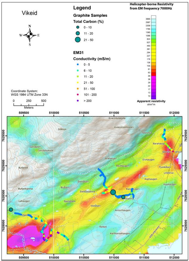
Figure 10.2: Results from EM31 measurements at Vikeid and graphite showings overlain on top of helicopter-borne measurements of apparent resistivity from EM 7000 Hz coaxial coil configuration.
