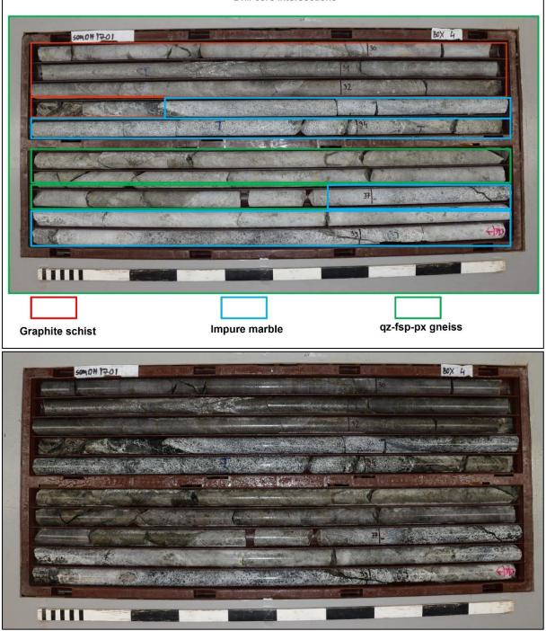
Figure 6.9: Part of drill core (dry upper and wet lower picture) showing a sequence with graphite schist, impure marble (calc-silicate rock) and quartz-feldspar-pyroxene gneiss. Appendix 3 show pictures of all drill cores from 2017 drilling.
