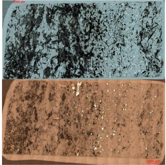
Figure 7.11: Gneiss with graphite flakes up to 2 mm and spotted pyrrhotite and pyrite in thin section JK-DhHau1702-5.57, (upper picture transmitted light, lower picture reflected light).
