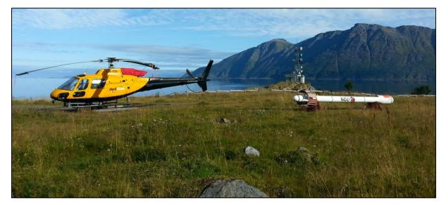
Figure 4.1: The equipment used in the helicopter-borne geophysical survey in Vesterålen and Lofoten.
