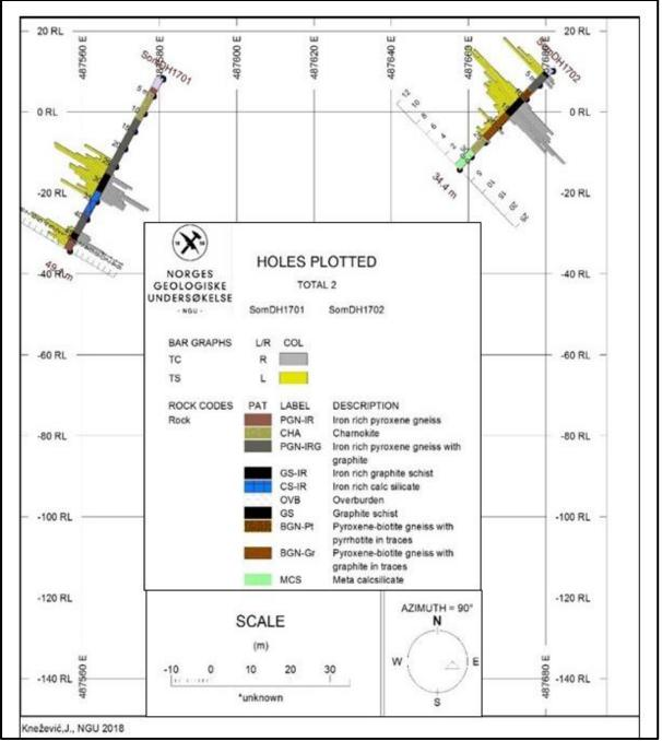
Figure 6.6: Lithological log and a graphical display of Total Carbon (TC in %) and Total Sulphur (TS in %) for the two drill holes at Sommarland acquired in 2017 (Som1701 and Som1702) seen from the south.
