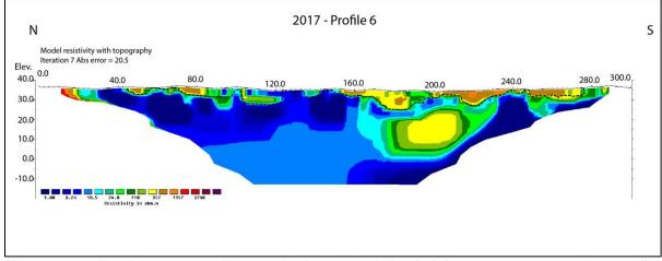
Figure 10.10: The Brenna area. The results from the 2D Resistivity measurements along profile 2017-6. The interpreted soil-bedrock interface is shown as a dotted black line.
