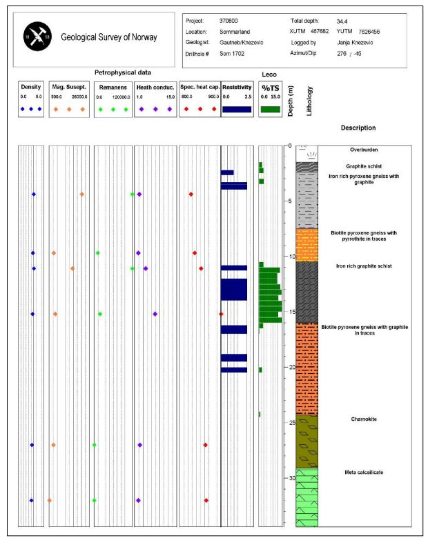
Figure 12.9: The petrophysical data and lithological log of the SOM1702 drill cores.
