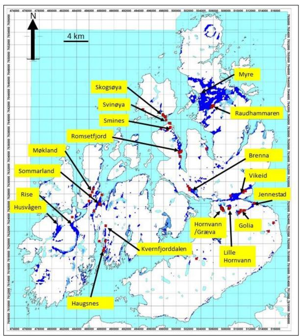
Figure 5.6: Blue colour show areas at Langøya where apparent resistivity from EM 7000 Hz coaxial coils is < 300  $\Omega$ m and magnetic anomaly field is < 300 nT. Red squares are samples of graphite bearing rock.
