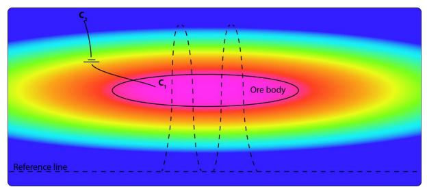
Figure 4.3: Conceptual illustration of the CP- method. The current electrode ( $C_1$ ) is connected to the ore body and the remote electrode ( $C_2$ ) is placed far outside the survey area. The colour indicates the strength of the charged potential above an ore-body. The dashed line shows the survey path which will the entire body.
