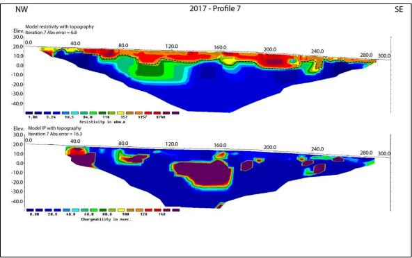
Figure 10.6: The Vikeid area. The results of the 2D Resistivity and Induced Polarisation measurements along profile 2017-7. The interpreted soil-bedrock interface as dotted black line.
