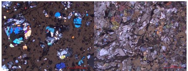
Figure 7.10: Left: Brecciated rock-type with fragments of silicate minerals (feldspars, quartz, pyroxene) with graphite in a groundmass of pyrrhotite. Right: Example where the proportion of silicates is higher and less brecciated. Graphite occurs both in pyrrhotite and in silicates. Thin section HG-DhHau1701-6.5 and JK-DhHau22.55 (combined reflected and polarized light).
