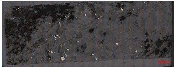
Figure 7.12: Mafic vein with graphite and pyrrhotite and partly disseminated graphite, thin section JK-DhHau1701-13.6.
