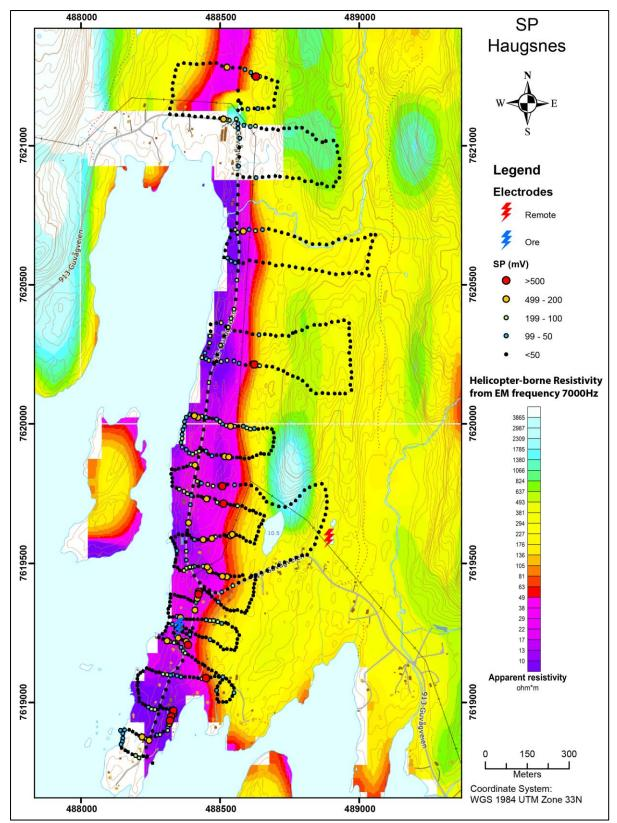
Figure 7.3: Results from SP measurements at Haugsnes overlain on top of helicopter-borne measurements of apparent resistivity from EM 7000 Hz coaxial coil configuration.
