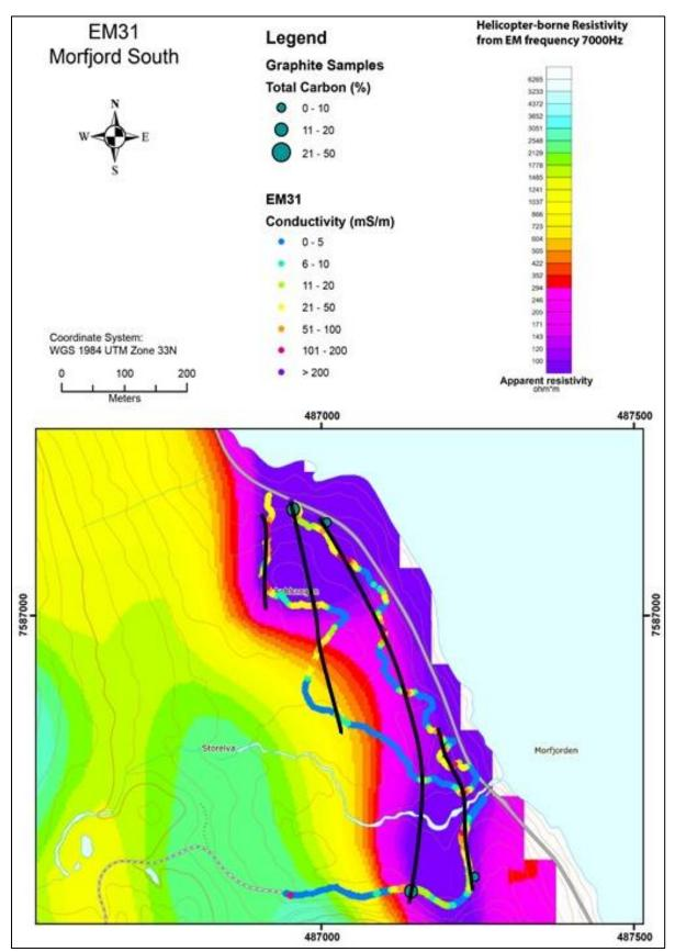
Figure 11.2: The Morfjord abandoned graphite mine. The interpreted graphite structures based on EM31 and helicopter-borne EM data are shown as black lines.
