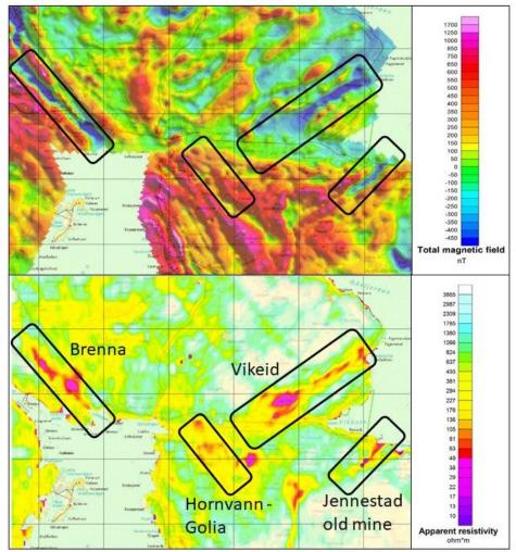
Figure 5.1: Magnetic anomaly field and apparent resistivity (7000 Hz coaxial coils) from helicopter-borne measurements in the Jennestad area, west of Sortland town (Modified from Rodionov et al. 2013a).
