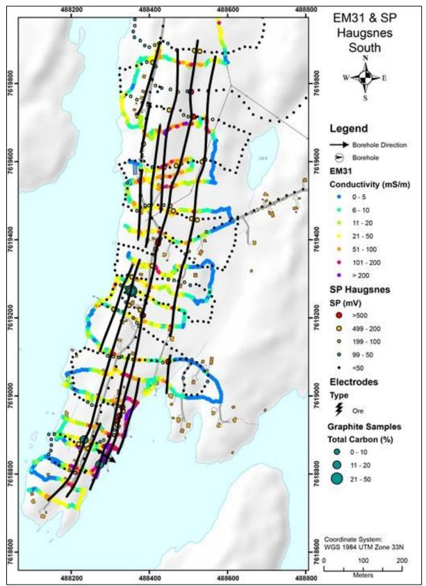
Figure 7.14: The southern part of Haugsnes. The interpreted main graphite structures based on exposed graphite, EM31 and SP data.
