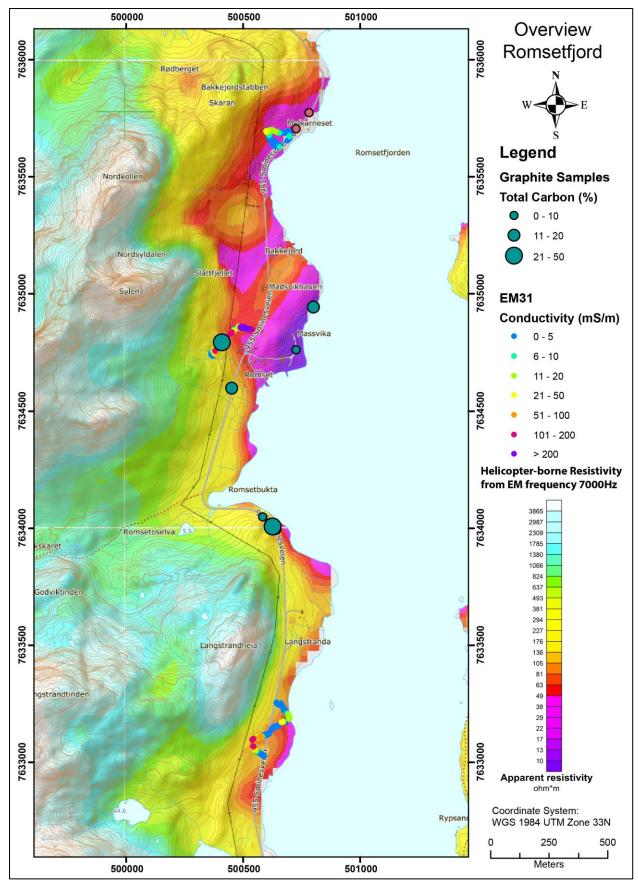
Figure 10.1: Results from EM31 measurements along Romsetfjord and graphite showings overlain on top of helicopter-borne measurements of apparent resistivity from EM 7000 Hz coaxial coil configuration.
