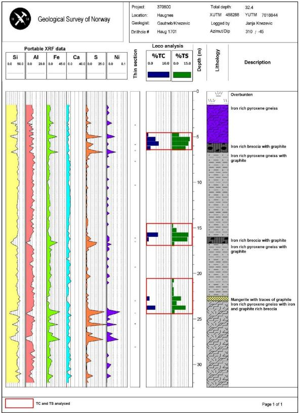
Figure 7.7: Portable XRF analyses of among others Fe-S-Ni, Leco analysis of total carbon (TC) and total sulphur (TS) together with lithological log from drill hole Haug1701.
