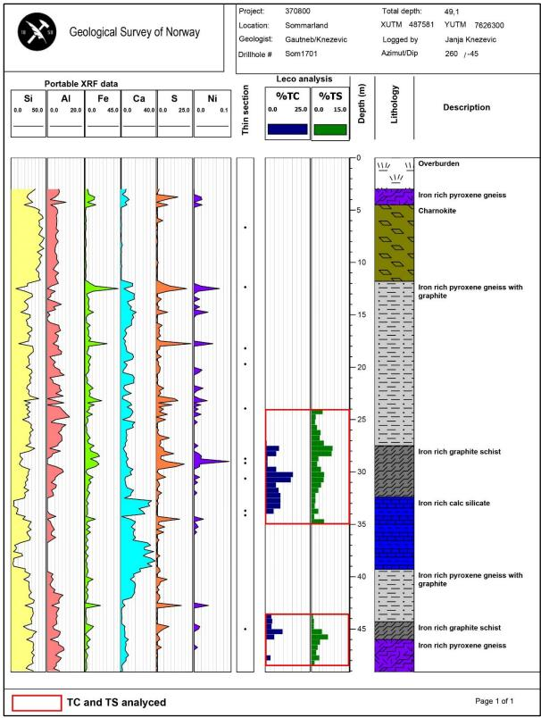
Figure 6.7: Portable XRF analyses of among others Fe-S-Ni, Leco analysis of total carbon (TC) and total sulphur (TS) in addition to the lithological log from drill hole Som1701.
