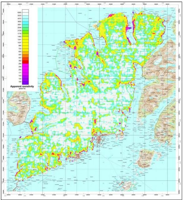
Figure 5.7: Apparent resistivity calculated from EM 7000 Hz Coaxial coil configuration at parts of Austvågøya, Lofoten.
