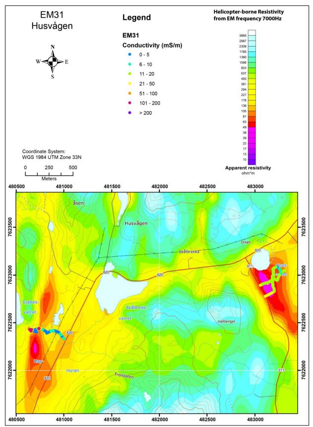
Figure 8.1: The Husvågen area is shown to the left and the Rise area is shown to the right. Results from the EM31 measurements are overlain on top of the helicopter-borne measurements of apparent resistivity from EM 7000 Hz coaxial coil configuration.
