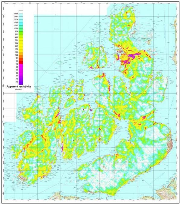
Figure 5.2: Apparent resistivity calculated from EM 7000 Hz Coaxial coil configuration at Langøya in Vesterålen.
