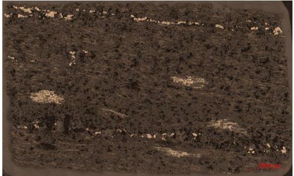
Figure 6.12: Thin section HG-DhSom1701-30.63, iron rich graphite schist in reflected light, TC 14.3 %, TS 4.88 % (30,5-31m).
