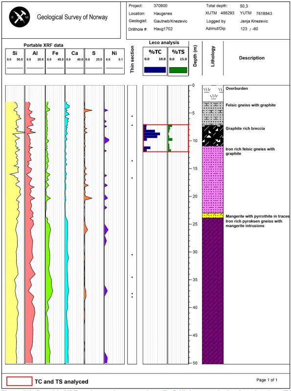
Figure 7.8: Portable XRF analyses of among others Fe-S-Ni, Leco analysis of total carbon (TC) and total sulphur (TS) together with lithological log from drill hole Haug1702.
