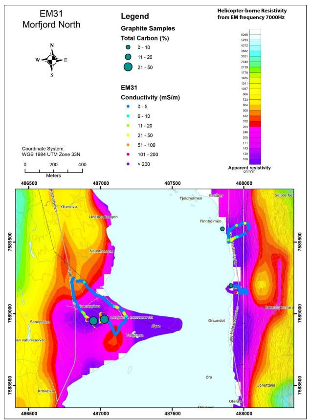
Figure 11.3: The Sommarhus and Sellåter areas. The results from the EM31 measurements and graphite showings overlain on top of helicopter-borne measurements of apparent resistivity from EM 7000 Hz coaxial coil configuration.
