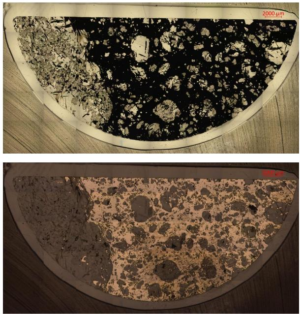
Figure 12.5: Thin section from half of a drill core, showing brecciation of the rock in areas with a high content of pyrrhotite combined with strong deformation, Transmitted light upper and reflected light lower (thin section HG-DhHau1701-6.5).
