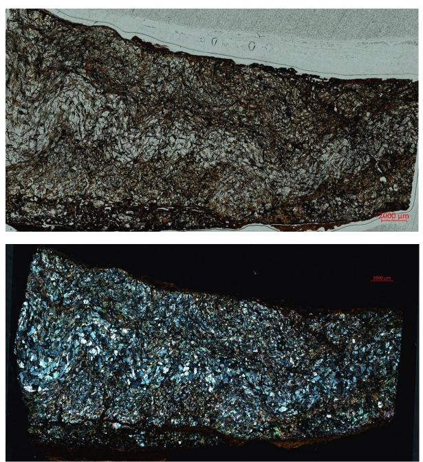
Figure 12.4: Thin section showing an example of a strongly foliated and folded graphite schist, Transmitted light upper, polarised light lower (thin section JK291517-9).
