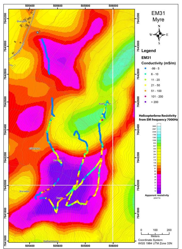
Figure 9.6: The Raudhammaren area, south-east of Myre. The results from EM31 measurements overlain on top of helicopter-borne measurements of apparent resistivity from EM 7000 Hz coaxial coil configuration.
