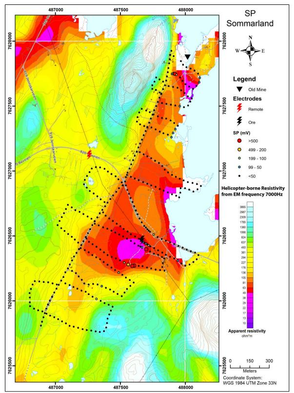
Figure 6.2: SP measurements in the central part of the Sommarland area and towards the Kråkberget abandoned mine in the north. The coloured background is apparent resistivity from helicopter-borne EM measurements with EM 7000 Hz coaxial coil configuration.
