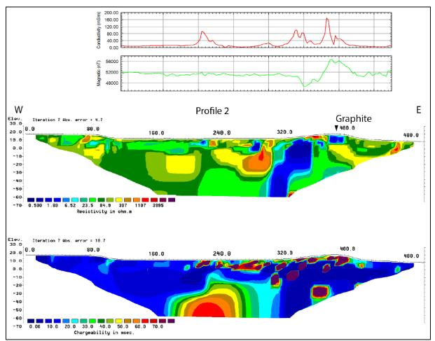
Figure 6.5: Apparent electric conductivity, magnetic total field measured with EM31, 2D Resistivity and 2D Induced Polarisation along almost the same line at Sommarland (see figure 6.4).
