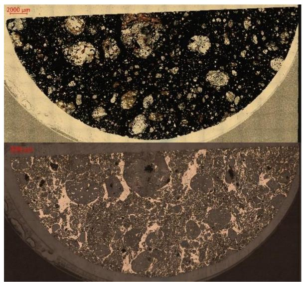
Figure 7.9: Iron rich breccia with graphite, pyrrhotite rich matrix with fragments of silicate minerals that contain graphite flakes. Thin section JK-DhHau1701-16.5 (transmitted and reflected light respectively).
