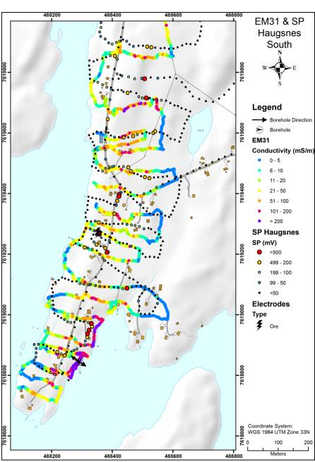
Figure 7.5: The southern part of Haugsnes. Location of core drilling and detailed results from SP and EM31 measurements.
