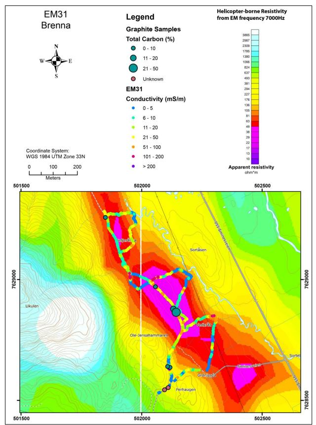
Figure 10.7: The Brenna area. The results from the EM31 measurements and graphite showings overlain on top of helicopter-borne measurements of apparent resistivity from EM 7000 Hz coaxial coil configuration.
