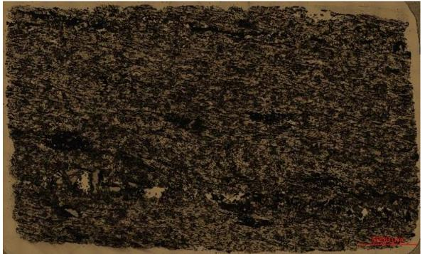
Figure 6.11: Iron rich graphite schist (transmitted light) TC 14,3%, TS 4,88% (30,5-31m). Thin section HG-DhSom1701-30.63.
