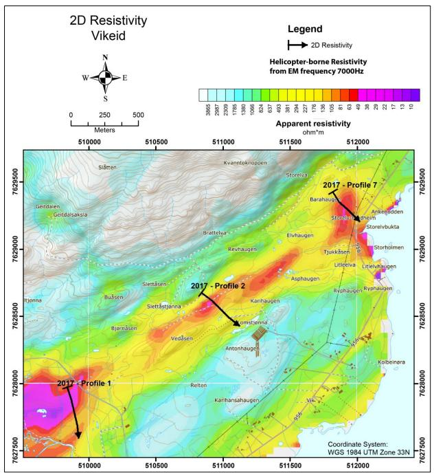
Figure 10.3: The Vikeid area. The location of the 2D Resistivity/IP profiles overlain on top of helicopter-borne measurements of apparent resistivity from EM 7000 Hz coaxial coil configuration.
