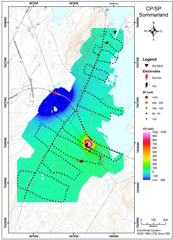
Figure 6.3: CP measurements with grounding point in the central part of the Sommarland area and SP data from the same area.
