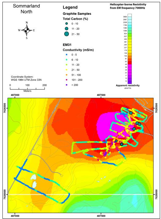
Figure 6.1: The central part of the Sommarland area. The results from EM31 measurements overlain on top of helicopter-borne measurements of apparent resistivity from EM 7000 Hz coaxial coil configuration.
