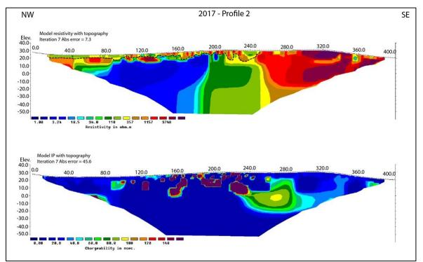
Figure 10.5: The Vikeid area. The results of the 2D Resistivity and Induced Polarisation measurements along profile 2017-2. The interpreted soil-bedrock interface as dotted black line.
