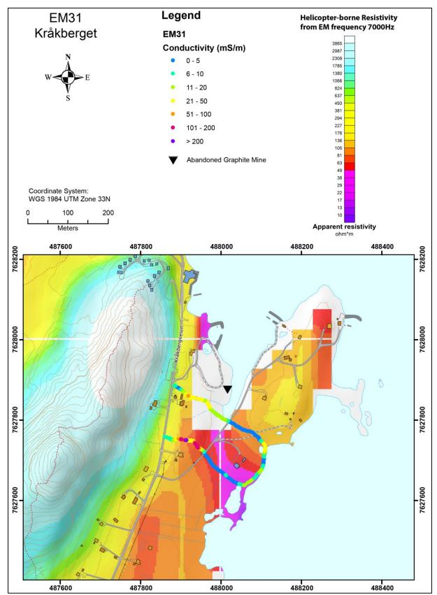
Figure 6.16: Kråkberget north of Sommarland. Results from EM31 measurements overlain on top of helicopter-borne measurements of apparent resistivity from EM 7000 Hz coaxial coil configuration.
