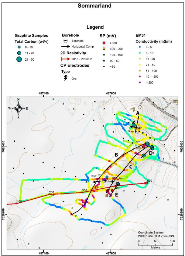
Figure 6.19: Central Sommarland. Interpreted main graphite structures based on EM31, SP and CP data.
