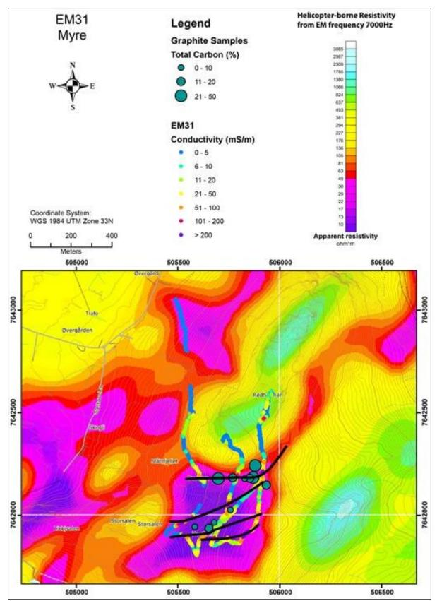
Figure 9.7: The Raudhammaren area, south-east of Myre. The results from EM31 measurements, the location of graphite bearing loose boulders and an interpretation of potential graphite structures overlain on top of helicopter-borne measurements of apparent resistivity from EM 7000 Hz coaxial coil configuration.
