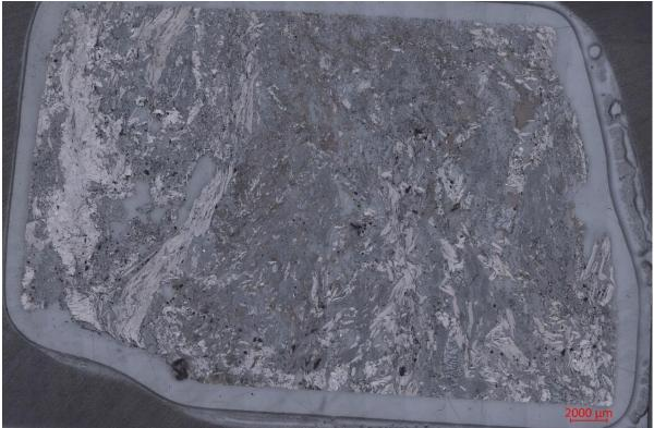
Figure 12.2: The graphite seen in reflected light showing large variations in the distribution and grain size of graphite flakes (thin section JK-2617-2-Sommarhus- 24,7%TC).
