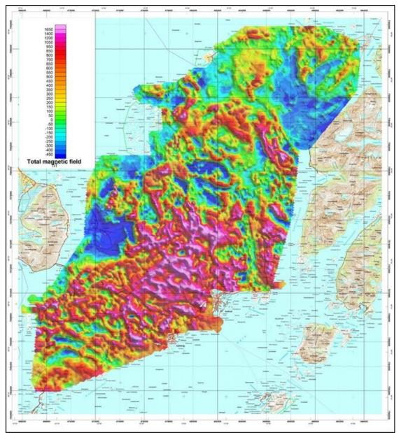
Figure 5.8: Magnetic anomaly field at parts of Austvågøya, Lofoten.
