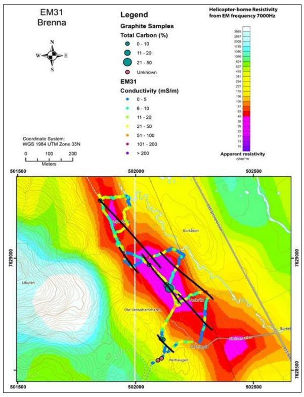
Figure 10.11: The Brenna area. The interpreted graphite structures based on EM31 and helicopter-borne EM data are shown as black lines.
