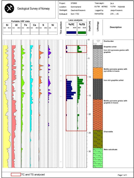
Figure 6.8: Portable XRF analyses of, among others Fe-S-Ni, Leco analysis of total carbon (TC) and total sulphur (TS) together with the lithological log from bore hole Som1702.
