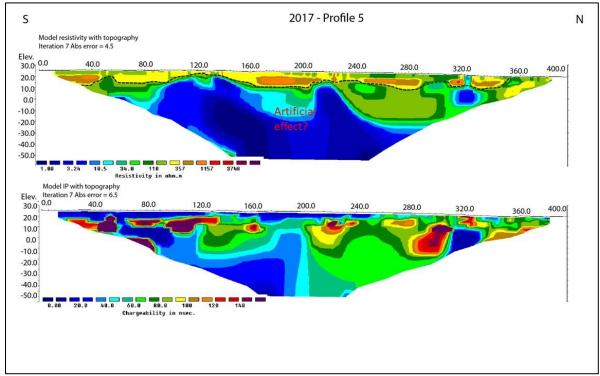
Figure 9.5: The area east of Myre. The results from 2D Resistivity and Induced Polarisation measurements along profile 2017-5. The interpreted soil-bedrock interface is shown as a dotted black line.
