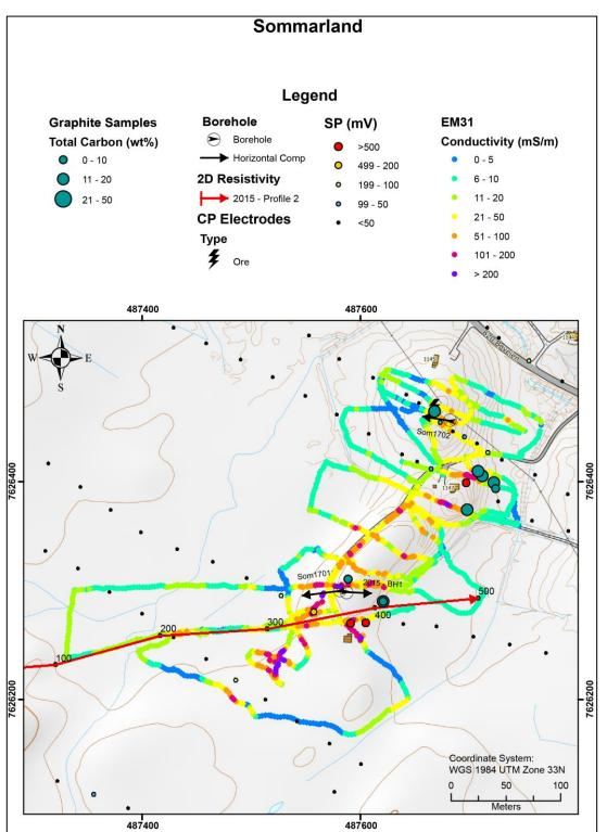
Figure 6.4: Location of the bore-holes in Sommarland (2015 Bh 1, Som1701 and Som1702), 2D Resistivity/IP profile from 2015 and graphite showings overlain on top of EM31 and SP anomalies.
