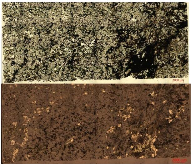
Figure 6.13: Thin section JK-DhSom1701-19.7, host rock that contain graphite in veins and disseminated thin long graphite flakes and abundant iron sulphides.
