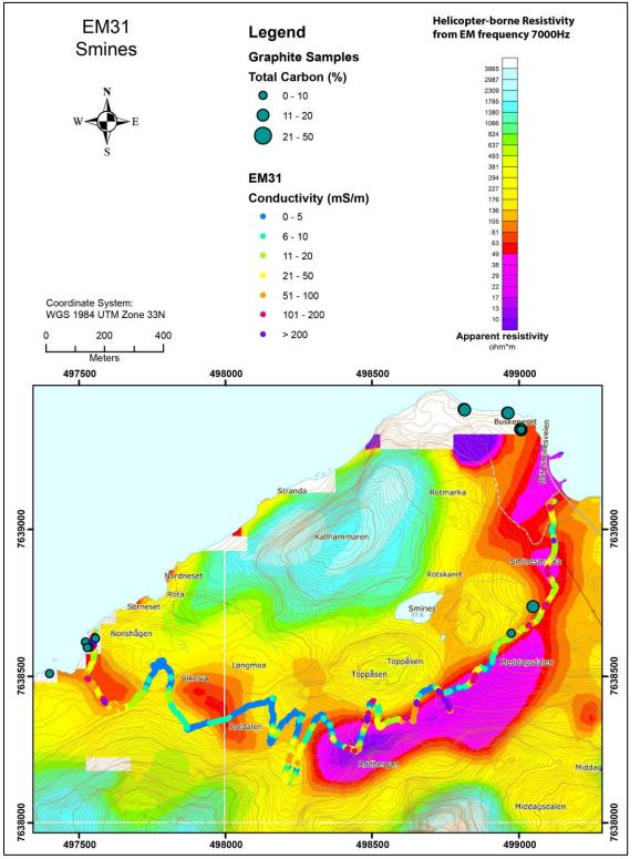
Figure 9.1: Results of EM31 measurements from the Smines area overlain on top of helicopterborne measurements of apparent resistivity from EM 7000 Hz coaxial coil configuration.
