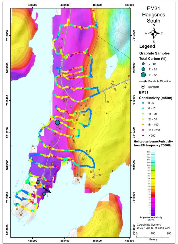
Figure 7.2: The southern part of Haugsnes. Results from EM31 measurements overlain on top of helicopter-borne measurements of apparent resistivity from EM 7000 Hz coaxial coil configuration.
