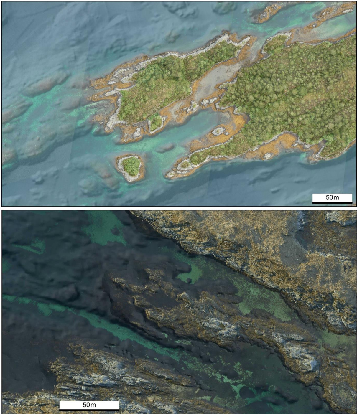
Figure 6. Examples of transparency applied to GLaSS aerial photographs overlain on GLaSS LiDAR and multibeam shaded relief allowing bottom types visible in the photographs to be related to topographic variations. This makes it easier to delimit areas with similar properties.
