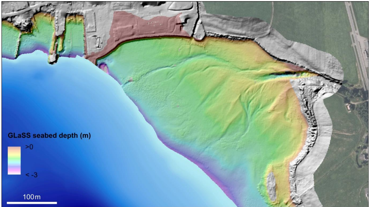
Figure 2. GLaSS LiDAR bathymetry (colour shaded relief) and multibeam bathymetry (blue-scale) showing 100% coverage and overlap between the 2 datasets. The multibeam data are shown on the top of the LiDAR data. Background data: orthophotos from www.norgeibilder.no
