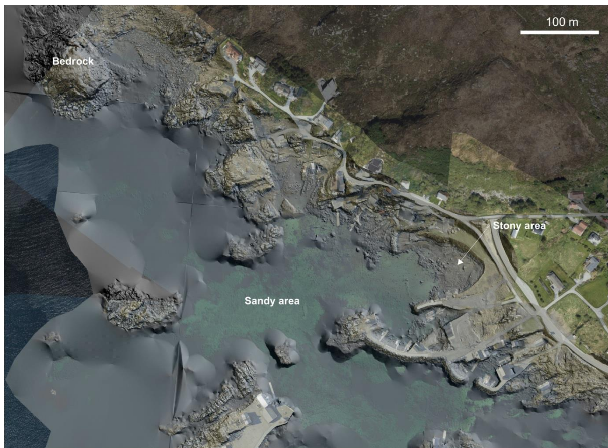
Figure 16. Example of GLaSS bathymetry data, overlain by photomosaics with 60% transparency. Note the different properties of the three main classes (i) sandy areas (here likely gravelly sand, clearly visible in the photomosaics with light color patches) occurring as flat seabed (ii) stony areas (here sand, gravel, cobbles and boulders) show moderate rugosity with variations in relief representing boulders (iii) bedrock areas have a high rugosity. Background data: Orthophotos from www.norgebilder.no .
