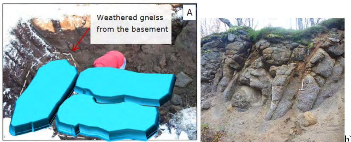
Figure 11.20. a) Photo by Rambøll with reconstruction of how the angular blocks were lying in the pit before they were moved by the excavator. b) An example from Eiavatnet in Nordland for such angular blocks. The angular blocks are a common appearance in the deepest part of a weathering profile, close to the front with unweathered basement, commonly referred to as sapro-rock.
