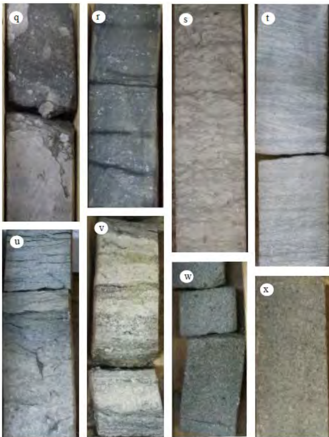
Figure 10.14. cont. Photos of cores from Well B. q) Fine-grained sandstone overlain by intraformational conglomerate with sandstone intra-clasts (depth 503.8 m). r) Very fine- to fine-grained sandstones containing siltstone laminae (depth 501.7 m). s) Syn-sedimentary deformed sandstones with thin laminae of siltstones (depth 485.3 m). t) Cross-laminated sandstones (depth 481.8 m). u) Flat-laminated sandstone laminae. w) Green massive fine- to medium-grained sandstone (depth 459.9 m). x) Grey massive fine- to medium-grained sandstone (depth 457.8 m).
