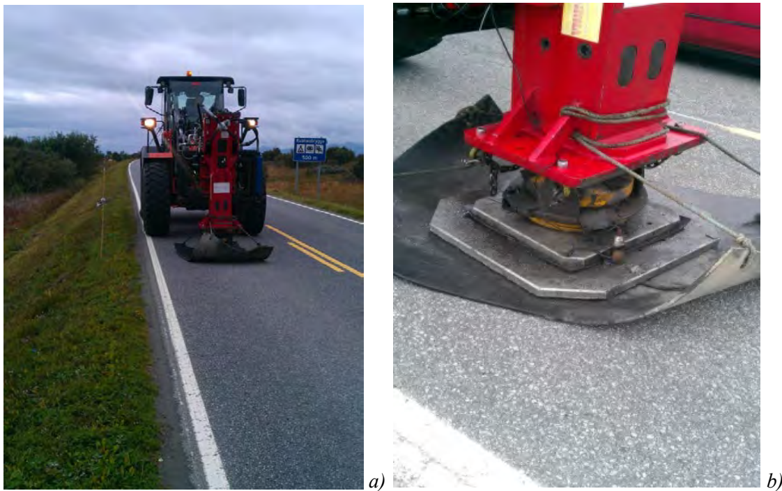
Figure 5.3. Picture of truck carrying the Vibrist-3000 seismic source, including a close-up of the hydraulic hammer and steel plate (b).
