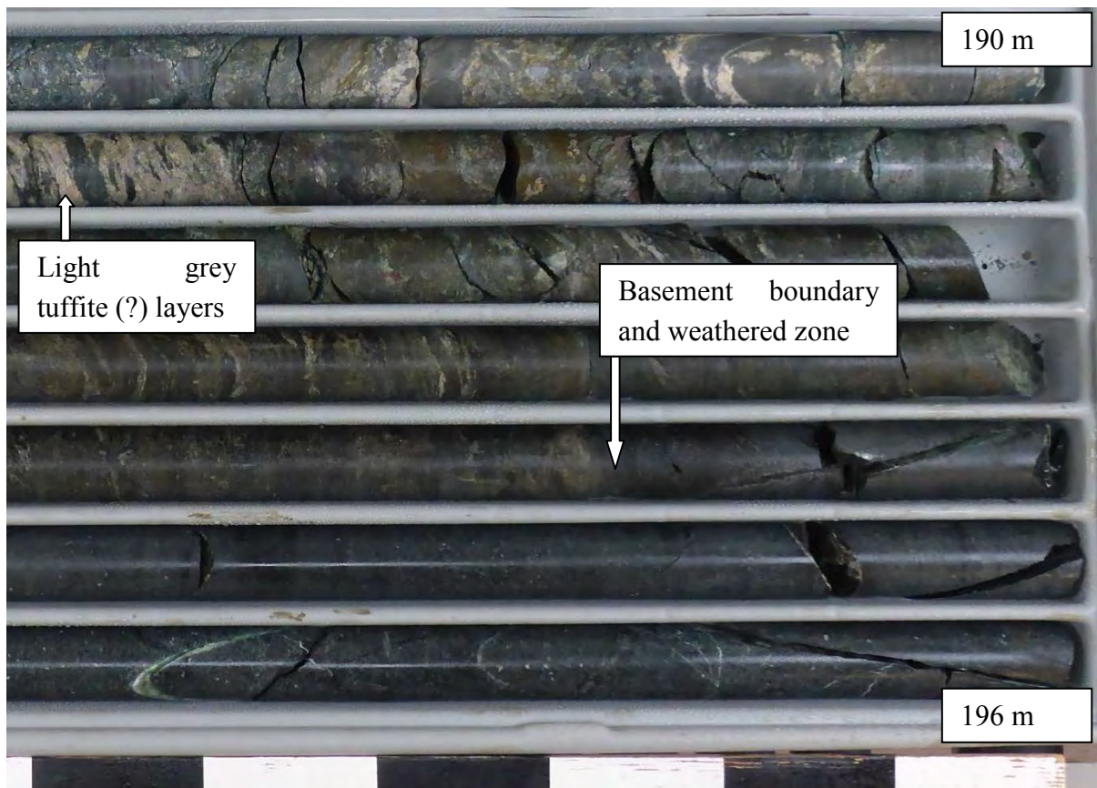
Figure A3-12B: NGU BH 1: Cores from 189-196 m depth in NGU BH 1. A magnified view of the right hand side of the previous picture (Fig. A2-12A), showing lithologies and textures of the sediments. Also the basement boundary with its weathered zone (in granodiorite) is marked.
