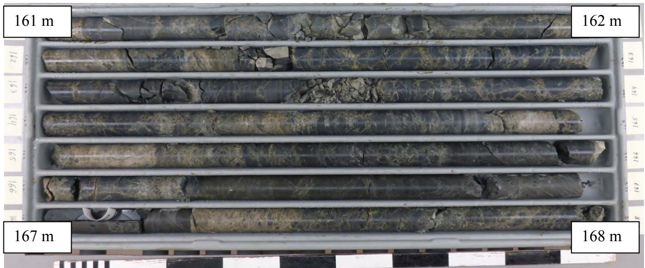
Figure A3-8: NGU BH 1; cores from 161-168 m depth. Sample 167.0 is from this core box (white label). These sediments are characterized as sedimentary breccia or debris flow, partly with large clasts of altered mafic rocks. Fragments of fine-grained light grey sandstone are also seen, partly as layers and in the matrix, together with talc and chlorite. The mineralogy of this fine sandstone (Sample 167.0 m) indicates that it is actually an altered tuffite; the dominating minerals being plagioclase, smectitic clay minerals, biotite and hematite. Furthermore, this is the only sample between 129.8 m and 193.75 m depth that is without talc, which further indicates an origin different from the debris flows/sedimentary breccias.
