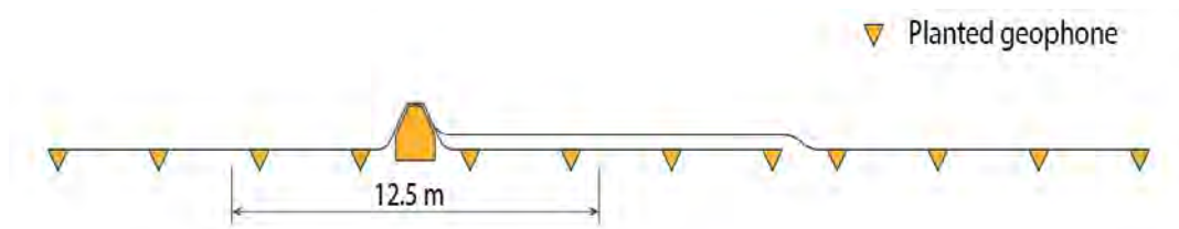
Figure 5.2. Schematics of recording set up during autumn (planted geophones) and during winter (gimballed geophones).
