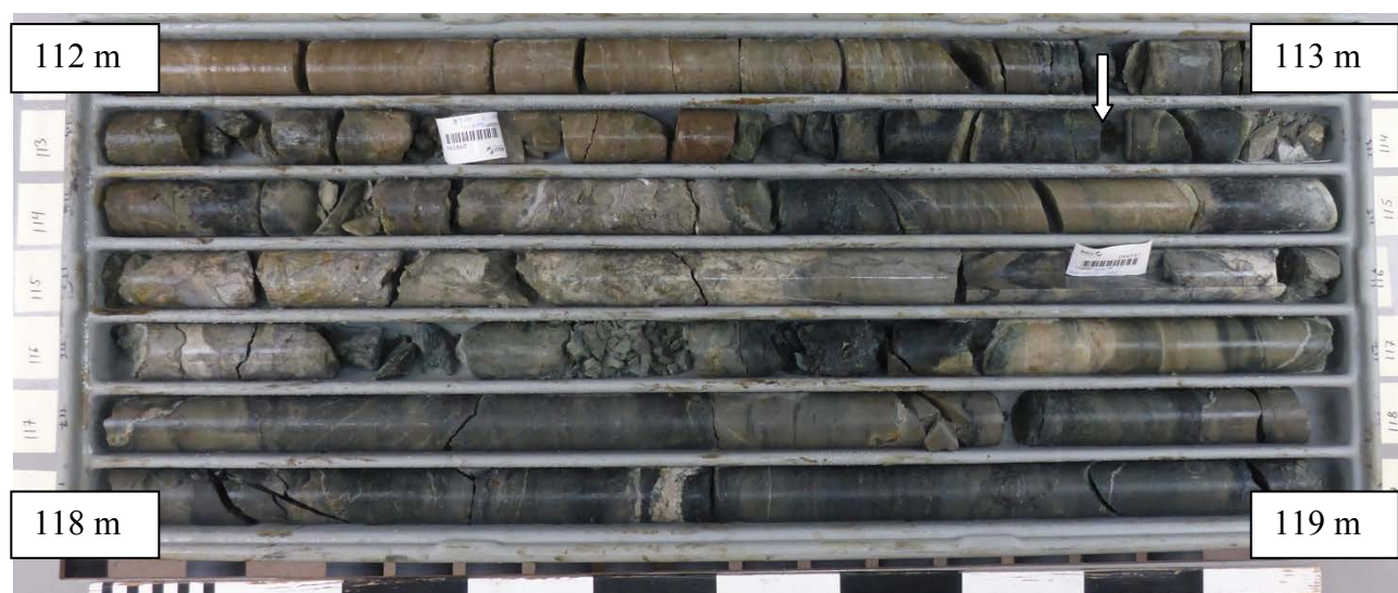
Figure A3-1. NGU BH 1; cores from 112-119 m depth. Three samples are selected from this core box: 113.4 m (marked with white label), 113.9 m (marked with arrow), and 115.6 m (marked with white label). From 112 to 114 m: Motley, fine clastic sediment, consisting of mainly feldspars, quartz and kaolinite (Table 7.1). Sample 115.6 represent an altered conglomeratic rock consisting of actinolite, calcite and quartz. The rocks further down to 129.8 are sediments derived mainly from mafic rocks (dark grains), but also some quartz-feldspatic layers. Possibly also some thin layers of chert and clay (smectitic clay?). The top and bottom of the first and last core in the box are marked with correct depth. (The scale bar is divided into dm and cm).
