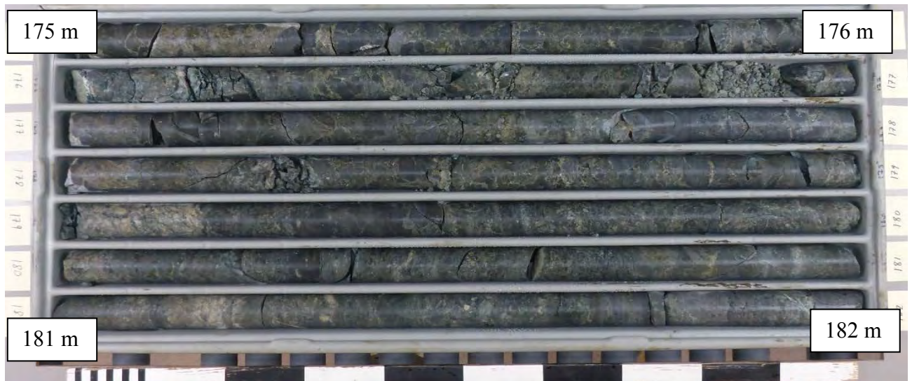
Figure A3-10: Cores from 175-182 m depth in NGU BH 1. The sediments in this interval are described as polymict conglomerates of dark angular mafic rock clasts with abundant (lighter) matrix; probably debris flows. Some interlayering with thin layers of fine-grained light grey sandstone.
