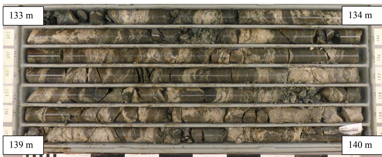
Figure A3-4. NGU BH 1; cores from 133-140 m depth. Sediment derived mainly from mafic rocks, also with quartz-feldspatic layers and lenticular lenses. Some conglomeratic layers with angular rock clasts; maybe debris flow? Sample 134.7 m is from this core box. XRD data for this sample shows mainly talc, biotite, illite, plagioclase, and some chlorite (Table 7.1).
