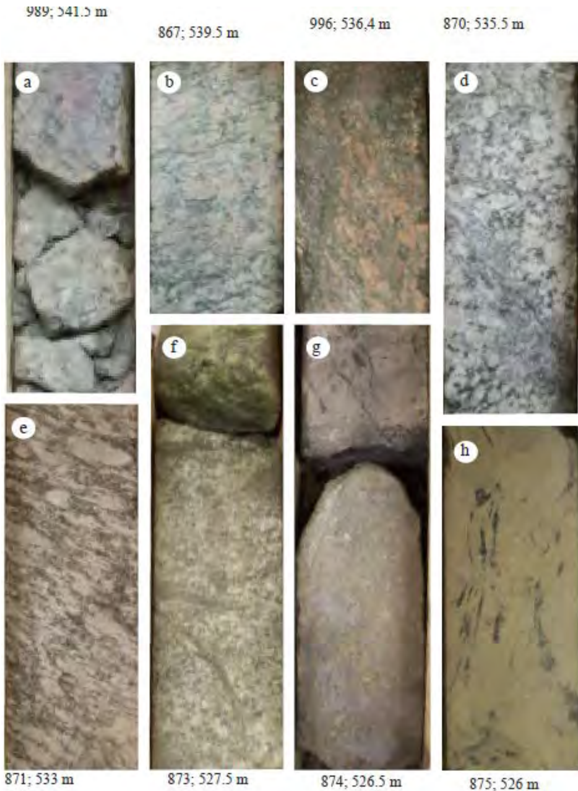
Figure 10.14. Photos of cores from Well B: a) fractured granodiorite, enriched in clay along fractures (depth: 541.5 m). b) Granodiorite with phaneritic texture (depth: 539.5 m). c) Greenish granodiorite, with some chlorite and feldspars (depth: 536.4 m). d) Granodiorite with phaneritic texture and diagonal seam poor in feldspars (depth: 535.5 m). e) Granodiorite with deformed feldspars (depth: 533 m). f) Green rock with a texture of fine-grained sandstone (depth: 527.5 m). g) Conglomerate overlain by claystone, containing rootlets and organic matter. The conglomerate contains sub-rounded quartz clasts floating in a sandy matrix (depth: 526,5 m). h) Claystone with rootlets (depth: 526 m).
