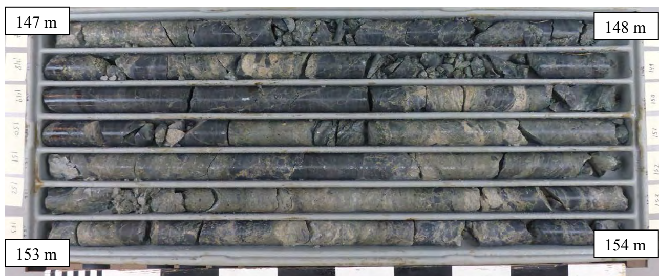
Figure A3-6. NGU BH 1; cores from 147-154 m depth. Similar lithologies as the previous core interval. Several conglomeratic layers, with angular to sub-rounded clasts; commonly in a light grey matrix.
