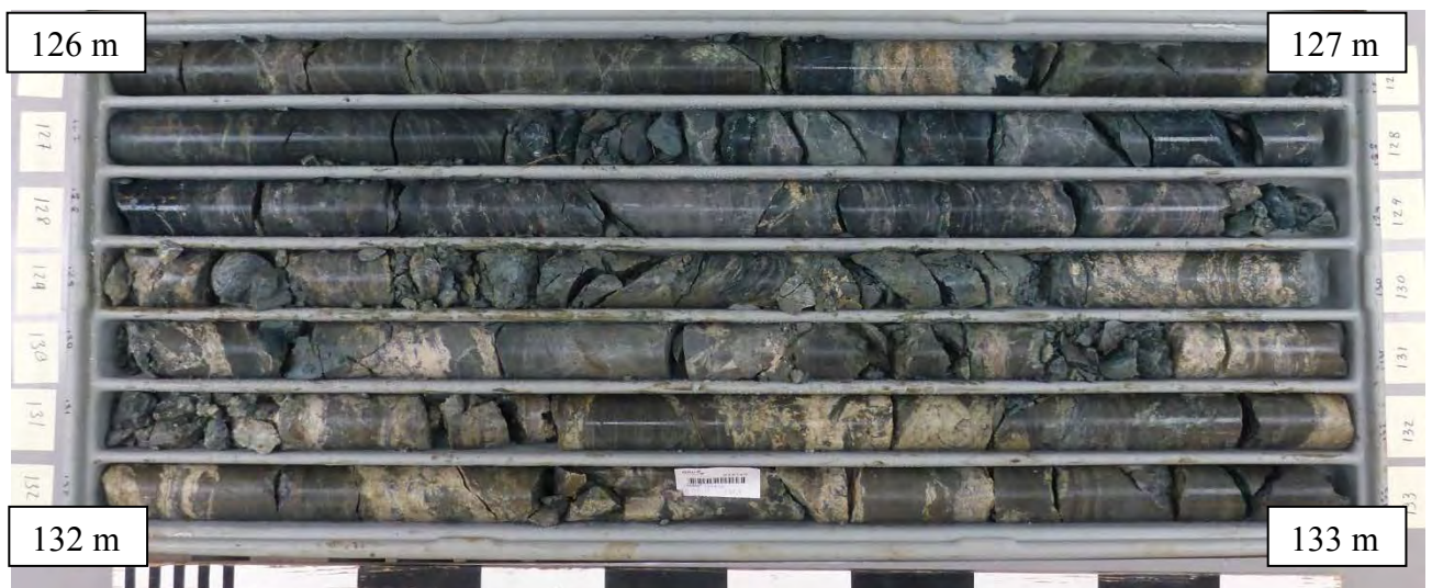
Figure A3-3: NGU BH 1; cores from 126-133 m depth. Sample from 132.4 m is marked with white label. The cores represent mainly mafic derived sand (dark grains), but also some quartz-feldspatic layers. Lenticular lenses and also some thin layers of possibly chert and clay (smectitic clay?). Sample 132.4 m consists mainly of talc, biotite, illite, plagioclase, and some chlorite (Table 7.1). The cores from 130-132 m show conglomeratic intervals, with angular rock clasts: may be debris flows?
