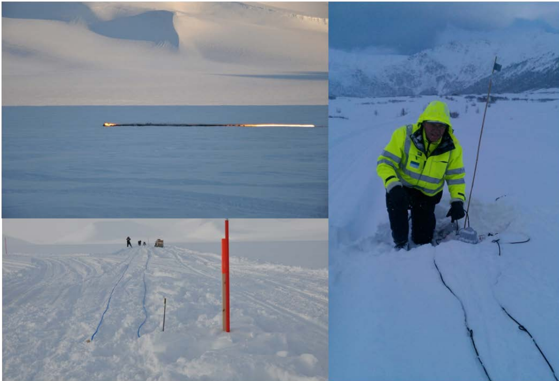
Figure 5.6. Seismic acquisition during wintertime. a) Detonating cord laid out. b) A shot fired, and c) Geophone strings were partly buried in snow, sheltering them from weather noise.
