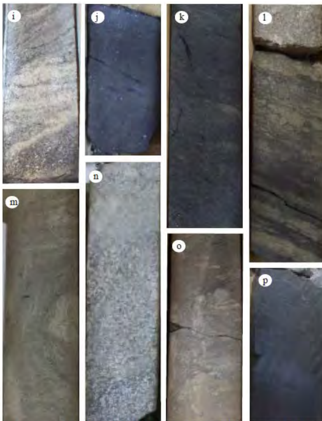
Figure 10.14 cont. Photos of cores from well B. i) Medium-grained sandstone, syn-sedimentary deformed (depth 523 m). j) Coal layer (521.5 m). k) Siltstone with pyrite lenses and rootlets (519.5 m). l) Siltstones interbedded with slumped, fine-grained sandstones (504.8 m). m) Slumped siltstones interbedded with fine sand. n) Quartz sandstones, varying from very coarse to medium-grained (518.2 m). o) Slumped very fine sandstones interbedded with siltstones (517.7 m). p) Coal layer (491.5 m).
