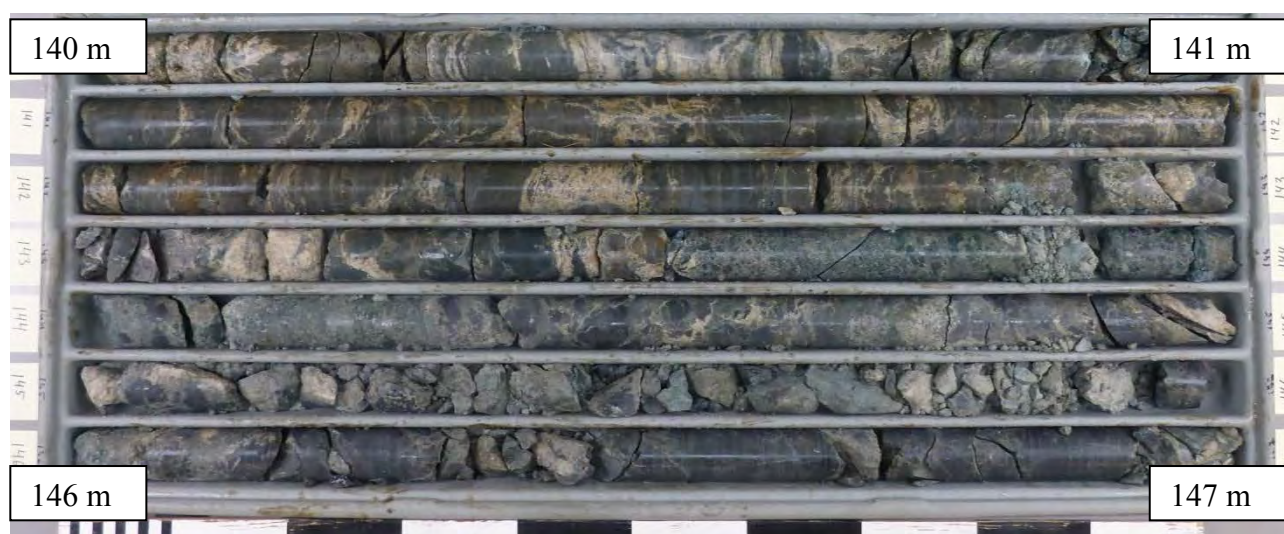
Figure A3-5. NGU BH 1; cores from 140- 147 m depth. 129.78-143.20 m: Some conglomeratic layers with angular-to-rounded rock clasts; maybe debris flow? Similar composition as the previous core interval.
