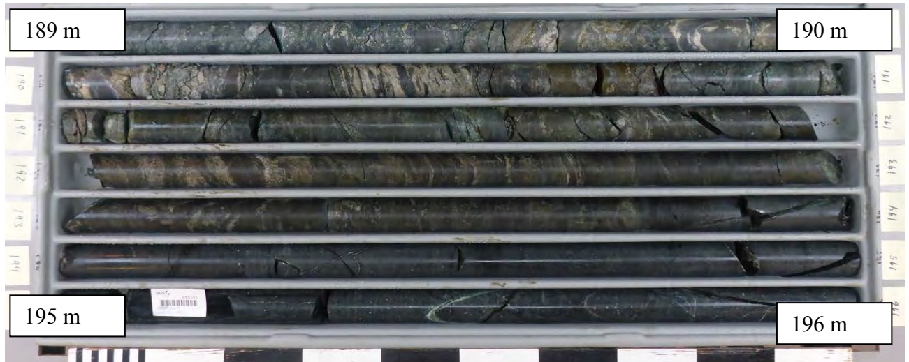
Figure A3-12A: Cores from 189-196 m depth in NGU BH 1. Sample 195.1m is from this core box (white label). The sediments from 189 to 190.55 m are described as a polymict conglomerate with abundant matrix, interlayered with thin layers of fine-grained light grey sandstone, while the interval from 190.55 m to 193.75 m are described as a sedimentary breccia or debris flow, partly with lenticular lenses and large clasts of talc-rich altered mafic rocks. The dominating minerals in Sample 195.1 m are plagioclase and hornblende; i.e. an amphibolite intrusion (Table 7.1). The boundary to the granodioritic basement is at 193.75 m, and a c. 5 cm thick fossil weathering zone seem to have developed in the upper rim of the granodiorite.
