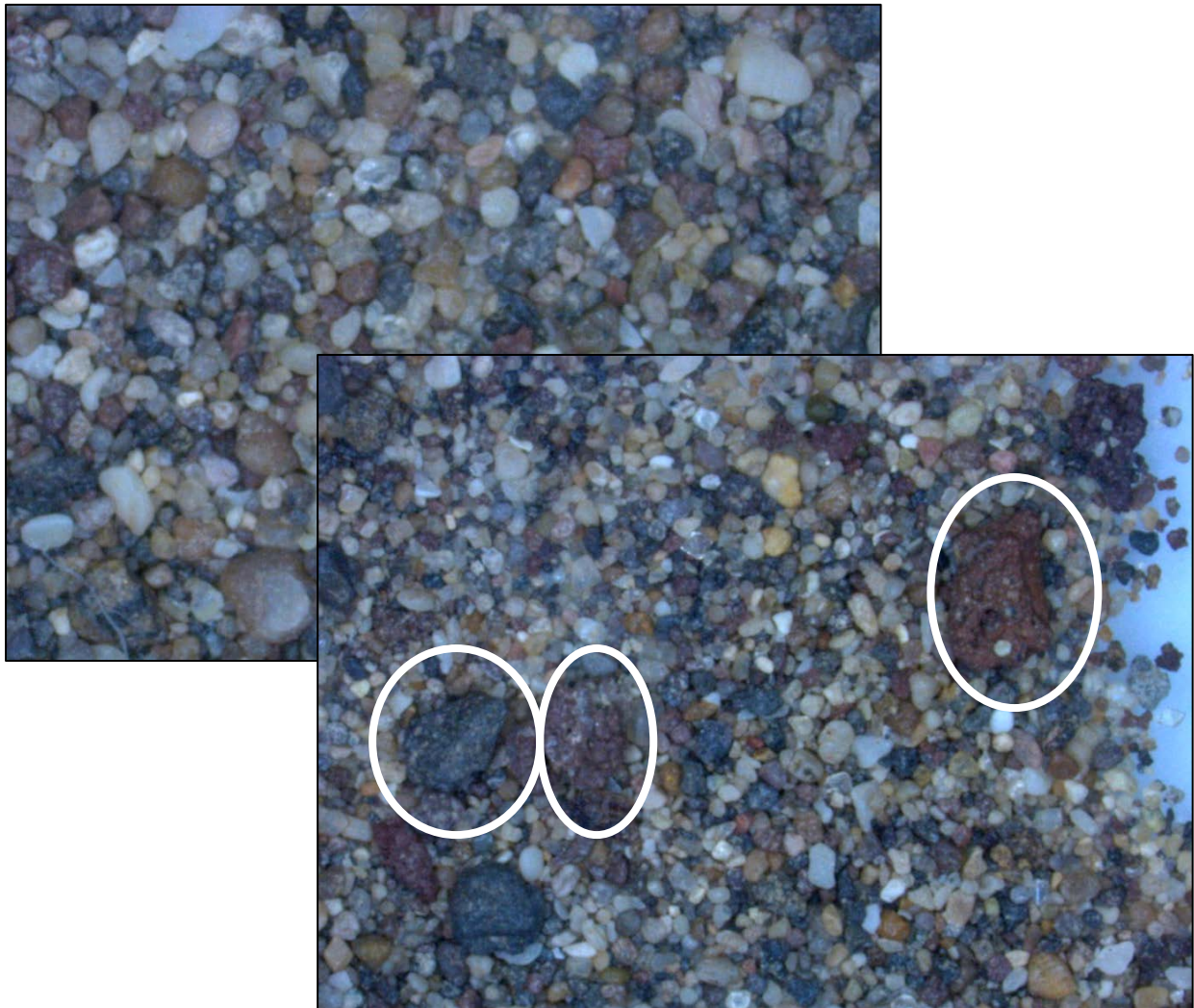
Figure 2. Microphotos of the fine fraction in the submitted sample. The fine fraction consists predominantly of rounded mineral grains of a fairly restricted size variation; 0.1-0.3 mm (no scale bar). The larger grains are all ash particles of volcanic origin; some of these grains are marked by circles.
