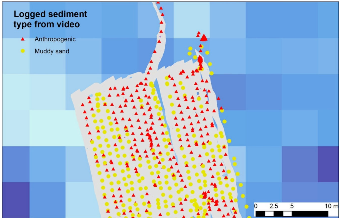
Figure 28. 1:250 view of 5 m multibeam resolution (blue pixels) and geo-logged shapefile showing bottom type overlain on UHI classification. Note that geo positions are 1.5 m ahead of the centre position of the ROV, estimating the field of view of the video camera. The UHI data are directly below the ROV.
