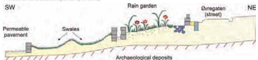
Section of the sustainable water management "treatment train", with rainwater garden, swales and permeable pavement. Drawing: Johannes de Beer, Geological Survey of Norway.
