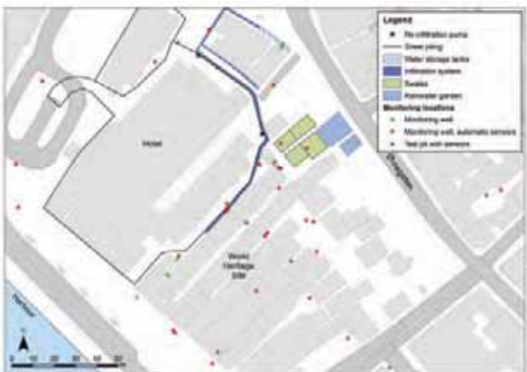
Overview map of mitigation measures carried out by the Groundwater Project, including locations of monitoring wells for measurement of groundwater level, temperature and sampling. Mitigation measures consist of a "treatment train" made up by rainwater gardens, green swales, permeable pavement and a subsurface infiltration/transport system with storage facility and re-infiltration of groundwater. Map: Anna Seither, Geological Survey of Norway.
