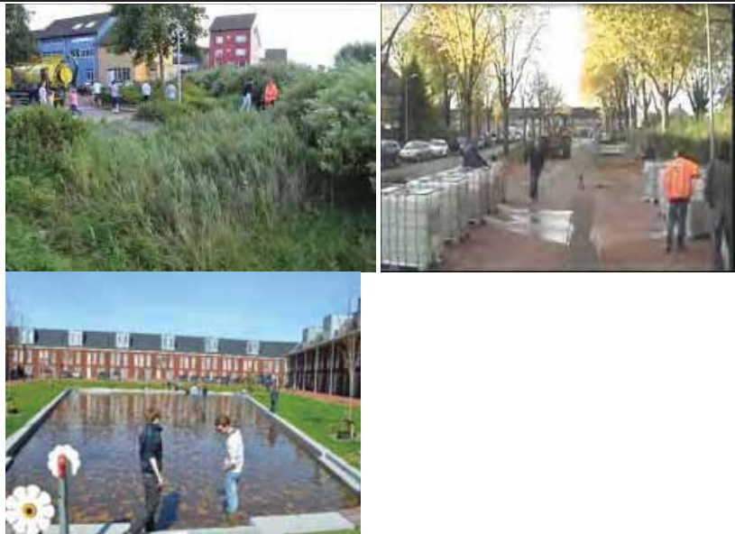
Full scale test at swale (left), full scale test at permeable pavement (right), Full scale test at watersquare (right).
