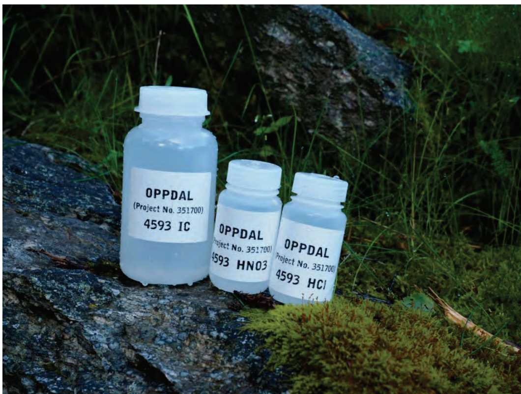
Figure 4: The three bottles filled at each sample site providing information on site number and sample treatment.
