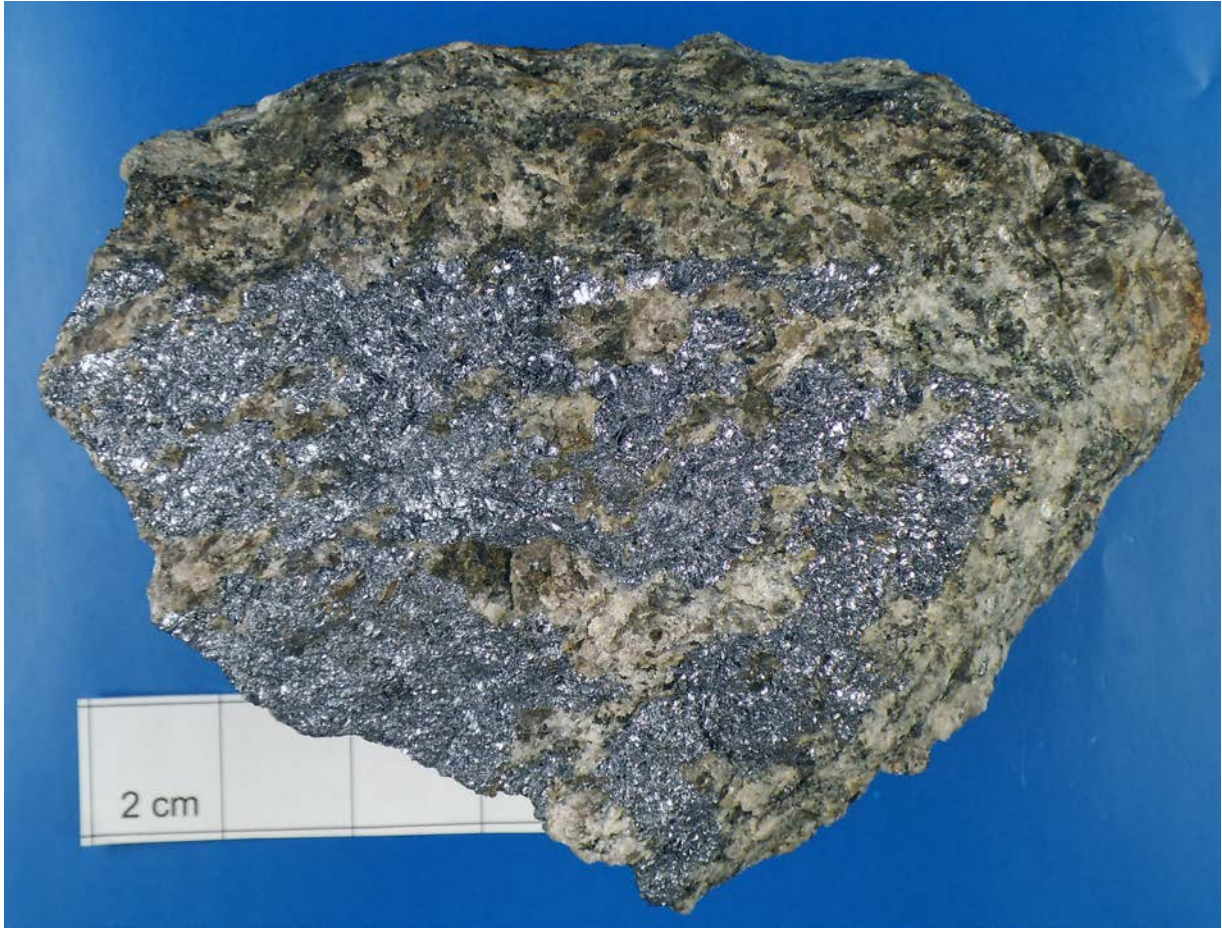
Figure 23. Hand specimen of grey, quartz-rich granite with coarse-grained molybdenite fracture filling. Knaben 2 mine, sample 24091101. The edges of the squares on the scale corresponds to 2 cm.
