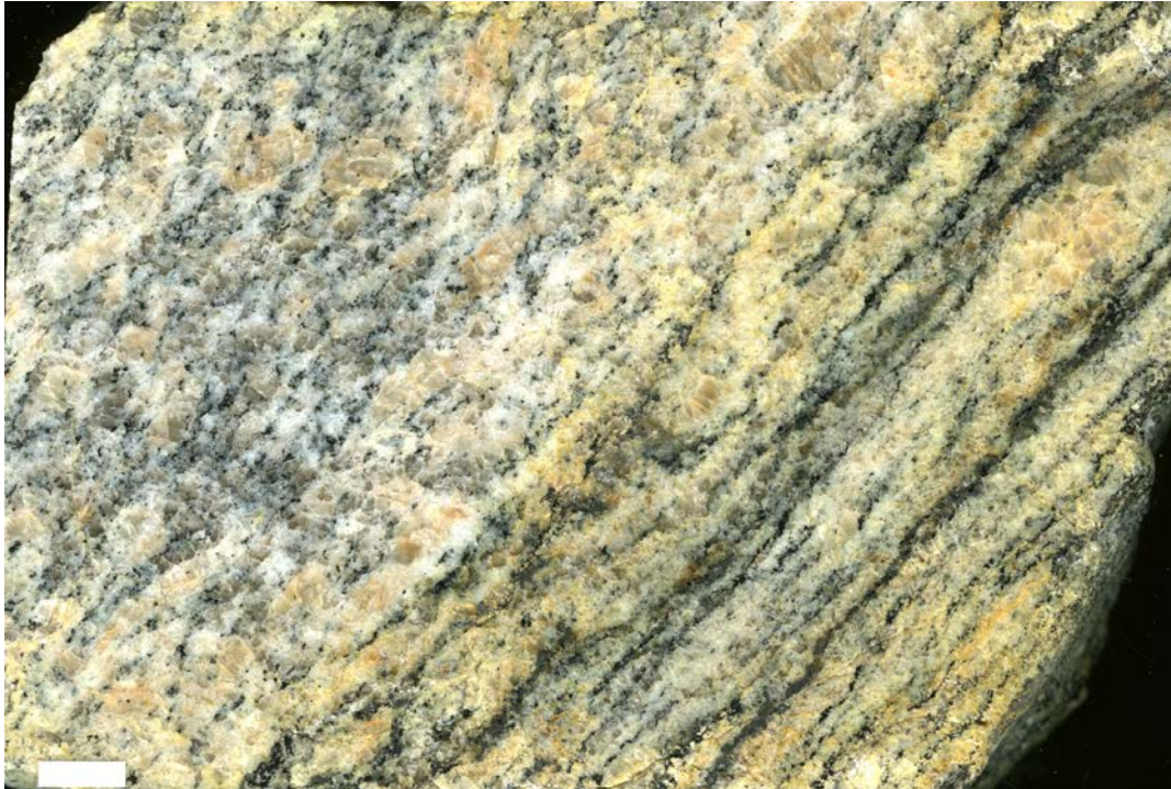
Figure 3. Hand specimen showing the contact between porphyritic reddish biotite granite (left) and flaser gneiss (right) from the Roma mine, upper north tunnel (sample 26091304). The scale corresponds to 1 cm.
