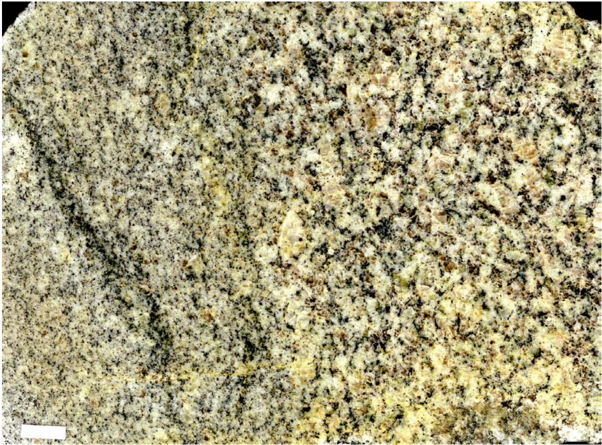
Figure 18. Hand specimen showing the diffuse contact between non-mineralized, fine-grained and medium-grained, weakly porphyritic reddish biotite granite. Ørnehommen lower tunnel, sample 25091301. The scale corresponds to 1 cm.
