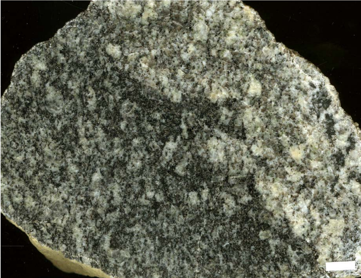
Figure 13. Hand specimen showing the diffuse contact between reddish porphyritic granite (upper right) and biotite-rich granite of presumably granodioritic composition (sample 26091306). The scale corresponds to 1 cm.
