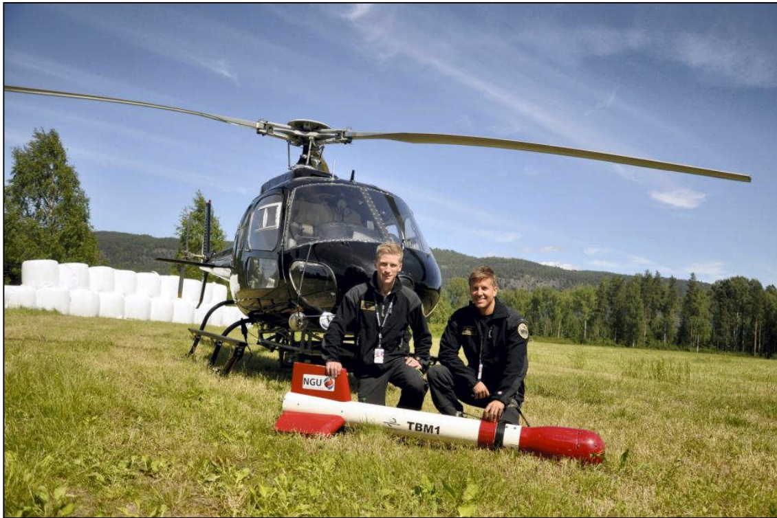
Figure 2: Photo of Heliscan's Eurocopter AS350-B2 (P1). The Mag bird in front of the helicopter and the spectrometer under its belly are also depicted.
