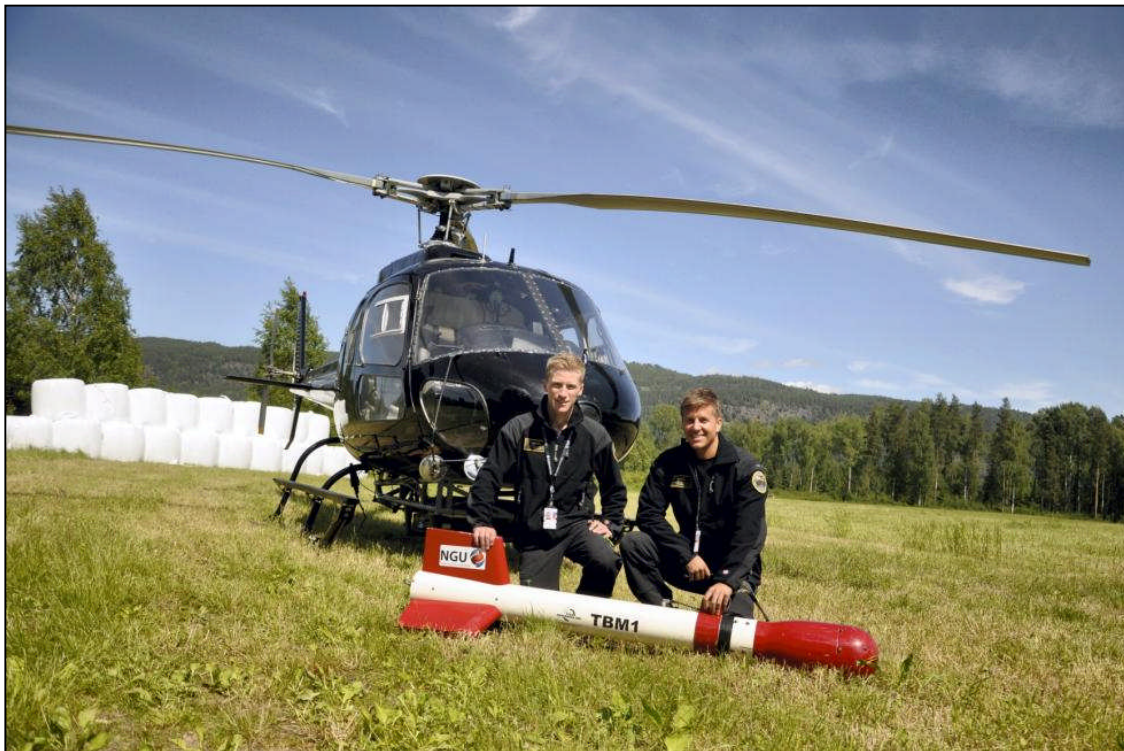
Figure 2: Pilots with Mag bird in front of the helicopter used in survey. (P1)
