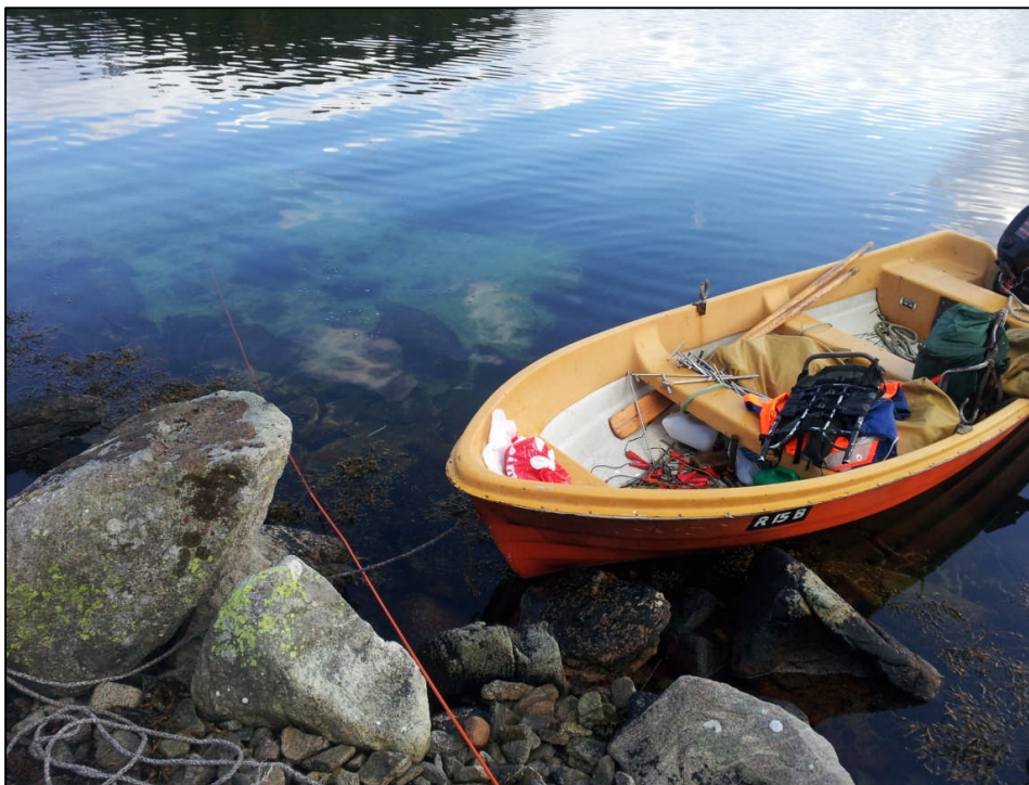
Figure 7: Sea-bottom electrode mode with the cable sinking to the sea bottom on its own weight.
