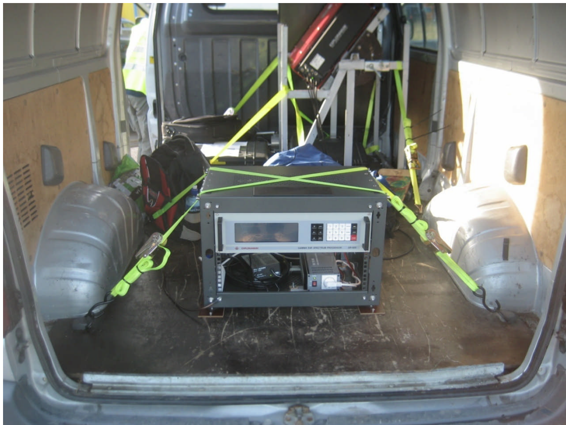
Figure 2: The GR-820 detector (red and black object in background) and spectrometer (foreground) mounted in the NGU van.
