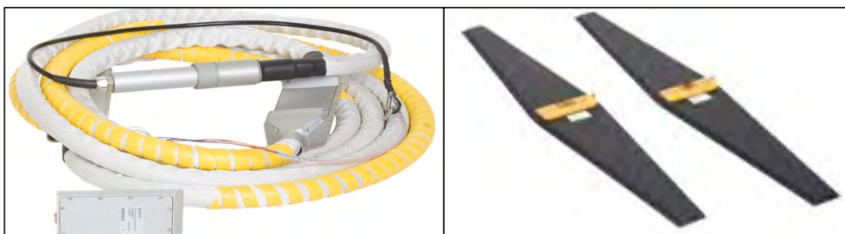
Figure 3: The RTA "snake" antenna (left) and standard unshielded 100 MHz antennas by Malå (right), ( www.malags.com ).
