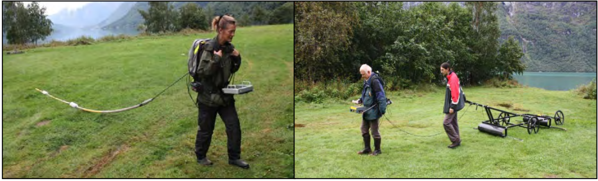
Figure 7: GPR profiling at Bøaøyna with the use of Georadars from Malå RTA (left) and Sensors & Software (right). Lovatnet lake is located in the background.
