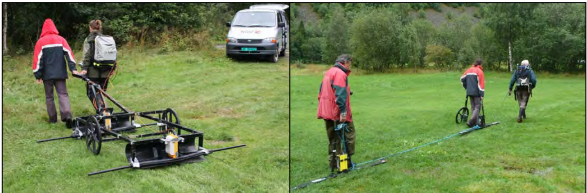
Figure 8: Malå 50 MHz Unshielded antennas on Sensors & Software cart (left) and S&S EKKO Pro in endfire mode (right).
