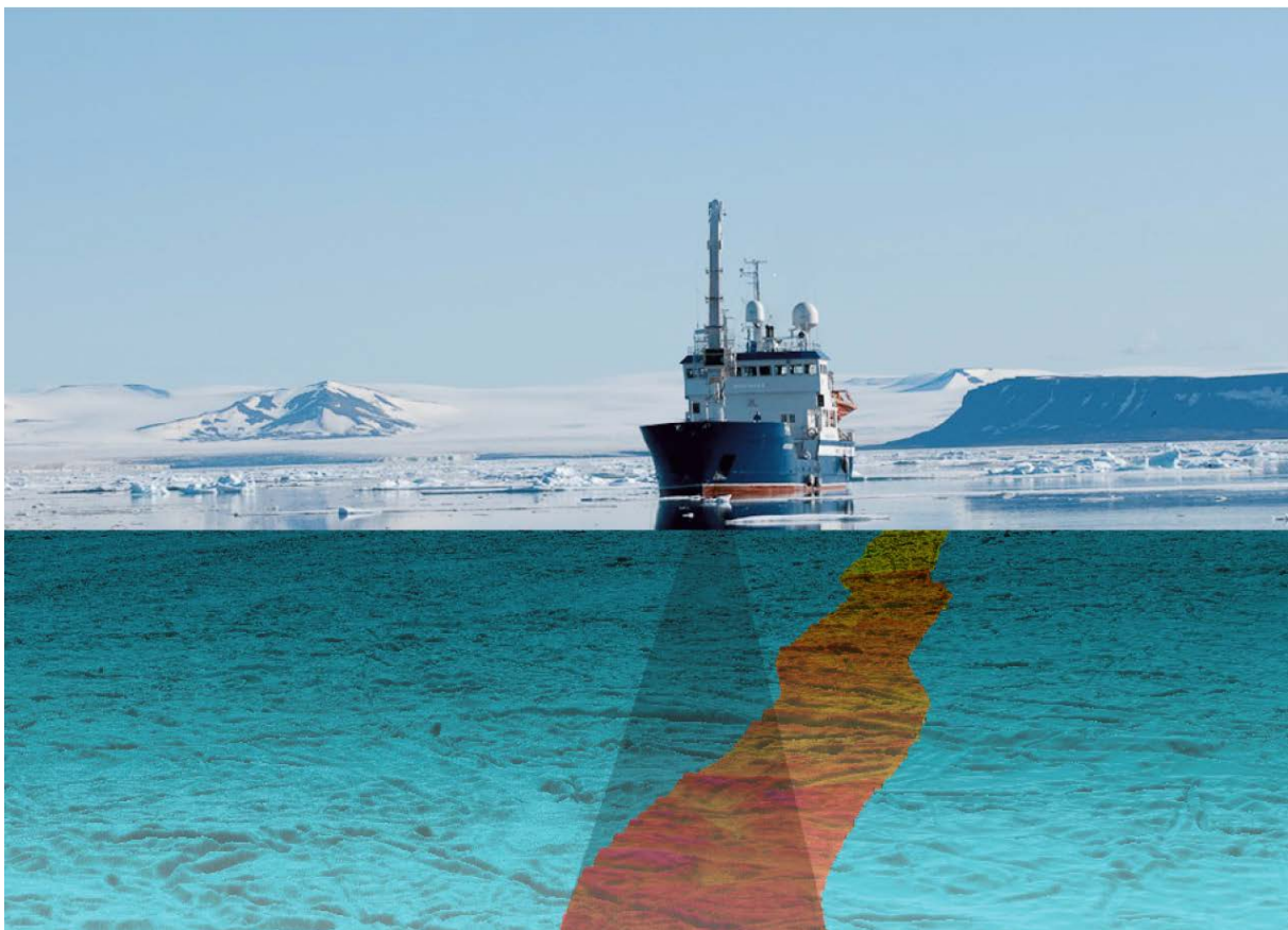
Figure 1. Illustration of surveying using multibeam echosounder.
