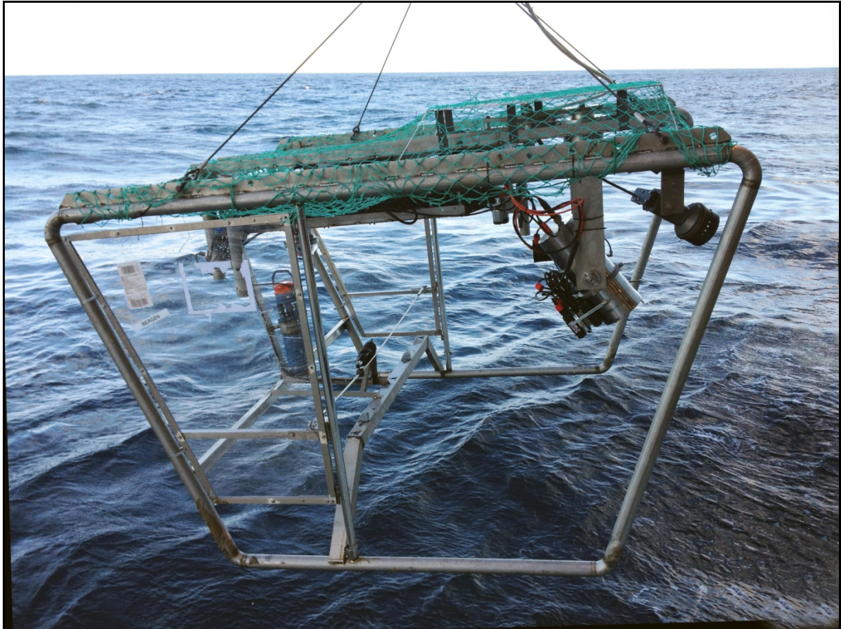
Figure 6. The video platform Chimaera has four video cameras. The main camera has High-Definition standard whereas the three additional cameras have Standard Definition. In addition, the video platform has current meters (short range ADCP) and sensors for temperature, salinity, and optical backscatter.
