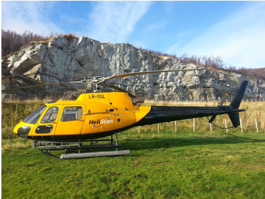
Figure 4: The Eurocopter AS350-B3 with the additional floats attached to its landing skids, that was used to conduct measurements over the lakes.
