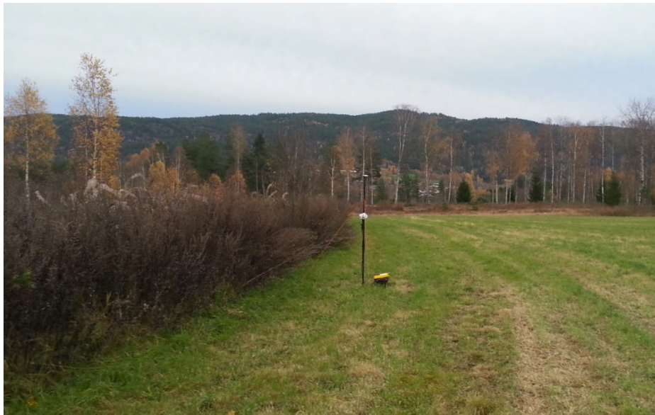
Figure 3: A base station magnetometer (GEM GSM-19) installed 4 km northwest of Notodden
