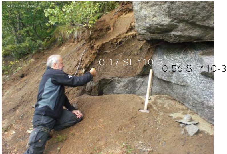
Figure 11.10. Magnetic measurements of weathered and unweathered bedrock on Hamarøya. The remaining magnetisation of the altered rocks is c. 30% lower than the parent material. Observations at other locations show a reduction of magnetisation by 50% and up to one order of magnitude.
