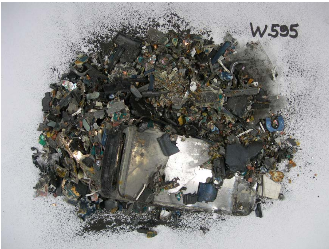
Figure 4. Electronically fragmented Sony Ericsson W595 mobile phone.
