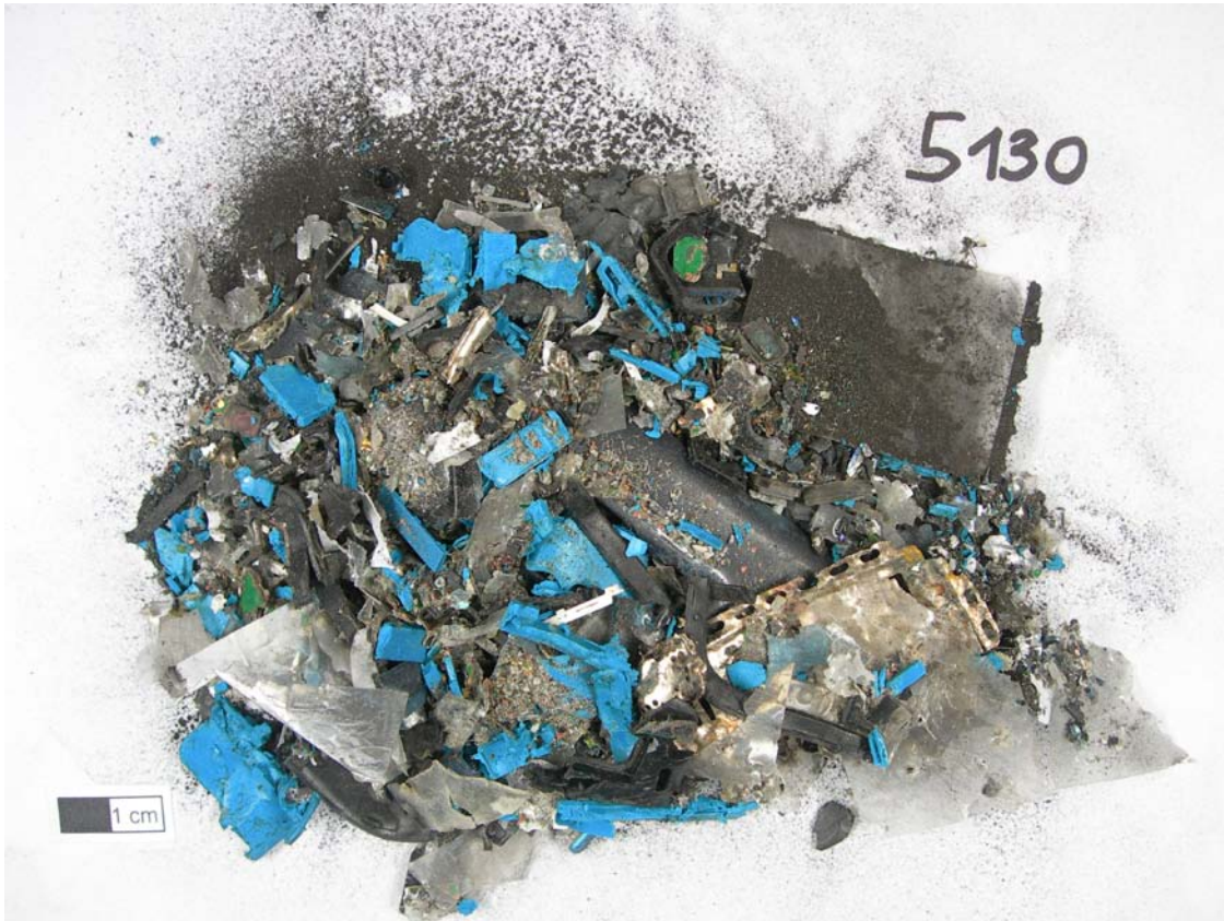
Figure 3. Electronically fragmented Nokia 5130 mobile phone.
