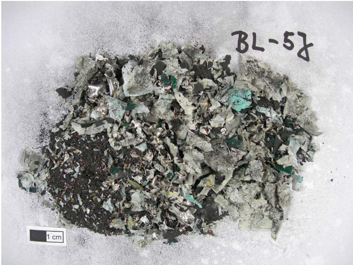
Figure 5. Electronically fragmented Nokia BL-5J Li-ion battery.
