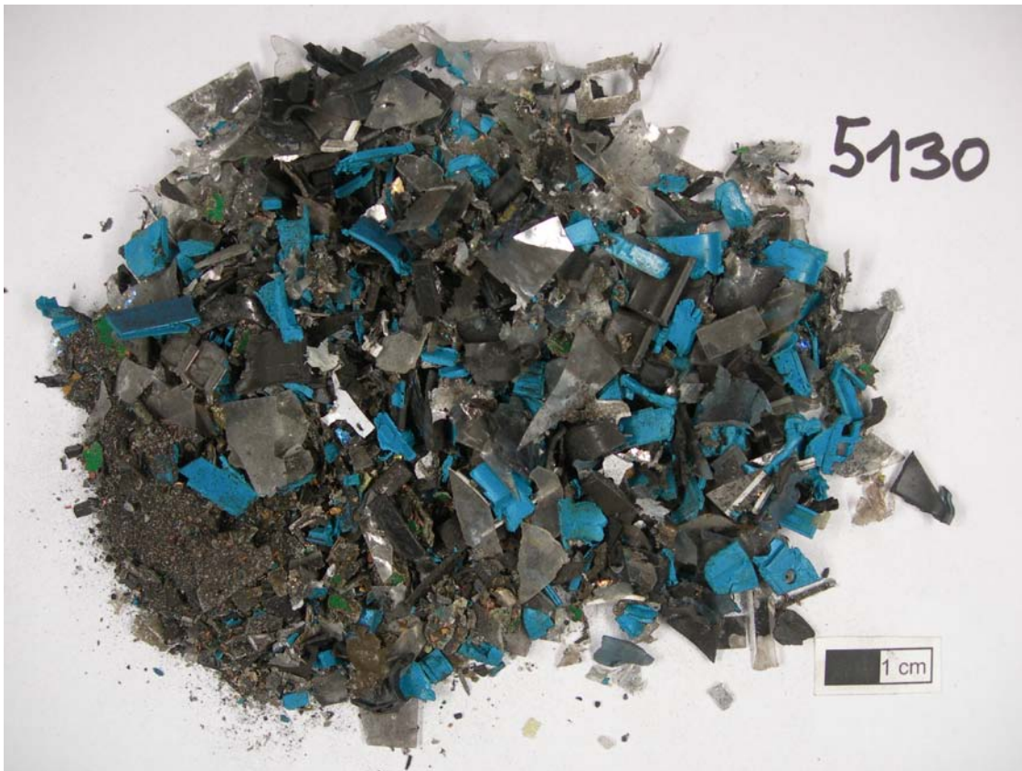
Figure 9. Electronically fragmented Nokia 5130 mobile phone. Components >1 cm were cut manually.
