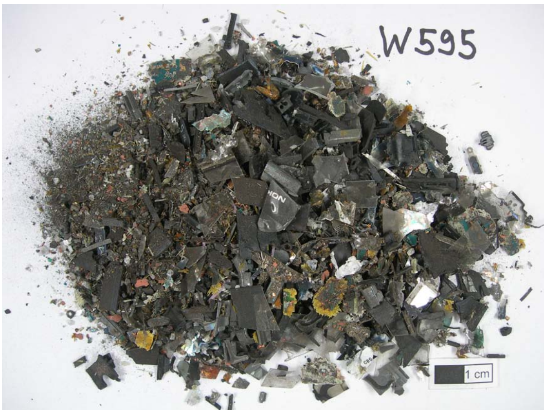
Figure 10. Electronically fragmented Sony Ericsson W595 mobile phone. Components >1 cm were cut manually.
