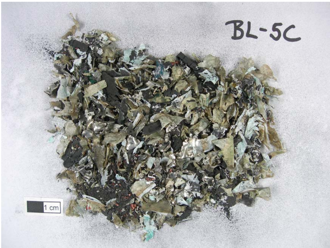
Figure 6. Electronically fragmented Nokia BL-5C Li-ion battery.
