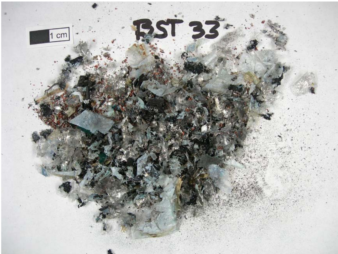
Figure 7. Electronically fragmented Sony Ericsson BST-33 Li-polymer battery.
