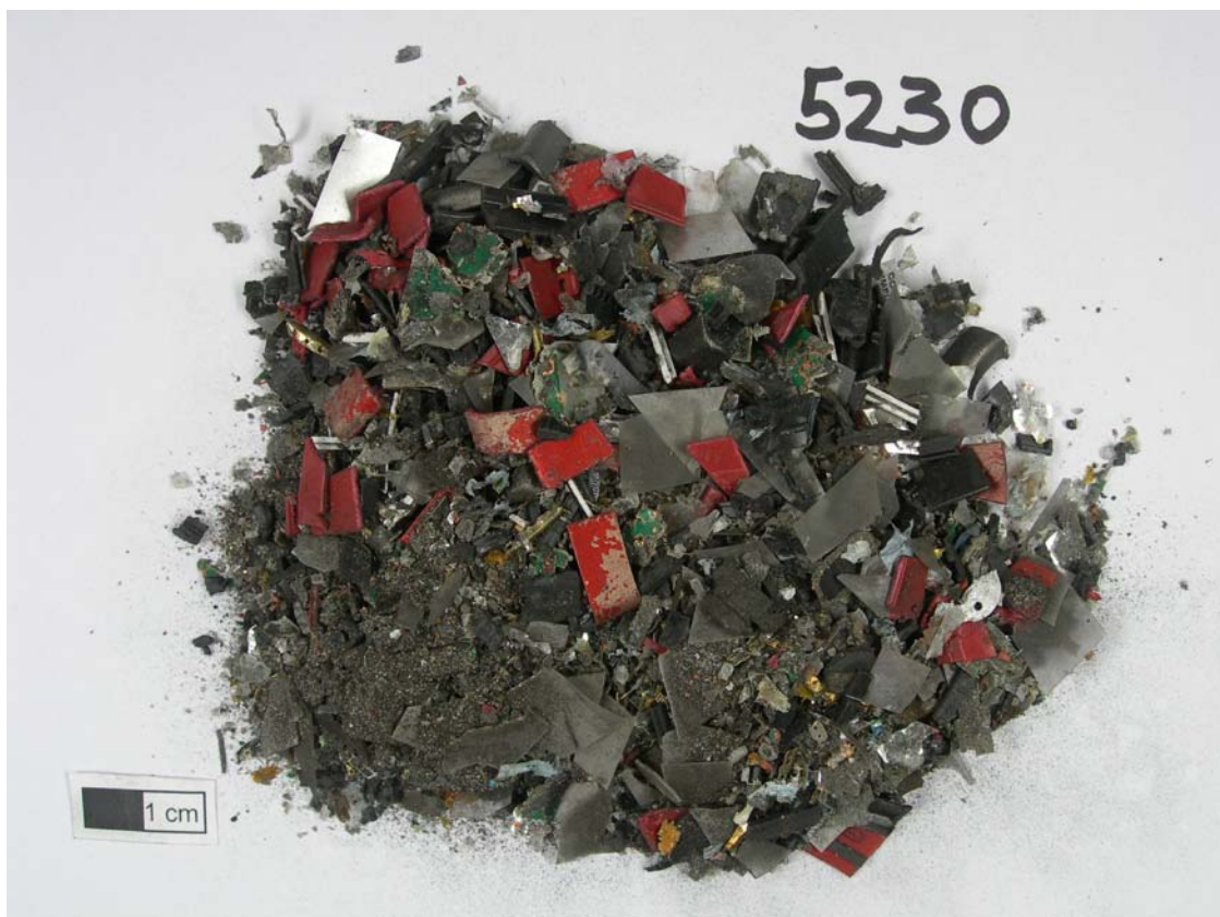
Figure 8. Electronically fragmented Nokia 5230 smart phone. Components >1 cm were cut manually.
