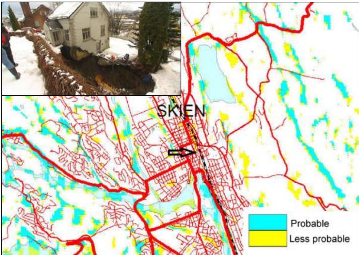
Figure 12. Interpreted deep weathered zones in the Skien area where an admit tunnel to an underground parking area in bedrock collapsed in 2009. Note that the method is able to indicate zones of probable and less probable deep weathering in urban areas.
