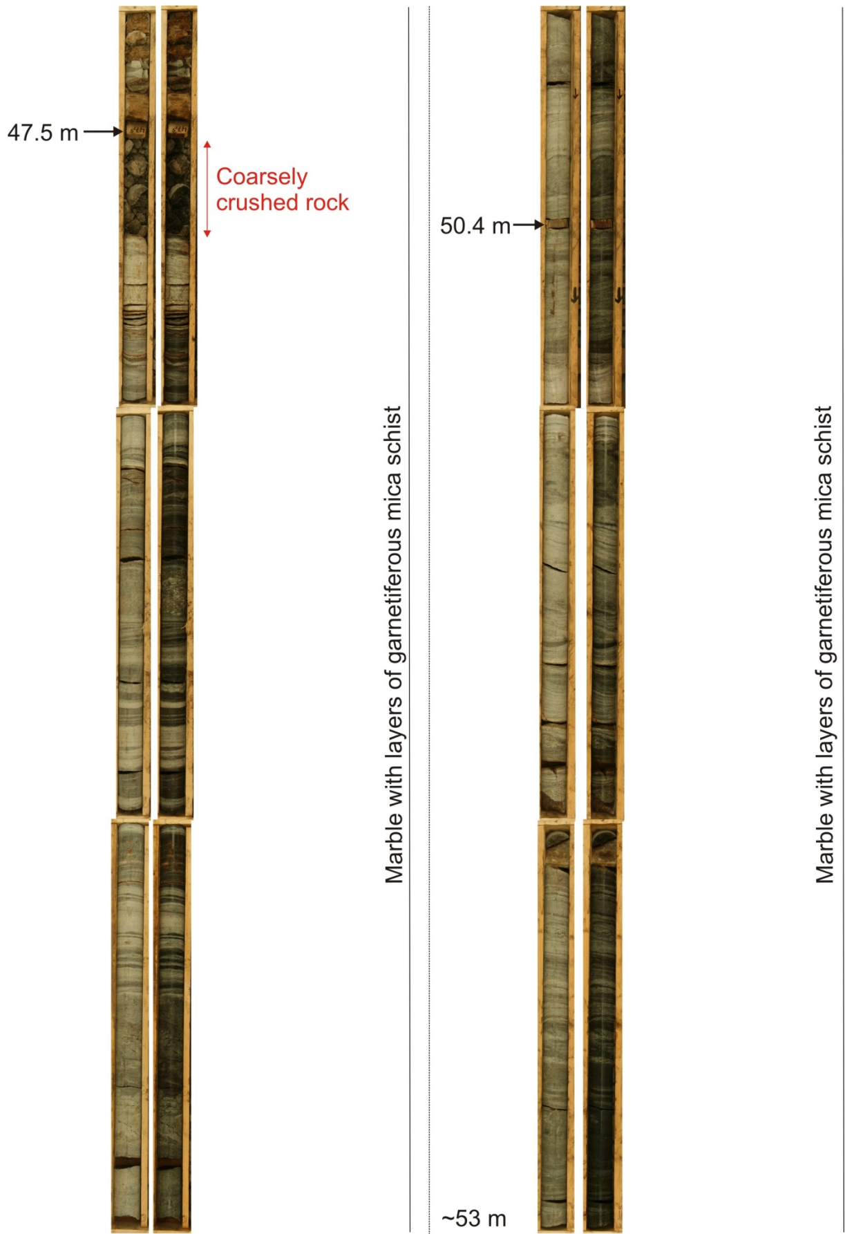
Figure 18. Geological core logging from ~47.2 to ~53 m depth with pictures of the dry (left) and wet (right) core.
