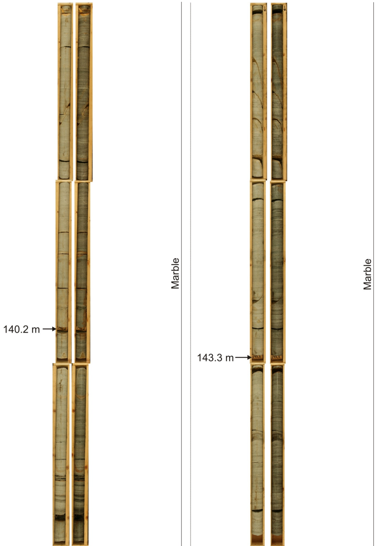
Figure 34. Geological core logging from ~139 to ~144 m depth with pictures of the dry (left) and wet (right) core.
