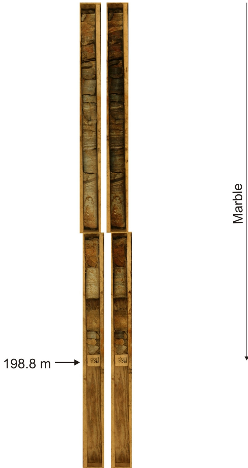
Figure 44. Geological core logging from ~197 to ~198.8 m depth with pictures of the dry (left) and wet (right) core.
