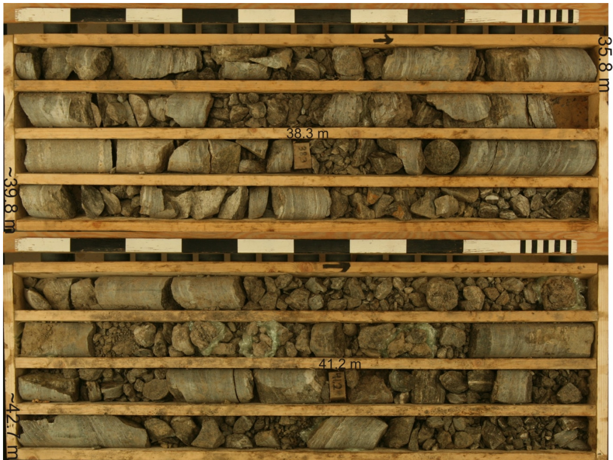
Figure 1. Pictures of the main zone of crushed rock, containing highly fractured and crushed rock with possibly clay at ~37.3~42 metre.
