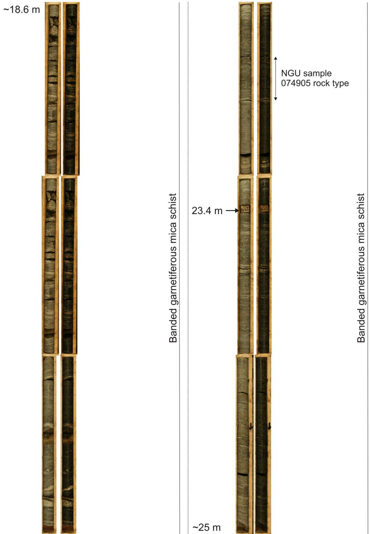
Figure 13. Geological core logging from ~18.6 to ~25 m depth with pictures of the dry (left) and wet (right) core.
