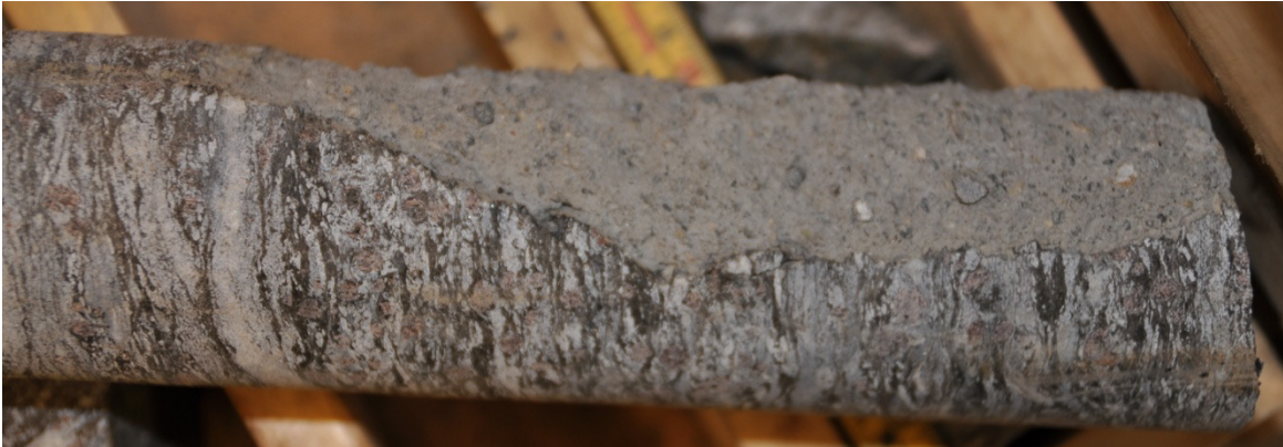
Figure 5. At ~18.30-18.40 m sediments most likely of Quaternary age is filled in along a fracture. The sediments contain small pebbles in clay/silt matrix.
