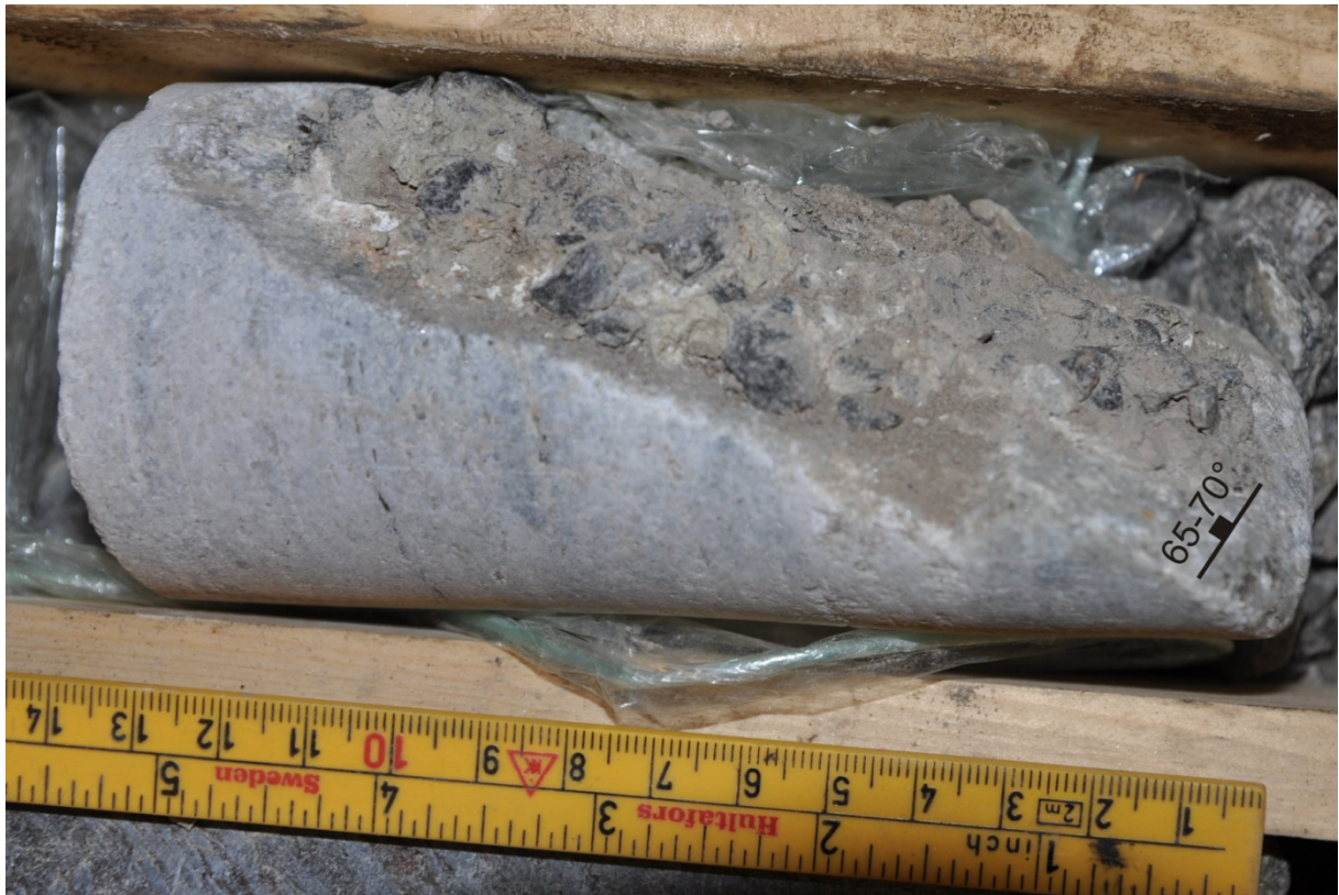
Figure 3. The old fault has a layer of breccia along the sliding plane, and is likely to contain calcite with deformed schist clasts at ~45.5 m. The fault plane is steep and the dip is estimated to 65-70°.
