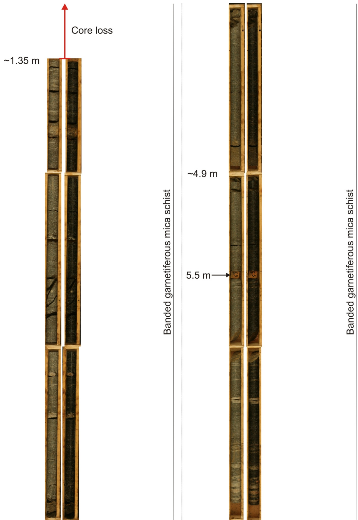
Figure 10. Geological core logging from ca. 1.35 to ~6.8 m depth with pictures of the dry (left) and wet (right) core.
