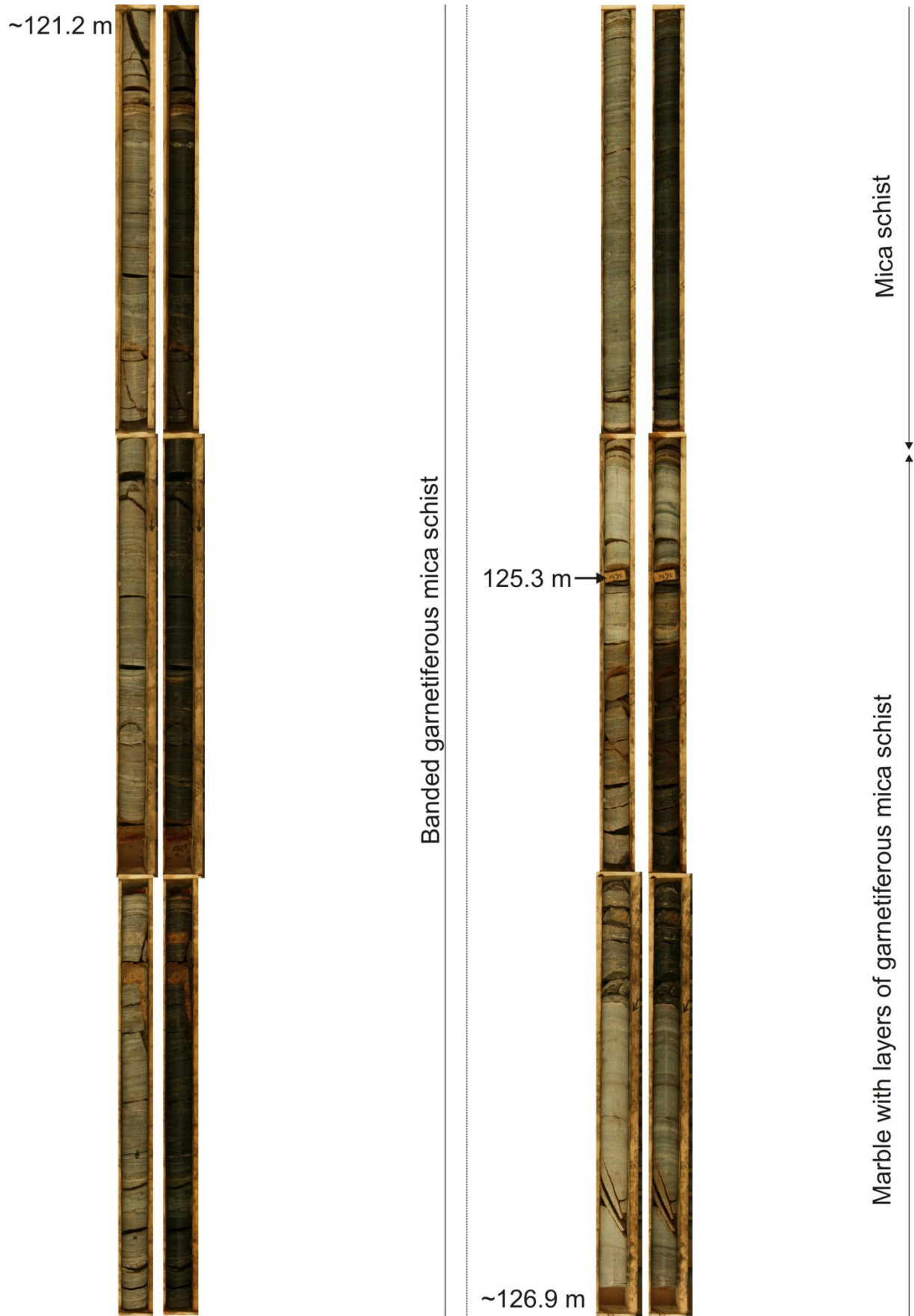
Figure 31. Geological core logging from ~121.2 to ~126.9 m depth with pictures of the dry (left) and wet (right) core.
