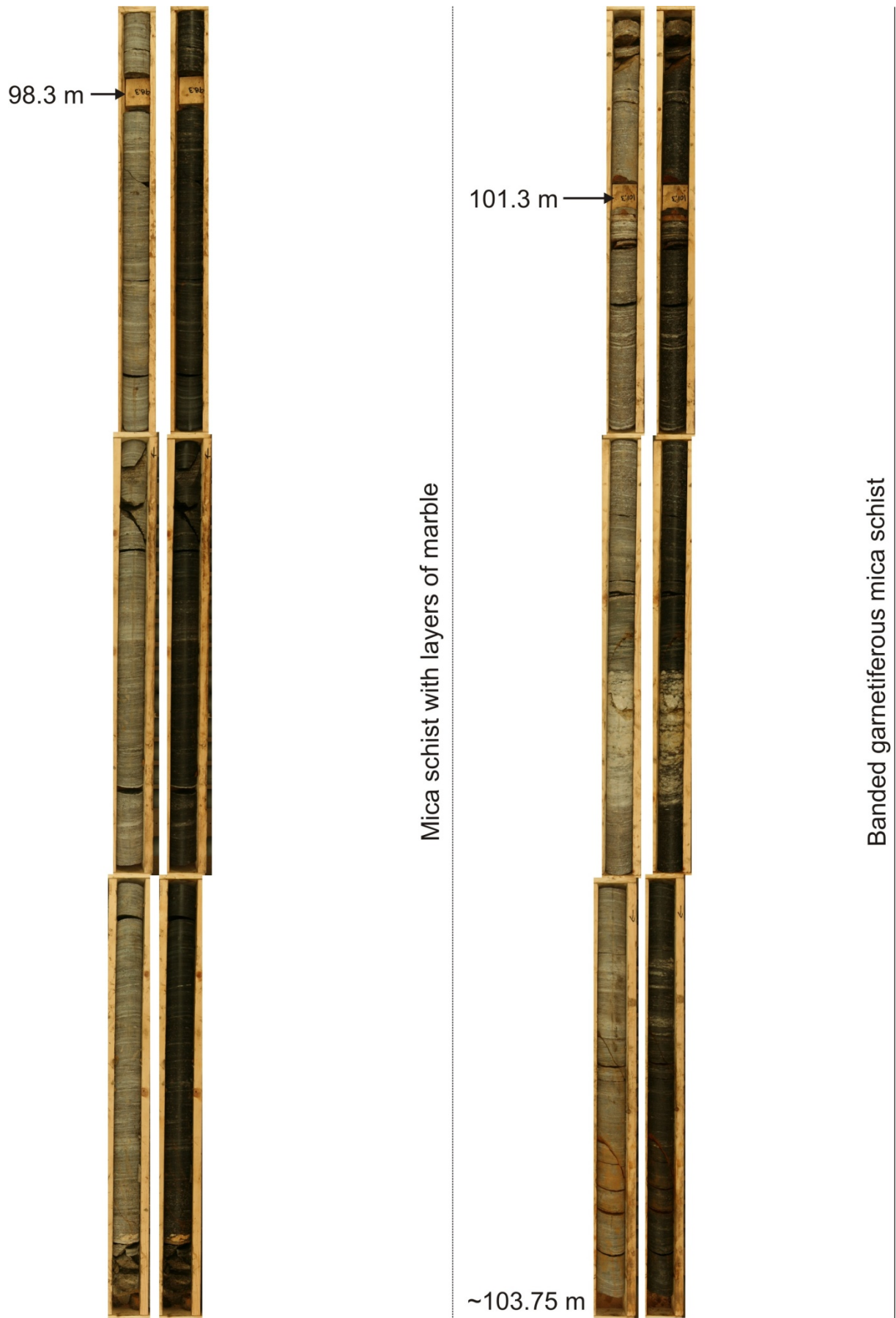
Figure 27. Geological core logging from ~98 to ~103.75 m depth with pictures of the dry (left) and wet (right) core.
