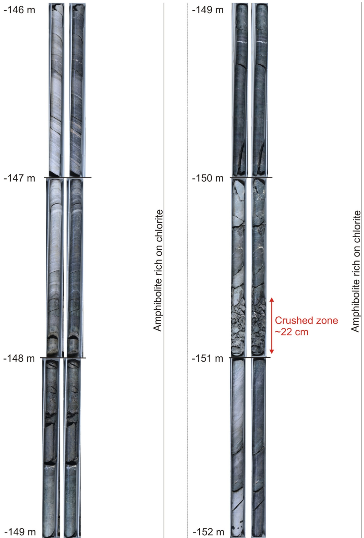
Figure 33. Geological core logging from 146 to 152 m depth with pictures of the dry (left) and wet (right) core.
