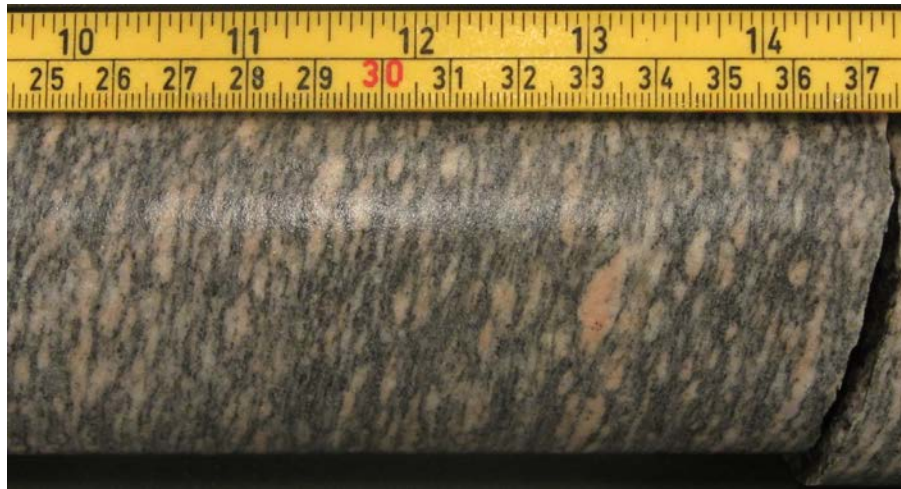
Figure 2. Example of augen structure in granitic gneiss, here at 4.25-4.37 m.
