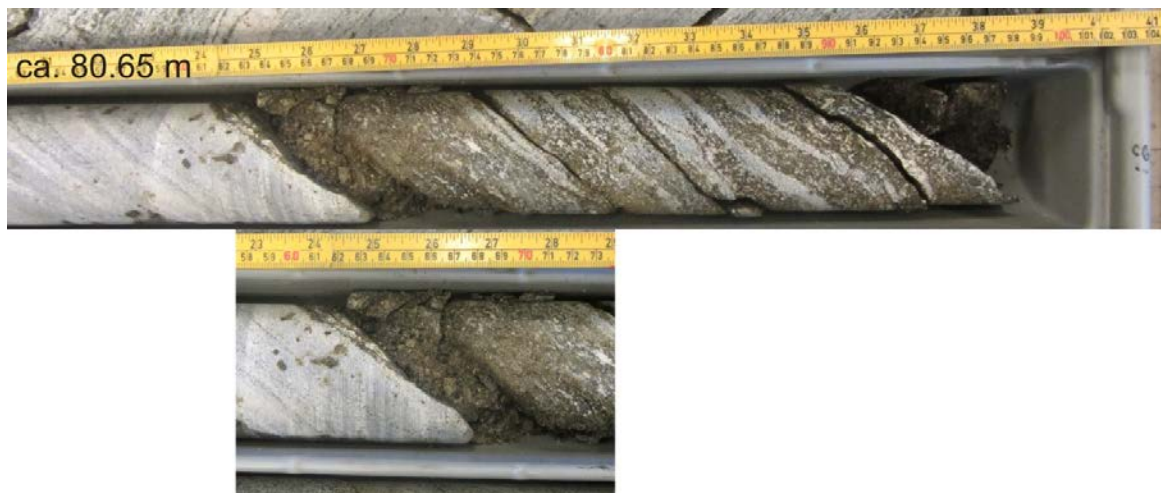
Figure 5. The mica (biotite) rich zones are prone to fracturing (crushing) as seen at ca. 80.65 m.
