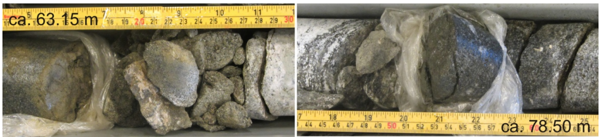
Figure 4. Clay zones at ca. 63.15 m and 78.50 m. The first is 1-2 cm thick and in combination with a zone of crushed rock, while the latter is ~1 cm thick and along a fracture.
