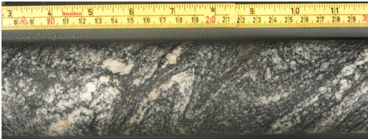
Figure 1. Example of folded foliation, here at 132-132.40 m.
