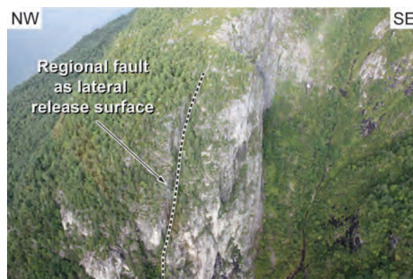
Figure 63: Photographs of the Kvarvesnippen instability: an eroded regional fault forms a potential lateral release surface and the instability is free on all other sides.
