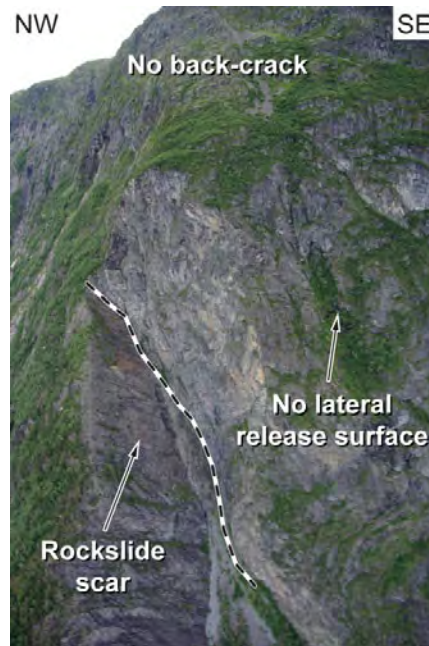
Figure 87: Photograph of the potential unstable rock slope at Kloven: the basal sliding surface of a past rockslide likely continues into the mountainside. The lack of back-crack and lateral release surface indicates that no past displacement occurred at this potential instability.
