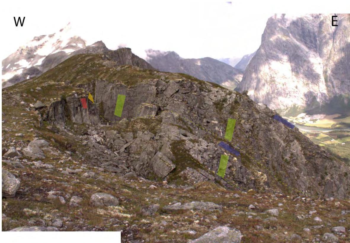
Figure 21: Panoramic view of the back graben site. 4 discontinuity sets are visible (green=J1, yellow=J2, blue=J3, red=J4).
