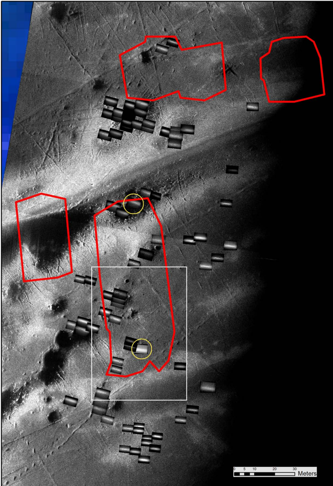
Figure 51. SAS image from the western flare site, Area B. Gas flares are shown as red outlines. Gas bubble locations are marked by yellow circles. TFish images with carbonate crusts and other seep related features are overlain. The location of figure 52 is indicated by the white rectangle.
