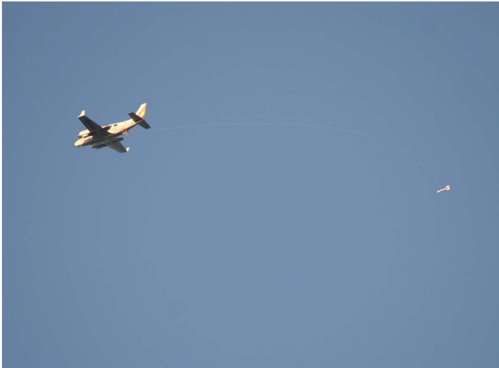
Figure 1.1 Piper Chieftain from Fly Taxi Nord AS with the towed Scintrex Caesium Vapour MEP 410 high-sensitivity magnetometer. (Photo: Aasmund Gylseth)
