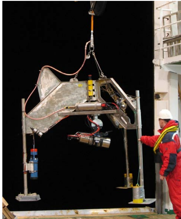
Figure 7. Photo of the CAMPOD video rig onboard R/V “G.O. Sars”.
