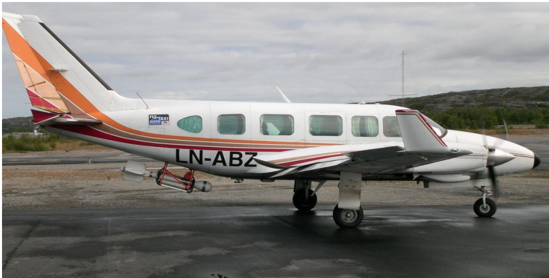
Figure 2.3 Piper Chieftain from Fly Taxi Nord with the docking cradle for the bird containing a Scintrex Cesium Vapour MEP 410 high-sensitivity magnetometer.
