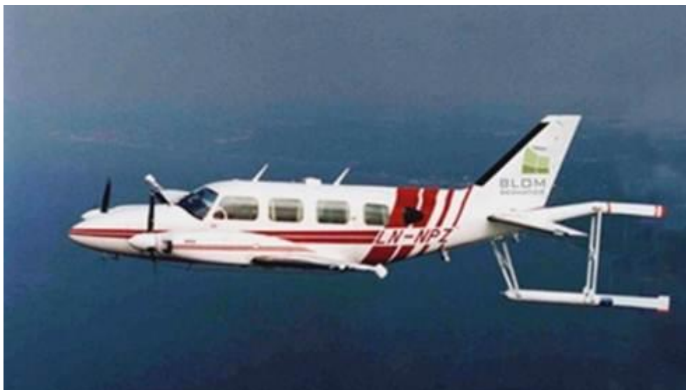
Figure 2.2 Piper Navajo PA-31 and the Geometrix G-822 high-sensitivity magnetometer, installed in a tail stinger used by Blom Geomatics AS during the first phase of acquisition in 2011.
