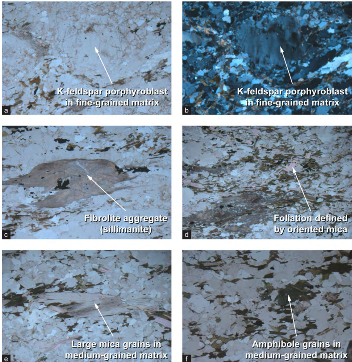
Figure 2: Microscope photographs of the thin-sections of rock samples from KH-02-11: a) sillimanite-bearing augengneiss (NGU sample # 67359) large K-feldspar porphyroblast within fine-grained matrix (image width: 2.7 mm); b) as in a) but with crossed nicols; c) fibrolite aggregate within sillimanite-bearing augengneiss (NGU sample # 67359, image width: 2.7 mm); d) sillimanite-bearing augengneiss (NGU sample # 67360) with foliation defined by oriented mica (image width: 5.3 mm); e) muscovite-rich gneiss (NGU sample # 67361) with coarse mica grains within medium-grained matrix (image width: 1.4 mm); f) medium-grained amphibolitic gneiss (NGU sample # 67363) with amphibole grains (image width: 2.7 mm).
