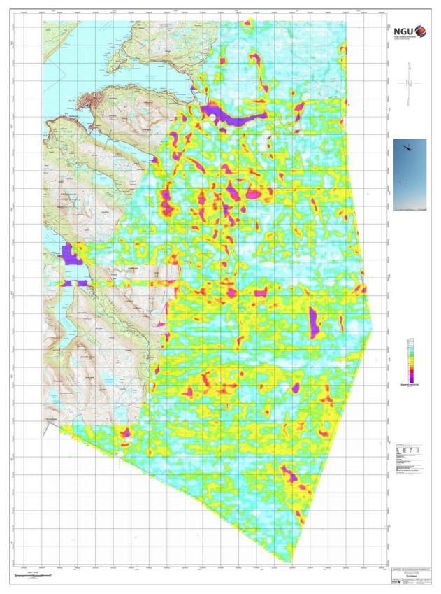
Figure 9. Apparent resistivity. Frequency 980 Hz, Coaxial coils
