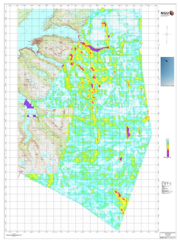
Figure 7. Apparent resistivity. Frequency 880 Hz, Coplanar coils
