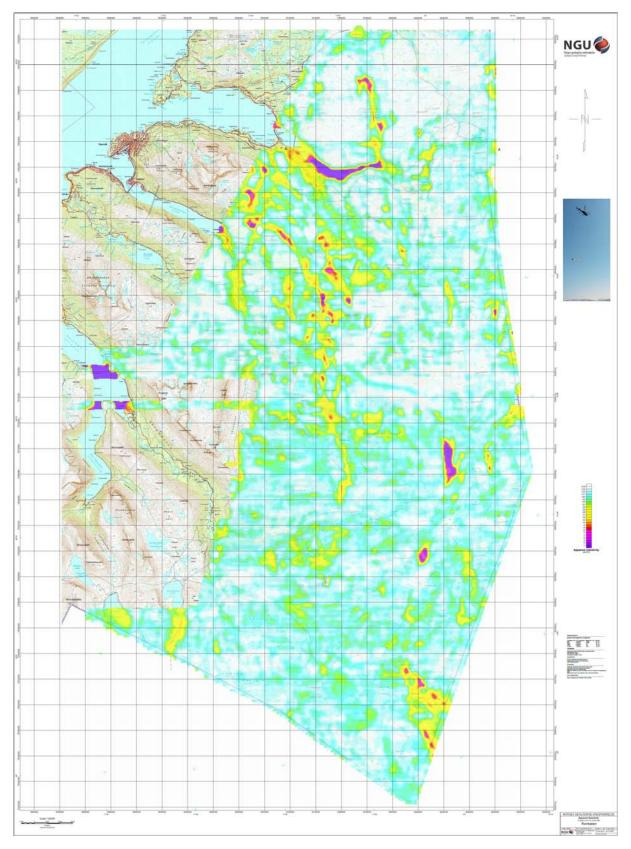
Figure 8. Apparent resistivity. Frequency 7000 Hz, Coaxial coils
