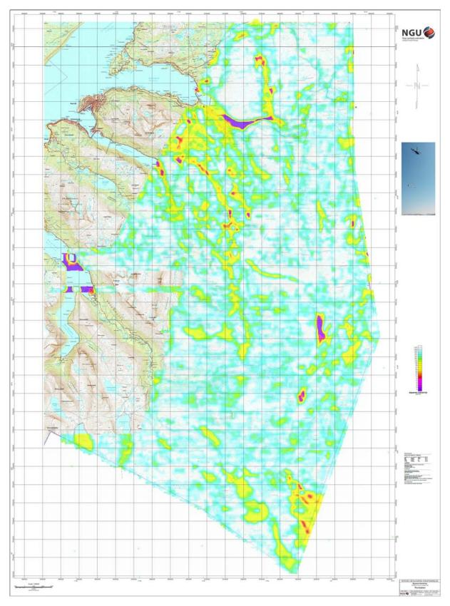
Figure 6. Apparent resistivity. Frequency 34000 Hz, Coplanar coils
