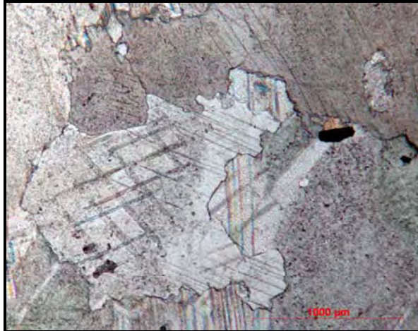
Figure 38: Microphotograph of irregular calcite crystal boundaries. Thin-section LR3-12.2 m.
