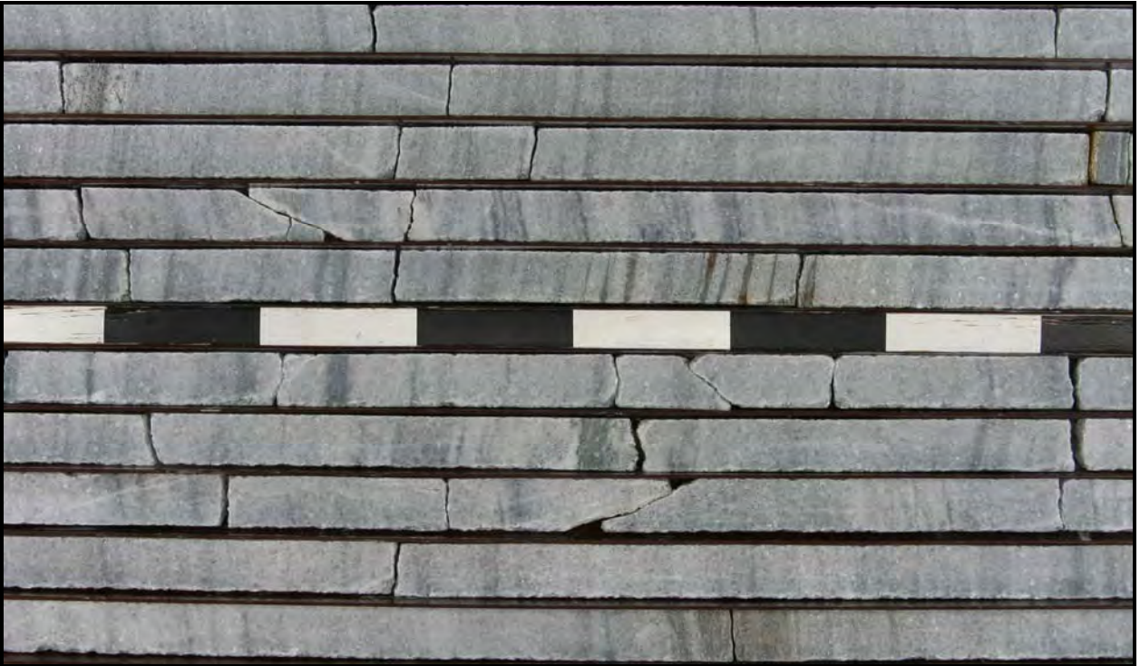
Figure 81: Core photograph showing white to pale grey distinctly banded calcite marble (units 2 and 3).
