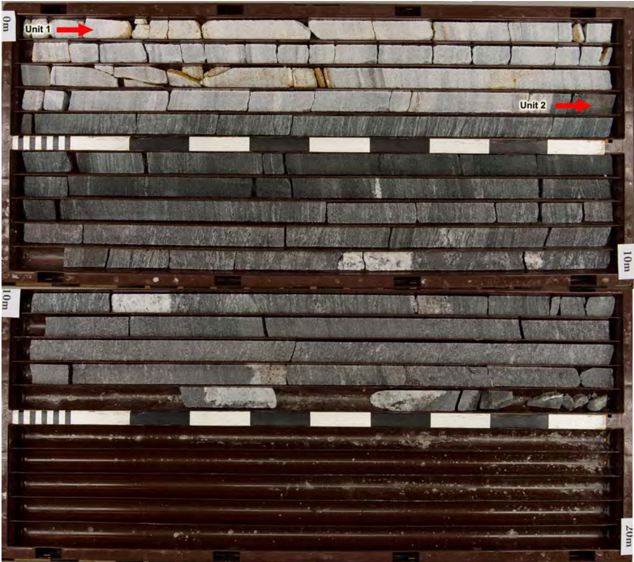
Figure 2: Overview photo of core LR1, Breivollia. Unit 1 is white or greyish calcium carbonate marble while unit 2 is amphibolitic gneiss.
