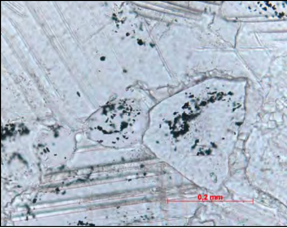
Figure 20: Microphotograph showing graphite (black) inclusions in carbonate. Thin section LE2-07.4 m.
