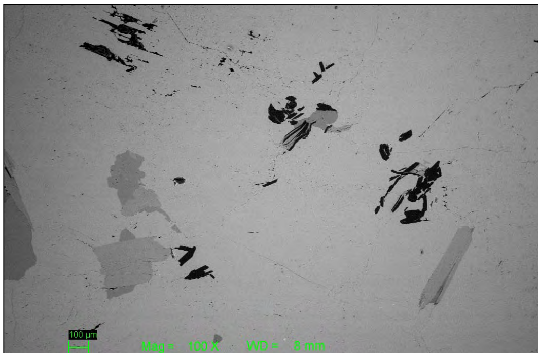
Figure 77: SEM BSE-image of calcite, mica (elongated medium grey minerals), feldspar and quartz (dark grey) and graphite (black). Thin-section LR5-23.9 m.
