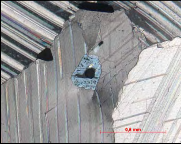
Figure 21: Microphotograph of unknown mineral (bluish) and graphite (black) within large calcite crystal. Thin-section LR2 12.9 m.
