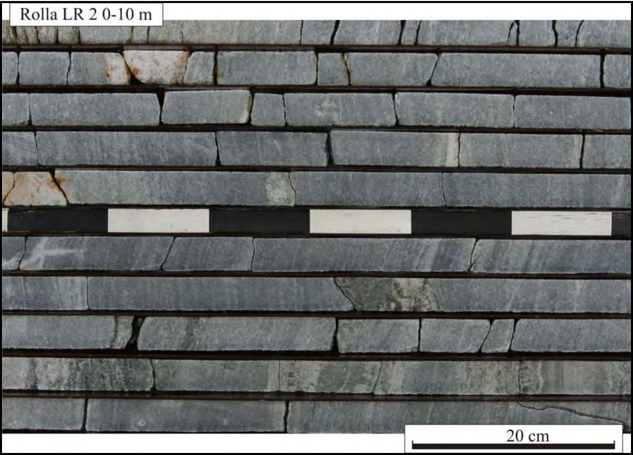
Figure 9: Photograph of fine to medium grained, variably banded, dark-greenish marble enriched in silicate minerals.
