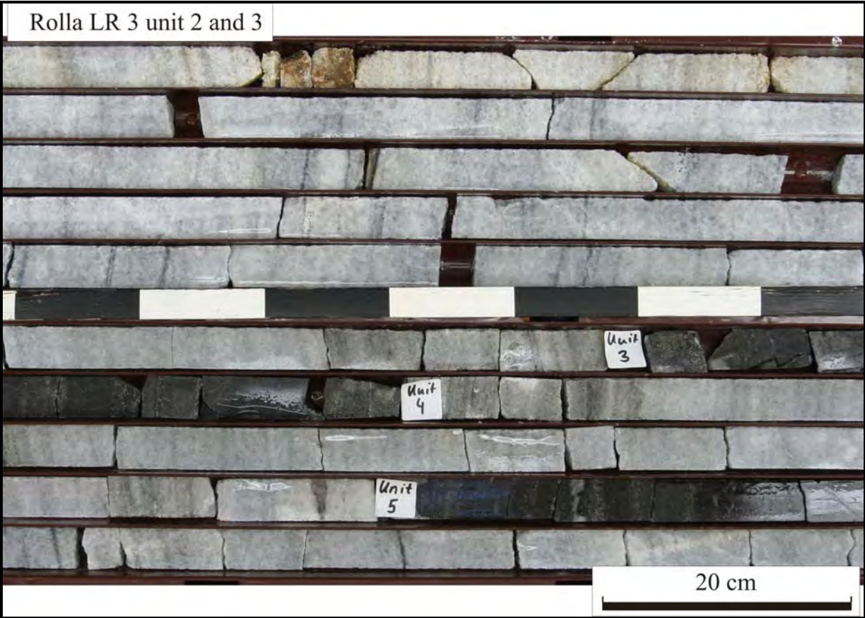
Figure 31: Core photograph of white marble with layers of amphibole-rich schist, core LR3.
