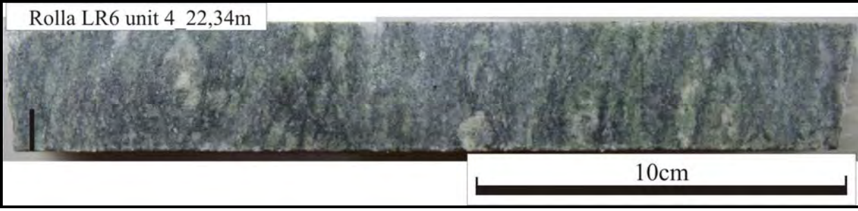
Figure 85: Close-up core photo of impurte carbonate / gneiss. LR6 at 22,3 m.
