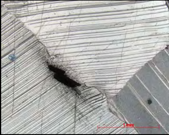
Figure 20: Microphotograph showing graphite (black) on calcite grain boundary. Thin-section LR2 12.9 m.
