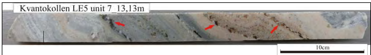
Figure 65: Photo of very heterogeneous, alternating pinkish and grayish calcite-dolomite marble, LE5 unit 7 at 13,1 m.
