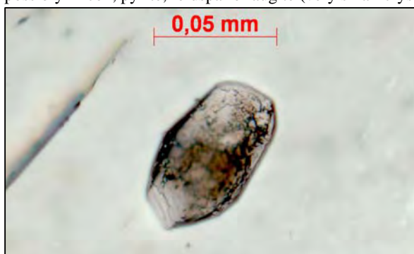
Figure 71: Microphotograph of zircon within carbonate; parallel-polarized light. Thin section LE5-04.8 m.
