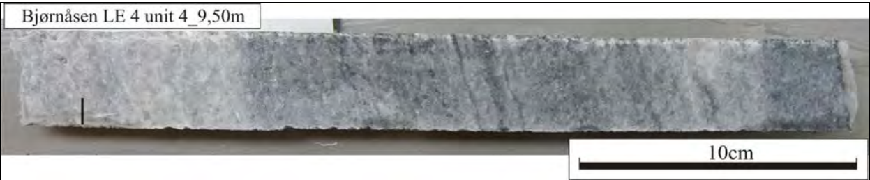
Figure 42: Photo of weakly banded light grey to dark grey marble, Bjørnåsen LE4 unit 4 at 9,5 m.
