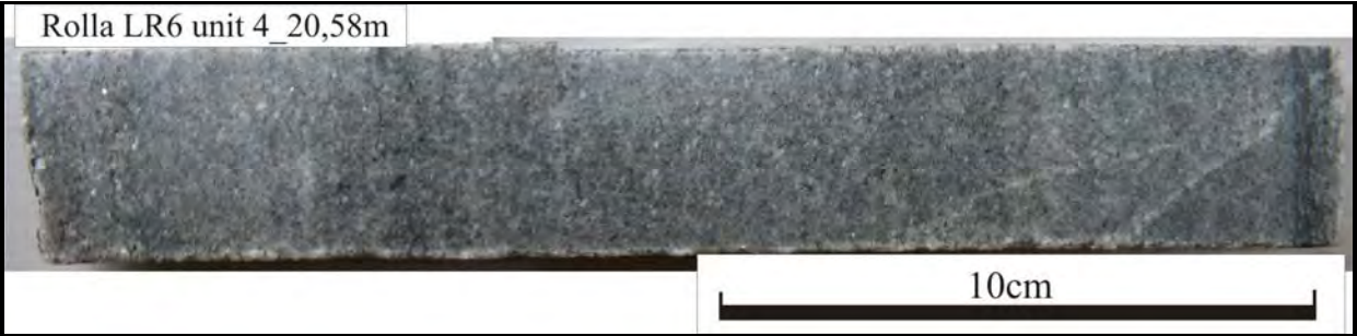
Figure 84: Close-up core photo of grey-green, medium to fine grained impure carbonate. LR6 at 20.6 m.
