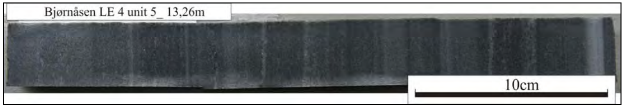
Figure 43: Photo of dark grey, fine-grained thinly banded and strongly dolomitised marble, Bjørnåsen LE4 unit 5 at 13,3 m.
