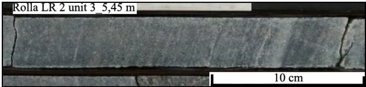
Figure 10: Weakly banded, dark grey marble enriched in silicate minerals, LR2 at 5,5 m.
