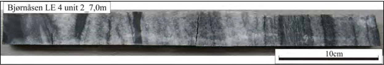
Figure 41: Photo of heterogeneous banded light grey to dark grey calcite-dolomite marble, Bjørnåsen LE4 unit 2 at 7,0 m.
