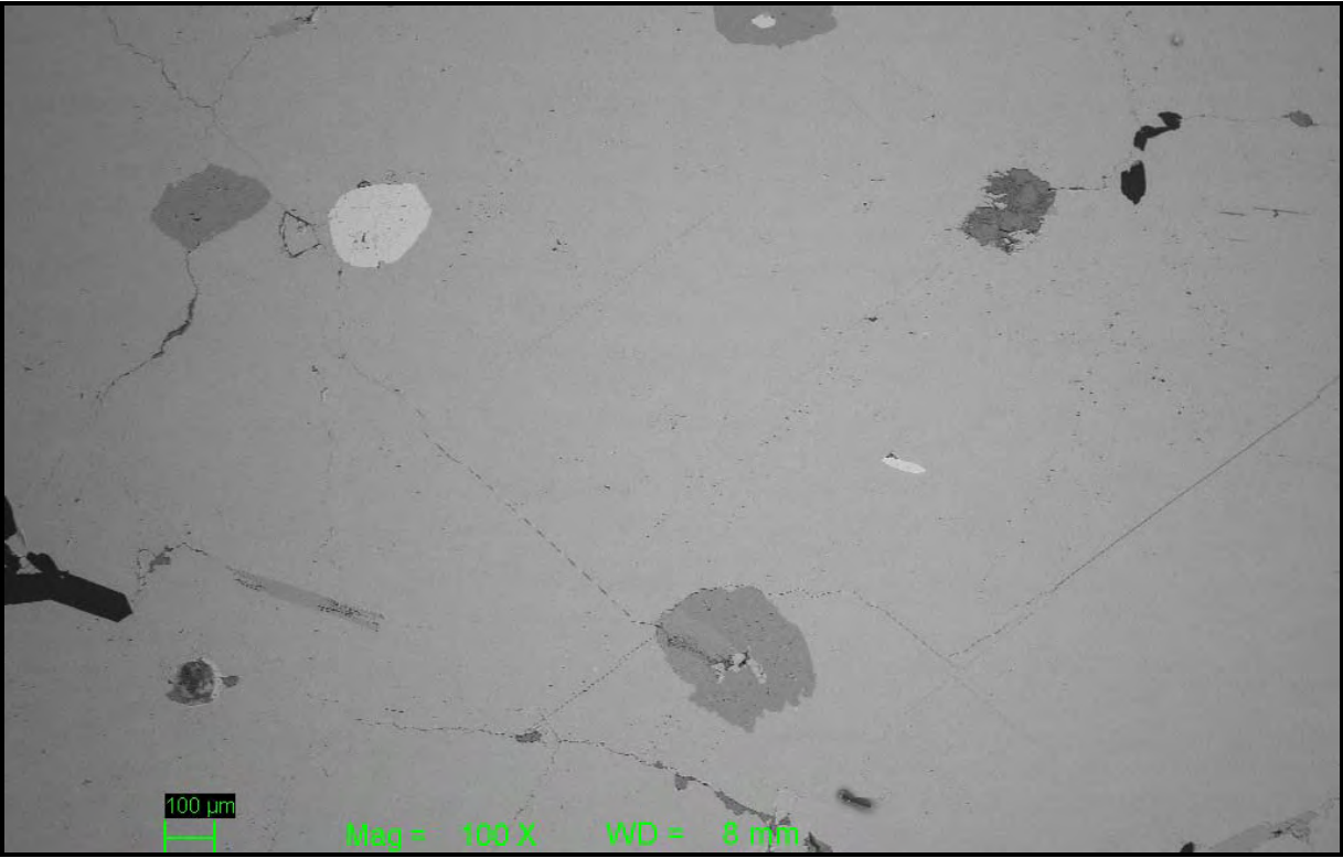
Figure 66: SEM BSE-images showing inclusions of other minerals in calcite; graphite (black), quartz (dark grey), apatite (light grey) and calcite (medium grey). Thin-section LR5-09.0 m.
