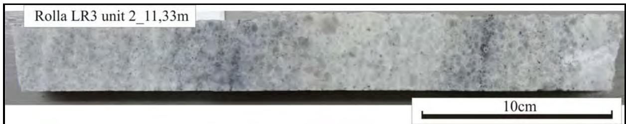
Figure 34: Close-up core photo of coarse-grained marble with diffuse layers enriched in graphite. LR3 at 11,3 m, unit 2
