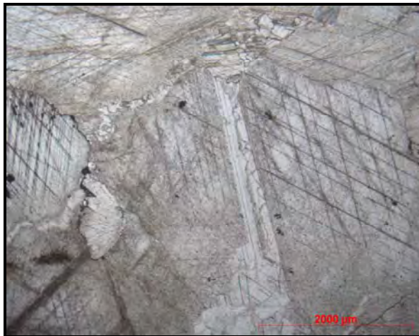
Figure 40: Microphotograph of partly recrystallised calcite carbonate. Thin-section LR3-12.2 m.
