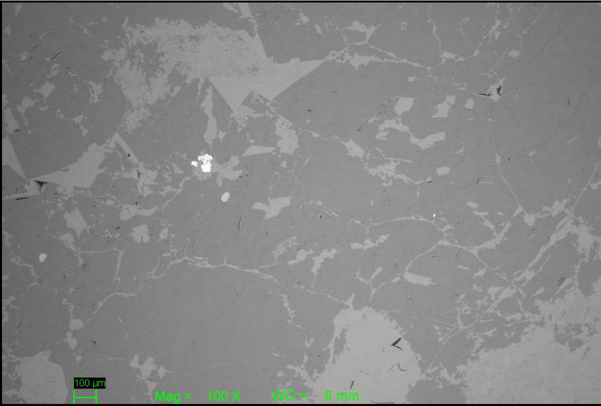
Figure 51: SEM BSE-image of dolomite (dark grey), calcite (grey), pyrite (white) and graphite (black). Thin-section LR3-21.9 m.
