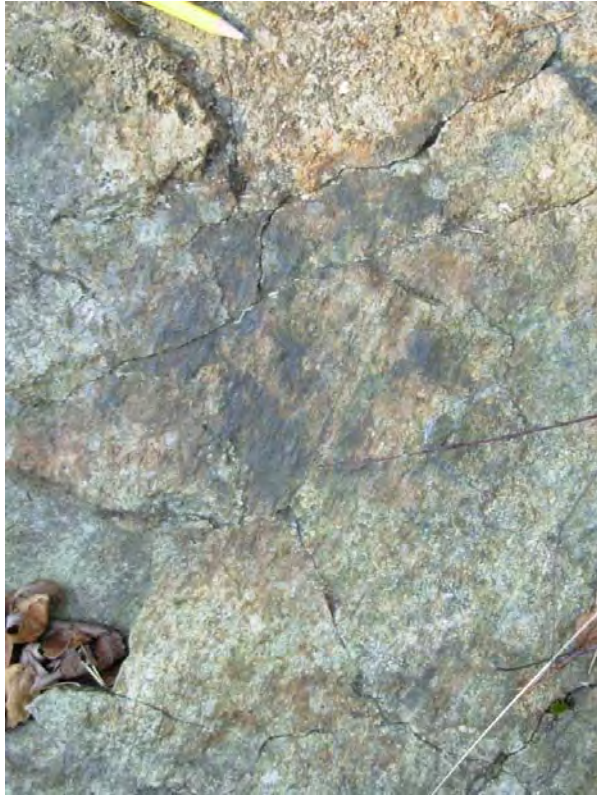
Figure 108. Photograph (view to N) of a striated fault measured at field point “Skoglia_1” (located on Figure 103) with strike/dip angle: N090/52 and pitch of striation: 80W.
