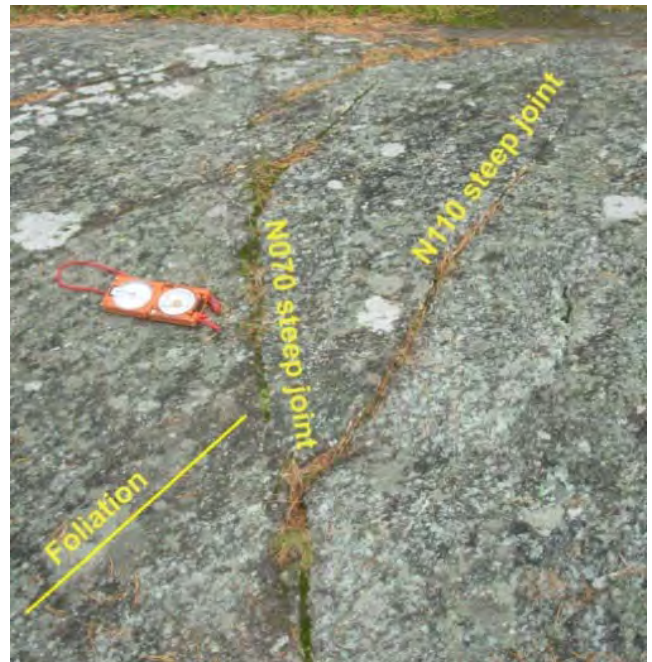
Figure 36. Structural field measurements displayed by rose diagrams and on stereonets at locality “Ekeberg Rideskole” close to resistivity profile 0 (keys to stereonets on Figure 32) and photograph of two fractures which belong to the two main sets of joints commonly found at the regional scale, which are the steep WSW-ENE and WNW-ESE orientated sets.
