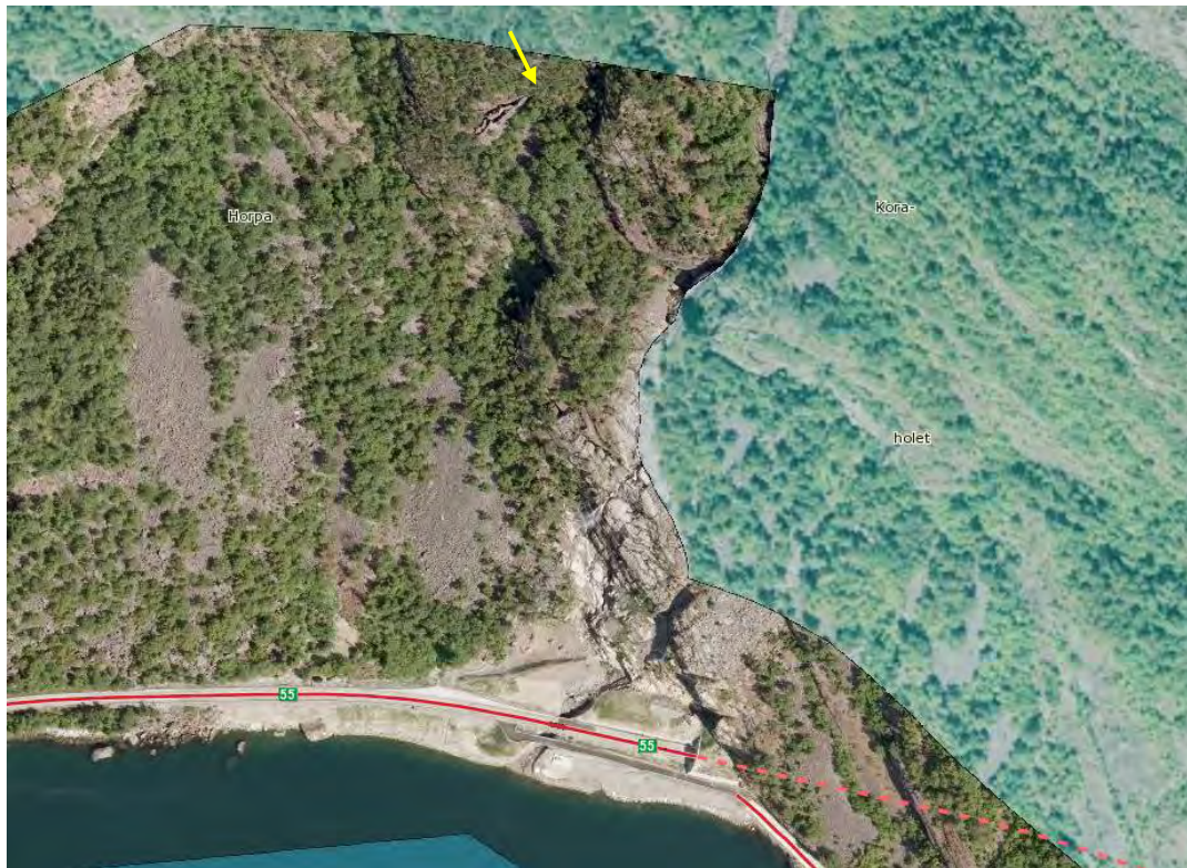
Figure 60. Orthophoto of the tunnel- entrance showing rockfall- talus beneath Anhovden and a larger, partly detached block at 6784456, 386327 indicated by arrow ( www.norgebilder.no )
