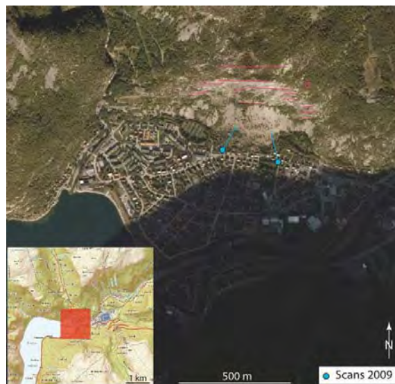
Figure 3: Scanning points of 2009 TLS data (in blue). The location of the points was estimated from field photographs, as for the overall directions (arrows) of scanning. Orthophoto from Statens Kartverk ( http://kart.statkart.no ). Pink lines indicate subvertical J5 discontinuity set.
