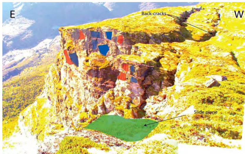
Figure 31: View from the top of the cliff with main discontinuity sets (pink=S1, red=J2, blue=J3, green=J4). The slide plane in green corresponds to the discontinuity set J4.
