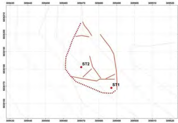
Figure 19. showing the main cracks and position of rover points at Strandanipa.
