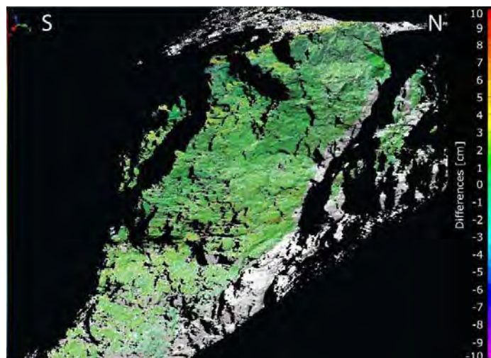
Figure 36: Piece-wise comparison between scans tussen1 (2008) and tu1a, tu1a2, tu1b (2009). No significant movement appears.
