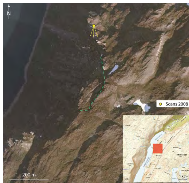
Figure 38: Scanning point of 2008 TLS data (yellow). Directions of scanning are indicated by the arrows. Green dashed line shows the limit of the instability. Orthophoto from Statens Kartverk ( http://kart.statkart.no ).
