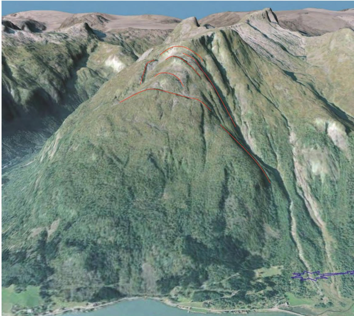
Figure 33. Frontal view of the unstable part of the Skrednipa mountain, showing several large, vertically displaced blocks.
