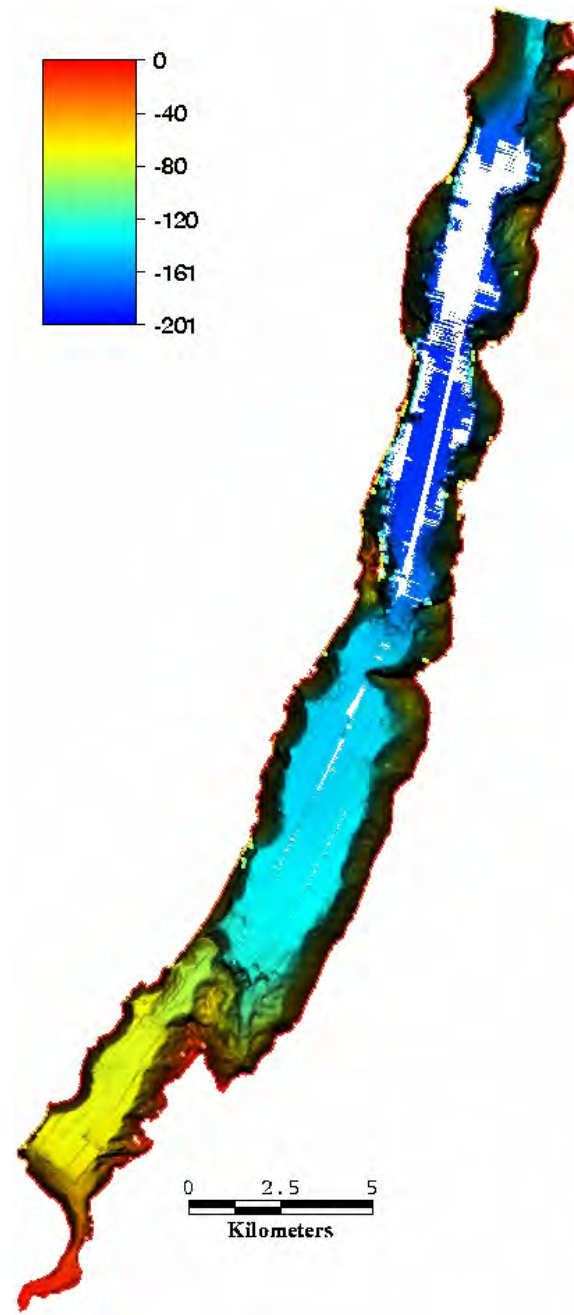
Figure 17. The bathymetry of Hyenfjord does not indicate any sub-recent rockslide deposits.
