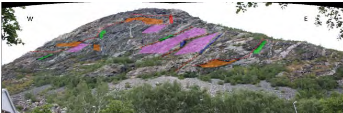
Figure 7: Panoramic view of the cliff with some examples of the main discontinuity sets (red=J1, blue=J2, green=J3, orange=J4, pink=J5).
