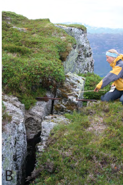
Figure 18) Strandanipa unstable area. A) Overview. The solid line marks the border of the unstable area and the dashed lines indicate open fractures and depressions that separate the block into several parts. View to the south. B) Fracture that limits the block to the east. View from the north. C) Exposed cliff on which the unstable part is located. The bedrock is highly fractured and therefore probably quite unstable below the uppermost approx. 10 m thick massive layer. View to the northeast.
