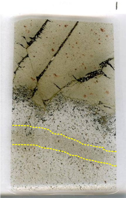
Figure 41: Photo of the cut core and scanned image of the thin section of sample H0811-13. The most carbonate-rich middle layer is marked with yellow dotted lines. Note the cracks in the upper siltstone layer. They are mainly filled with bornite, biotite and quartz.
