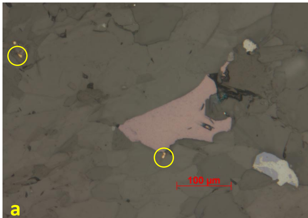
Figure 13 a: Photomicrograph of two interstitial grains of electrum in carbonate-rich sandstone where they occur intergrown with carbonate and bornite. Electrum is in contact with bornite (brown) in the lower centre of the image and composite grain of bornite (purple) and chalcocite (pale blue) to the right. b: Close-up of electrum in contact with bornite in a). The Au:Ag ratio in electrum is 1:3 (sample H0814-17A - reflected light).
