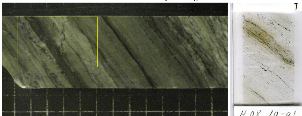
Figure 34: Photo of the cut core and scanned image of the thin section of sample H0810-01.
