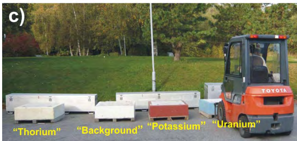
Figure 1: a) and b) illustrate the experimental arrangement for calibration measurements; c) shows the concrete calibration pads, one of which is being manoeuvred by forklift truck.
