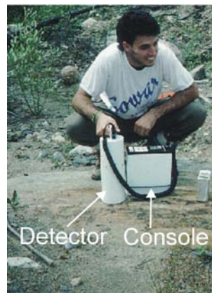
Figure 3.1. Handheld spectrometer in field (source Geological Survey of Canada).
