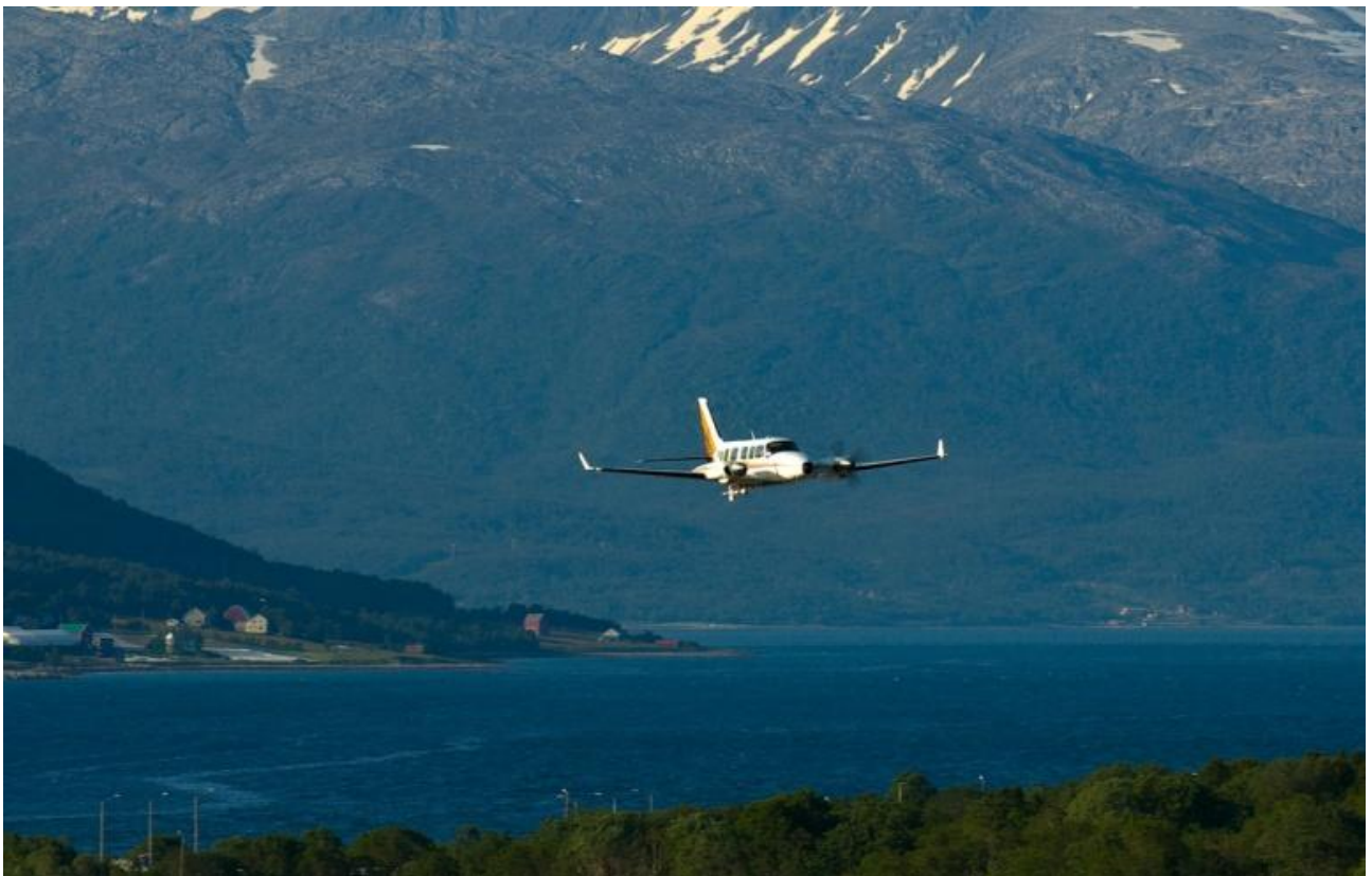
Figure 3.1 Piper Chieftain from Fly Taxi Nord with the towed Scintrex Caesium Vapour MEP 410 high-sensitivity magnetometer (still in the docking cradle).
