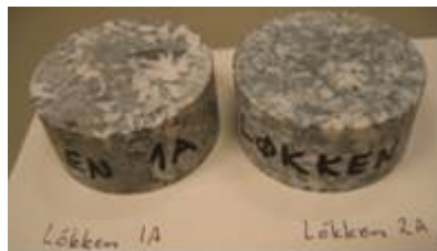
Figure 25 Photographs of the rock samples in the ring test measured at NGU.
