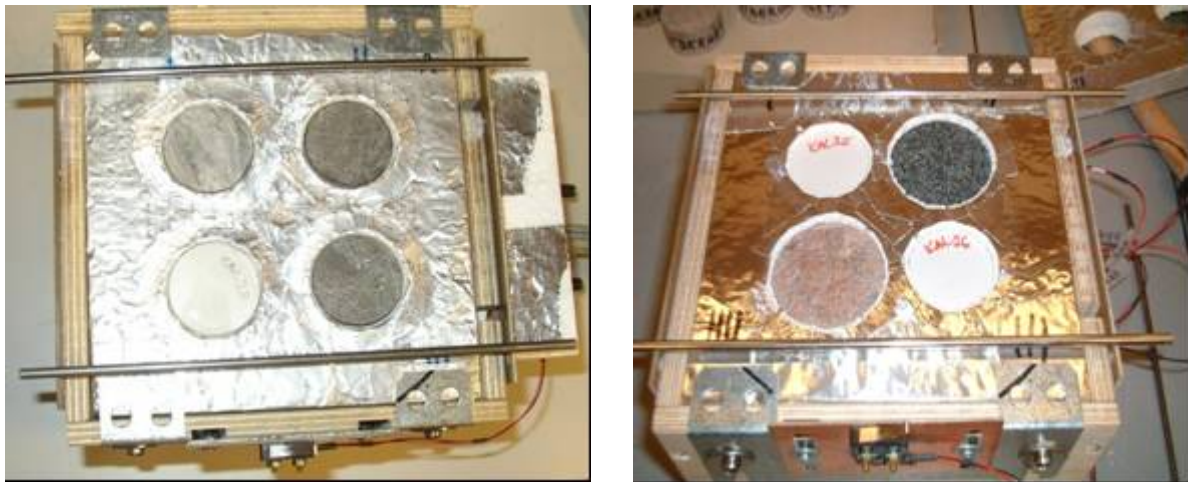
Figure 5 New sample box with standard sized samples (left), although different diameters and shapes can also be accommodated (right).
