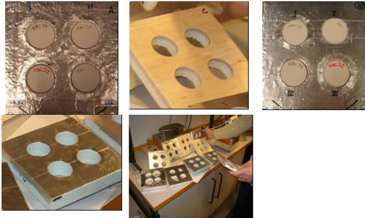
Figure 18 The different insulation plates used in the study (top row, plate A, C, G”; bottom row, plate H, I). Small variations in the material and layout of the plate should (in theory) not influence the determined thermal conductivity of the reference material.
