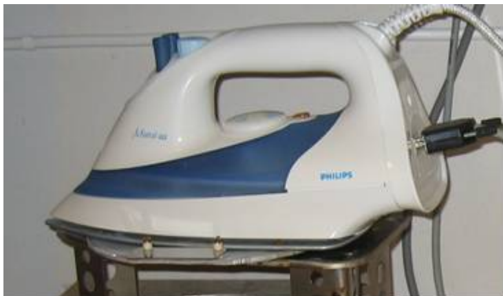
Figure 6 A disc-shaped plate of aluminium is fastened to the base of the flat iron to ensure a uniform surface temperature on the plate.
