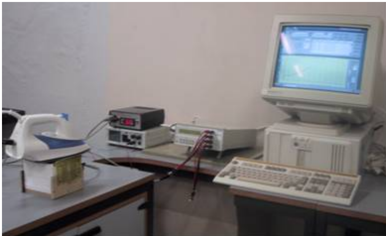
Figure 4 The 2001-version of the laboratory equipment for thermal diffusivity measurements where a flat iron is the heat source.
