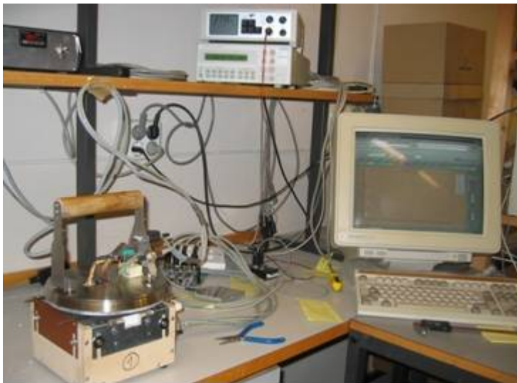
Figure 7 New heat source, a black hotplate, with a temperature of 300^\circ\text{C} \pm 1^\circ\text{C} .
