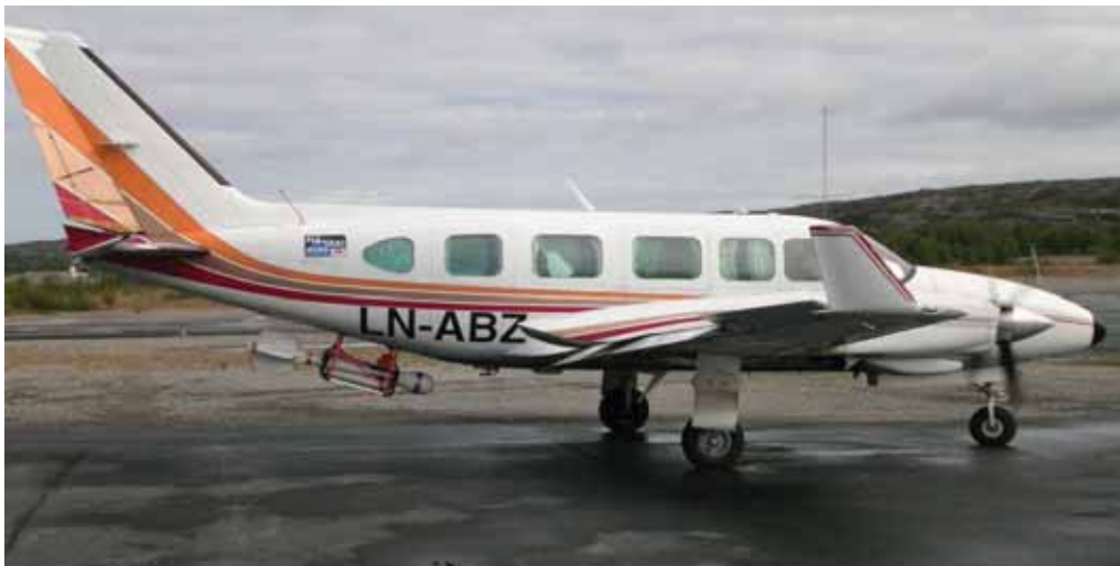
Figure 2.1 Piper Chieftain from Fly Taxi Nord with the docking cradle for the bird containing a Scintrex Cesium Vapour MEP 410 high-sensitivity magnetometer.
