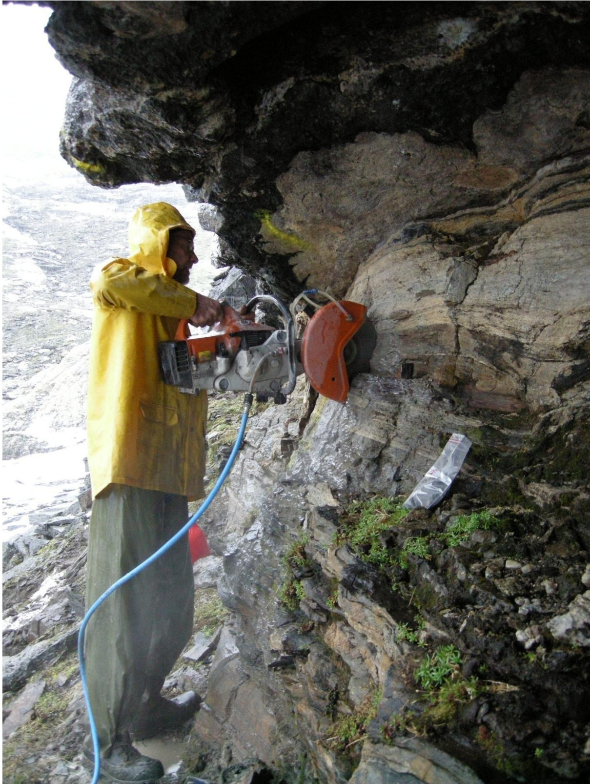
Figure 2: Channel sampling by hand held rock saw. Cutting of the uppermost part of Profile 3 at Locality 2.
