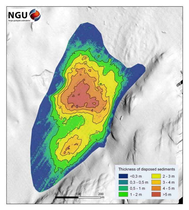
Figure 19. Thickness of disposed sediments in the CDF. Calculated thicknesses include corrections for settling of the original seabed and the offset (5 cm) between the 2004 and 2008 bathymetric datasets. Shaded-relief image of the 2008 dataset is given at the background.
