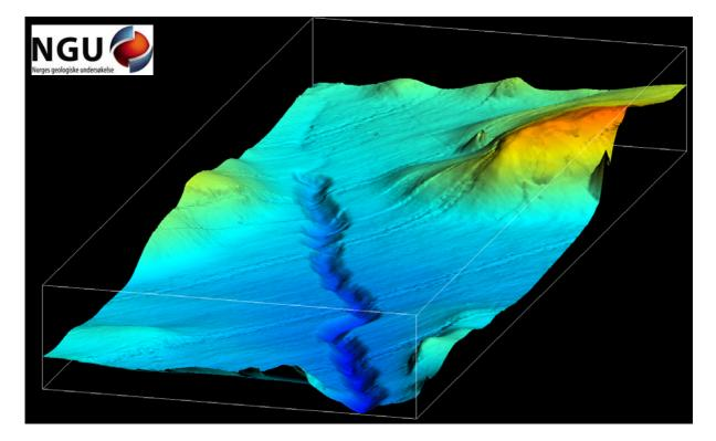
Figure 4. Depth-colored shaded-relief 3D model of a composite pockmark above the fault/permeable fracture cutting the bedrock of the Bekkelag Basin. The diameter of individual pockmarks within the composite pockmark is ca. 60 m, and the depth is ca. 6m. See Fig. 2 for location.
