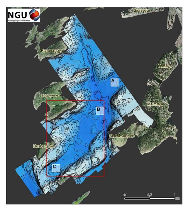
Figure 9. Depth-colored shaded-relief image with depth contours of the area of the Bekkelag Basin mapped in 2008. The red rectangle shows the position of the CDF area shown in Fig. 10. White rectangles outline reference areas A, B and C that were used for assessing the match between the 2004 and 2008 datasets (Fig. 13).
