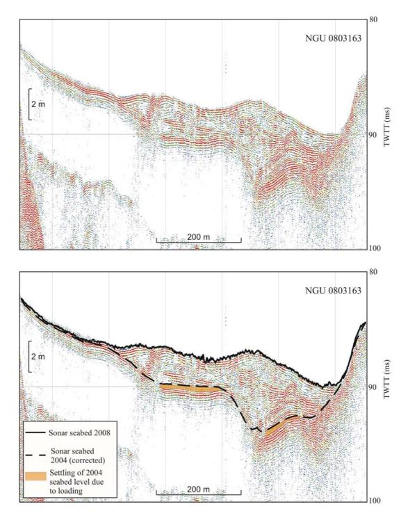
Figure 15. TOPAS seismic reflection profile (NGU0803163) across the CDF. Lower panel includes seafloor elevation lines from the 2004 and 2008 sonar datasets. Location of the profile is given on Fig. 6.
