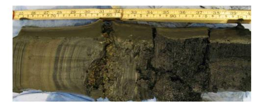
*Figure 18. Gravelly interlayer (at 80 cm) within finely banded/laminated, disposed sediments in core 0803030.*
