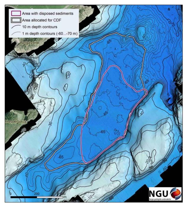
Figure 10. Depth-colored shaded-relief image with depth contours of the CDF area in April 2008.
