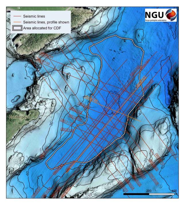
Figure 6. Locations of TOPAS shallow seismic profiles in the area of the CDF.
