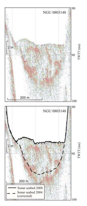
Figure 14. TOPAS seismic reflection profile (NGU0803148) across the CDF. Lower panel includes seafloor elevation lines from the 2004 and 2008 sonar datasets. Location of the profile is given on Fig. 6.
