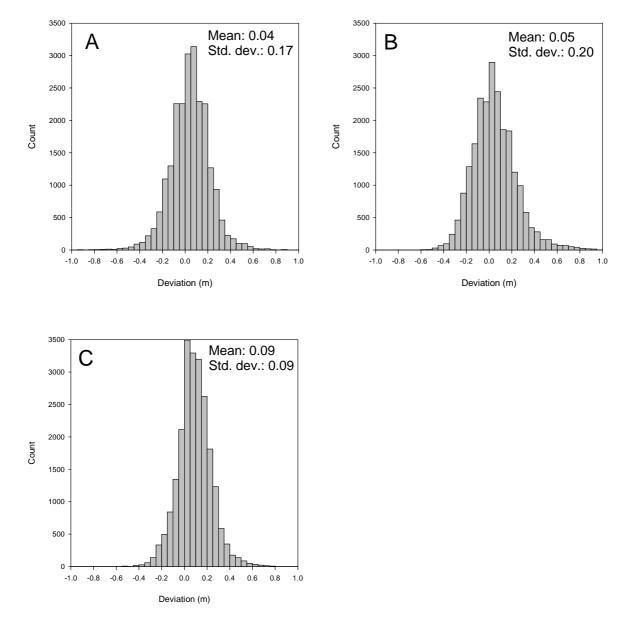
Figure 13. Histograms of seabed elevation differences between the 2004 and 2008 datasets in three reference areas of 22871  $m^2$  each (Fig. 9).
