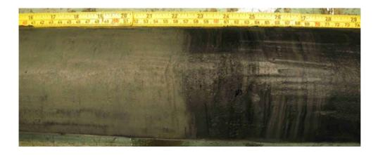
Figure 17. Contact between disposed sediments and natural sediments (at 63 cm) in gravity core 0803028. Gray to black disposed sediments (right hand part of the core), mainly mud, are commonly banded/laminated and contain sandy and gravelly interlayers. Natural olive gray mud (left hand part of core) is typically homogeneous, bioturbated, and has ca. 5 cm black, organic-rich layer at the top (57-63 cm).
