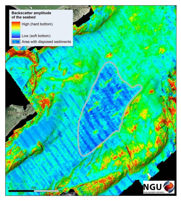
Figure 11. Backscatter amplitude of the seafloor allows outlining of the area covered with disposed sediments. The disposed sediments have typically low backscatter amplitude due to their very soft nature.
