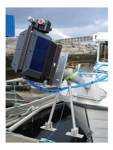
Figure 5. Sonar head with dual transducers mounted at 30 degrees to the vertical. The red device at the top of the photo is a single beam echosounder whereas the device at the side of it is a sound velocity probe.
