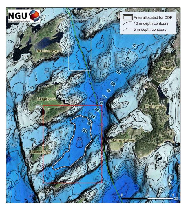
Figure 2. Depth-colored shaded-relief image with depth contours of the Bekkelag Basin in 2004. The red rectangle gives the position of the CDF area shown in Fig. 3. Green dashed line shows the location of a major fault/permeable fracture that cuts across the Bekkelag Basin. Pockmarks, illustrated by the 3D model from the area of the white rectangle (Fig. 4), are common along this fault.
