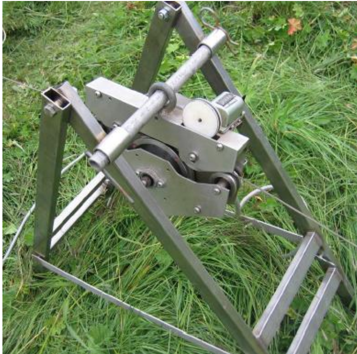
Figure 5.4. The electronic depth counter. An additional mechanical counter is also used (on top of the unit with the small white wheel).
