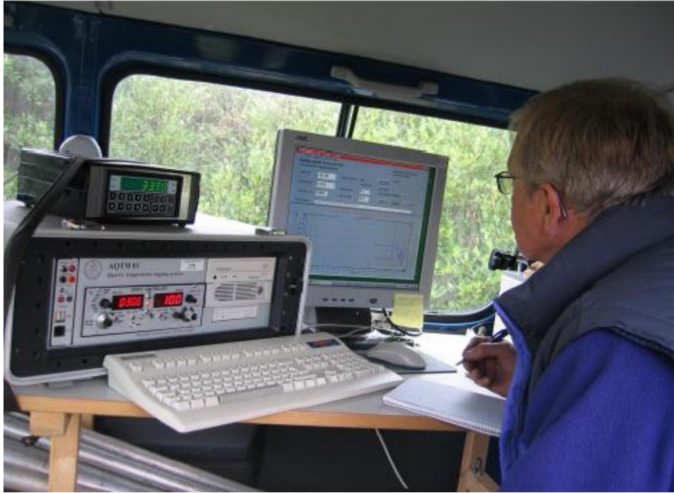
Figure 5.5. The electronic unit. Measured temperatures together with other recorded parameters (depth, weight of probe and cable and logging speed) can be followed in real time on the screen.
