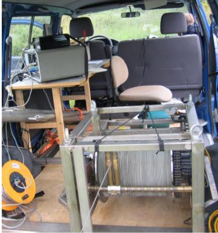
Figure 5.3. The logging winch is installed inside the logging car together with the electronic steering and recording unit.
