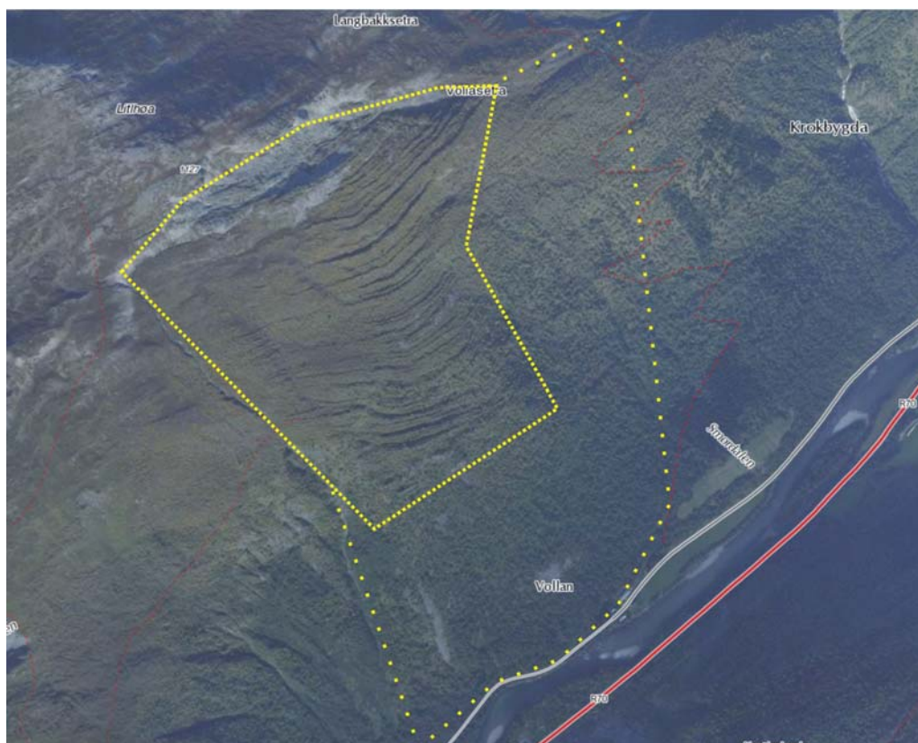
Figure 15. Aerial photograph of the Vollan site with indications of minimum and maximum boundaries of the slope instability. ( www.norgebilder.no )
