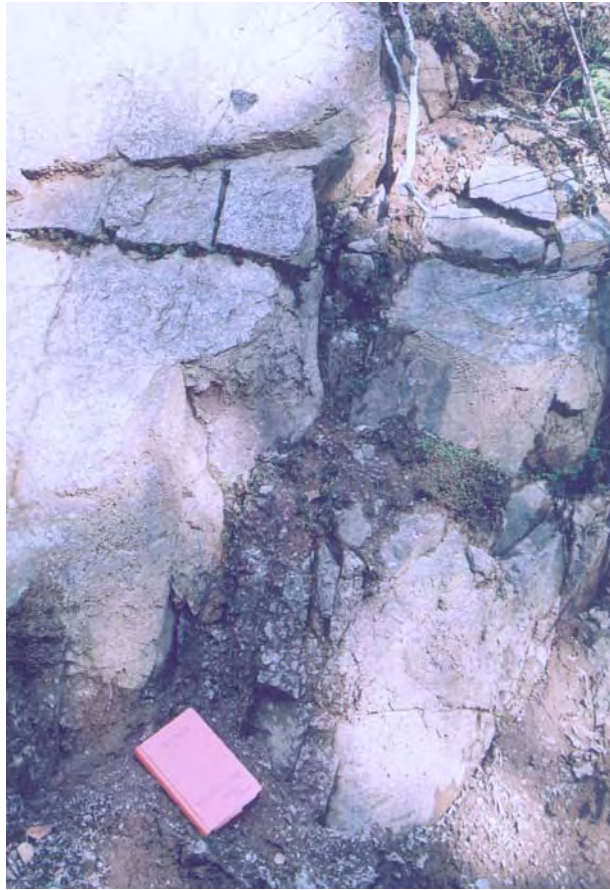
Figure 32. E-W crushed, brecciated and striated fault (strike and dip angle 252/87 and pitch 86E) at the reactivated southern border of an E-W mafic dyke (along the Svartebekk river, site18).
