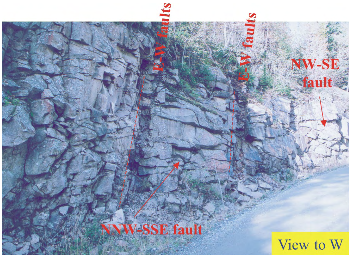
Figure 23. Photos of a highly fractured outcrop with E-W faults and NW-SE / NNW-SSE normal faults (site 14). The E-W faults show up to 40 cm-thick crushed zone.
