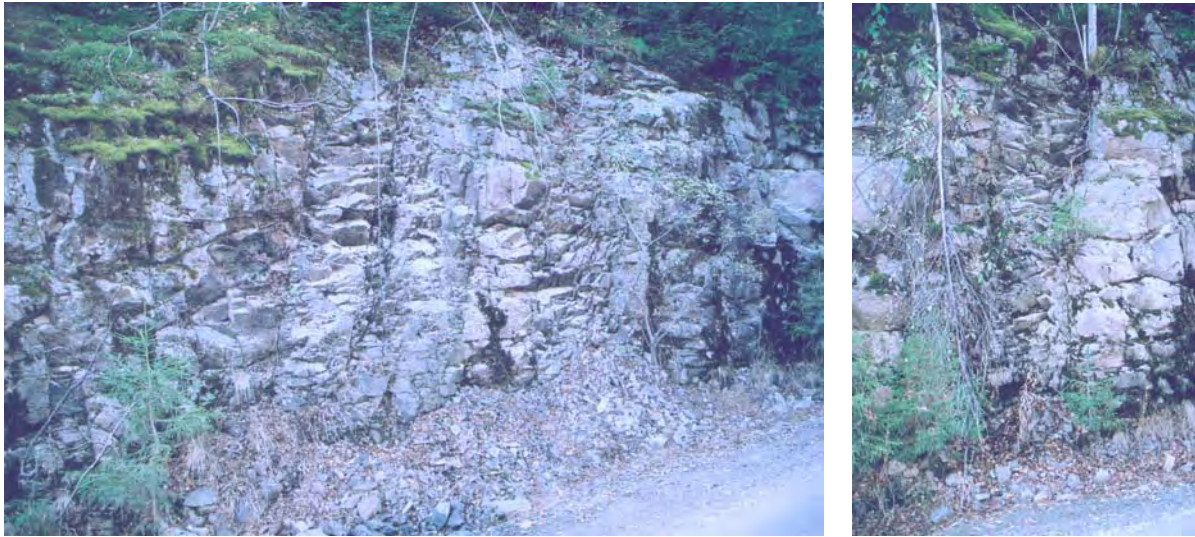
Figure 28. Example of NW-SE mafic dykes along the Sagdalen valley (site 11). Close to a large NW-SE lineament, the density of dyke increases to reach about 5 per 10 m. The picture to the right shows the high density of open joints within the dyke (compared to syenite host rock and with more than 9 fractures /m).
