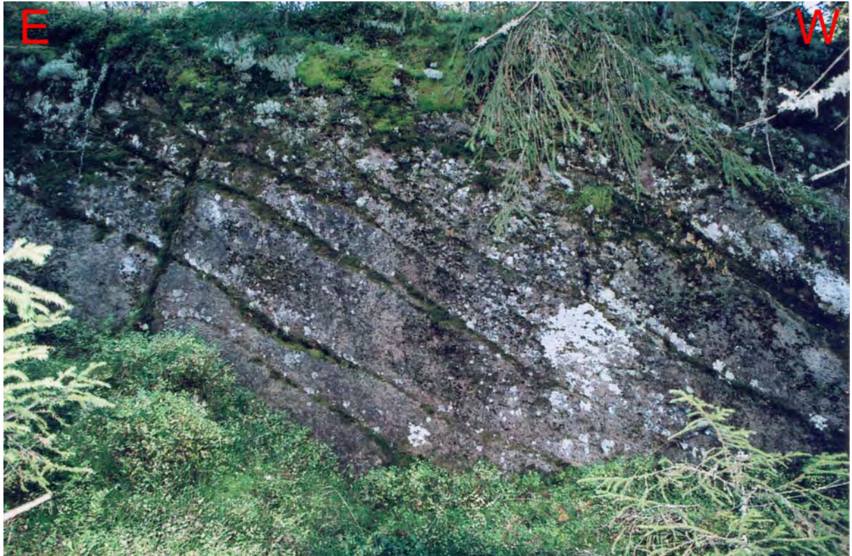
Figure 16. Example of shallow west-dipping joints, 1 m spaced, and large steep E-W trending joints (the front side of the outcrop) (site 9).
