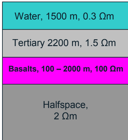
Figure 3.20 Simple model used for 1D modelling of variable thickness in the basalts.
