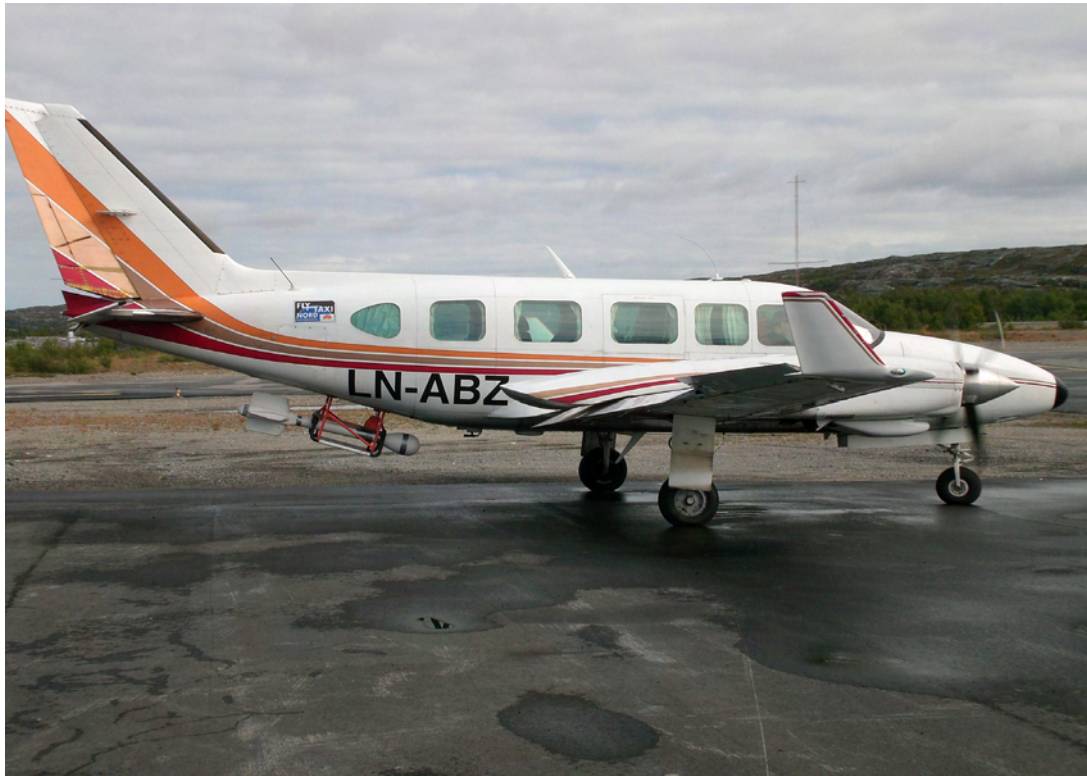
Figure 2.2 Piper Chieftain from Fly Taxi Nord with the docking cradle for the bird containing a Scintrex Cesium Vapour MEP 410 high-sensitivity magnetometer.
