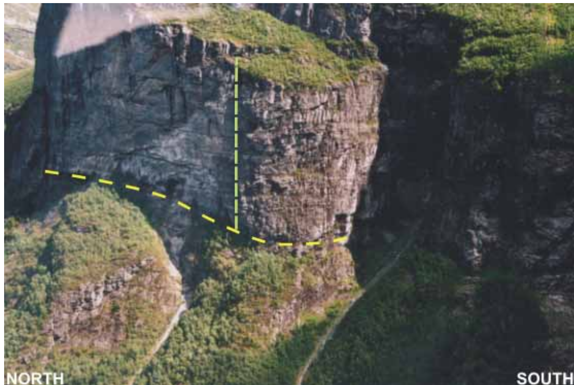
Figure 41: Development of a dense network of joints in a potentially unstable block at site 16. The steep, open fractures (a major one shown in green) appear to detach onto a shallow, fjord-dipping discontinuity (yellow).
