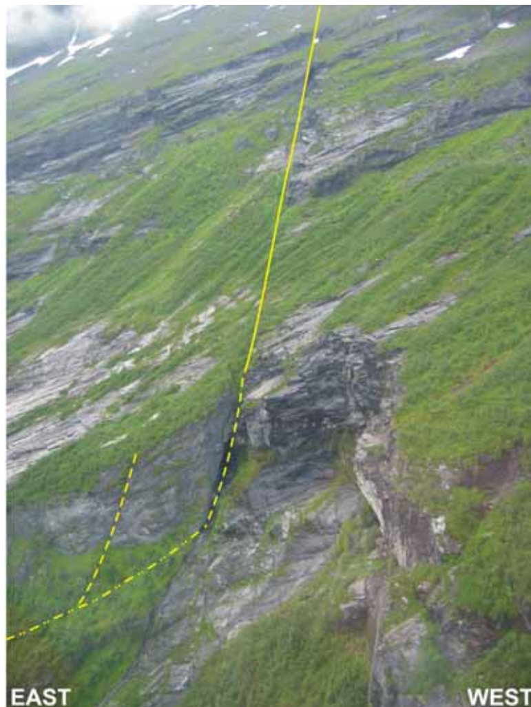
Figure 27: Site 10b seen from the air. Clearly visible are the foliation gently dipping towards the fjord and the back extensional fracture (dashed line on right), which appears to be an inherited north-south lineament (solid line).
