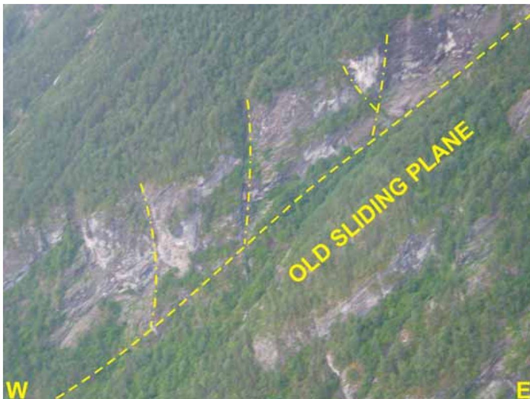
Figure 5: Structures observed from helicopter at Site 2. It was not possible to land at this site.
