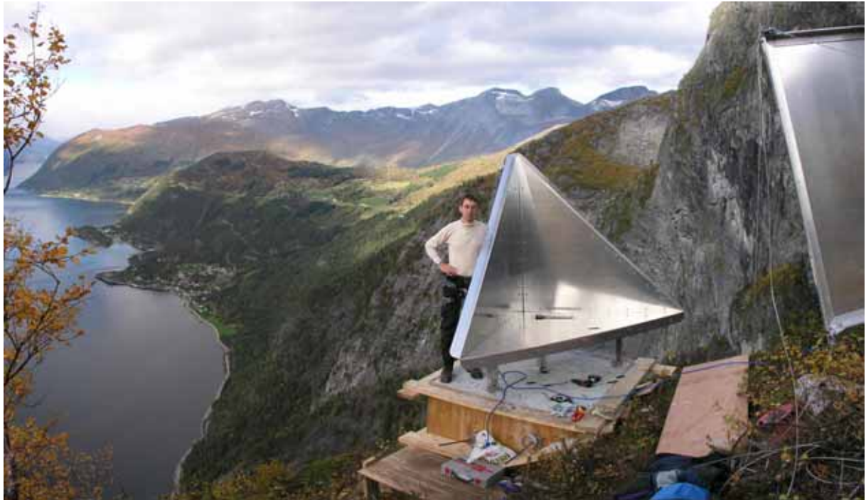
Figure 17. Artificial corner reflector installed near Tafford, in Norway. The reflector is constructed of 10mm thick aluminum.
