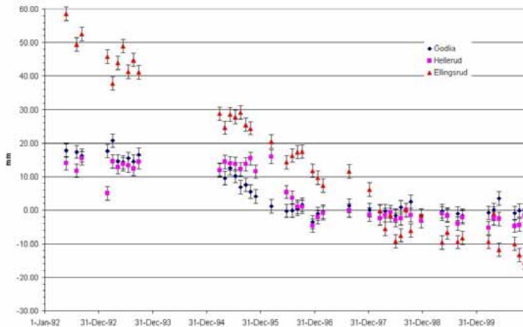
Figure 23. Displacement-time series for selected houses along the trace of the Romeriksporten tunnel. Accelerated subsidence in Hellerud and Godlia coincides with the time of tunnel construction in those areas. The subsidence in Ellingsrud shows no acceleration, as is unrelated to tunnel construction.
