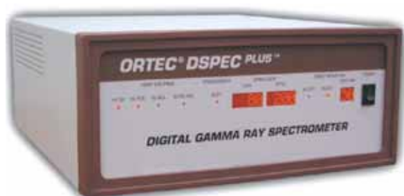
Figure 31. Ortec DSPEC-plus gamma ray spectrometer, front view.
