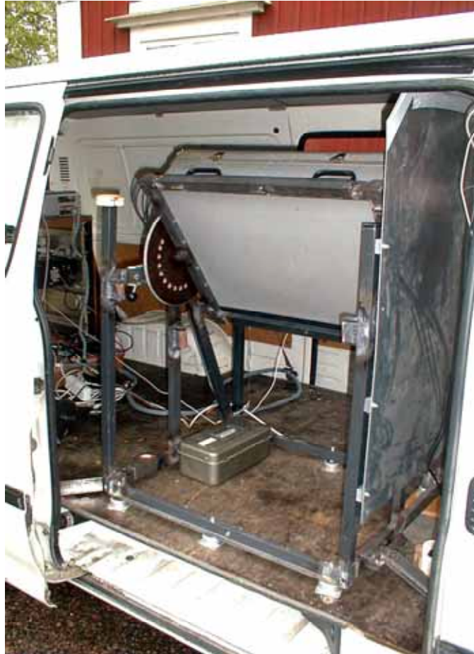
Figure 30. A close-up view of the NaI detector and the frame that supports it. The tilt angle of the detector can be adjusted so that it registers more gamma rays from the roadside than from the road.
