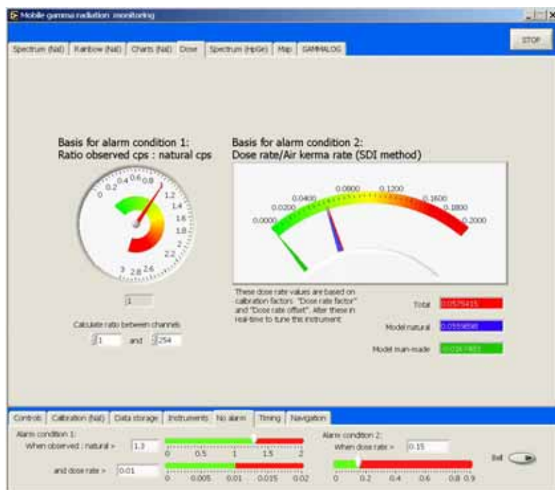
Figure 25. The alarm display consists of the Dose/**Warning: Check Dose!** panel and No Alarm/**Warning: Alarm!** panel. In this case the anthropogenic radiation alarm (alarm condition 1) shows no detectible anthropogenic radiation
