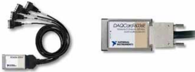
Figure 35. Left: PCMCIA card providing 4 extra serial ports (National Instruments PCMCIA 232/4). Right: PCMCIA Analogue/Digital card (National Instruments DAQ-card 6036E).
