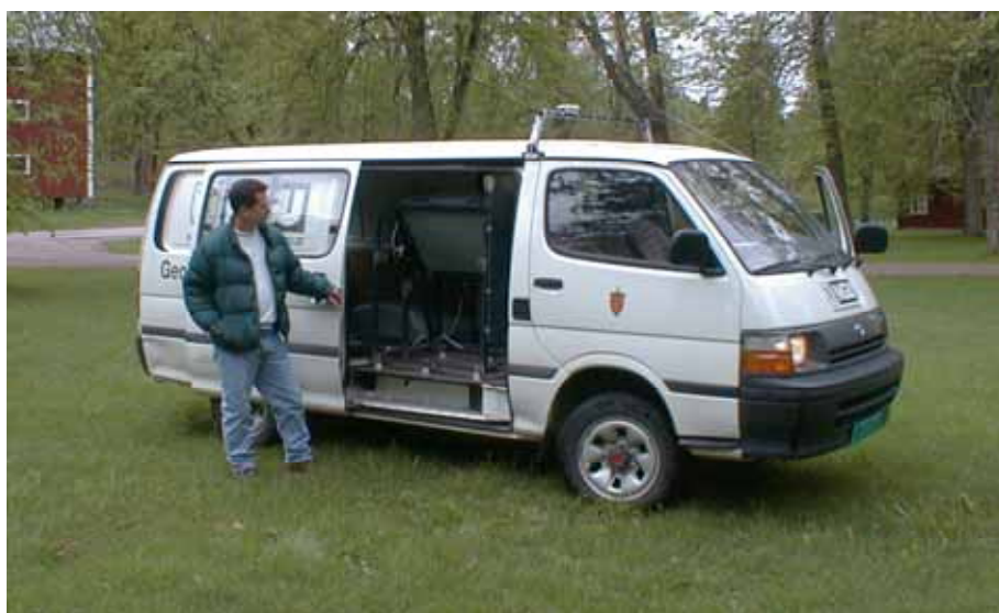
Figure 29. Exploranium GPX 256 NaI detector mounted in a van. A GPS antenna is mounted on the horizontal bar above the roof of the vehicle. Geological Survey of Norway's carborne system.
