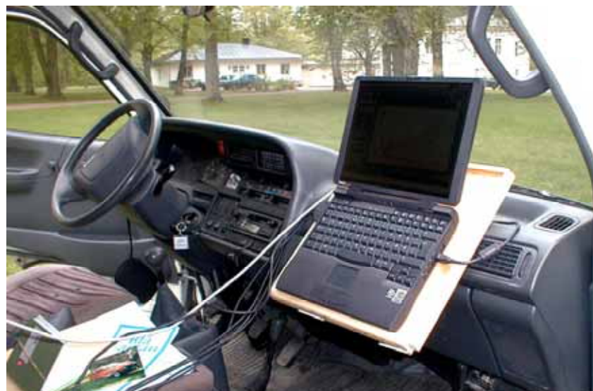
Figure 34. The laptop computer that controls the measuring system mounted in front of the passenger seat. This computer starts and stops the instruments, stores the data on disk, performs real-time processing and displays the data in various graphical forms. The software includes a visual and audio alarm warning of elevated radiation levels.
