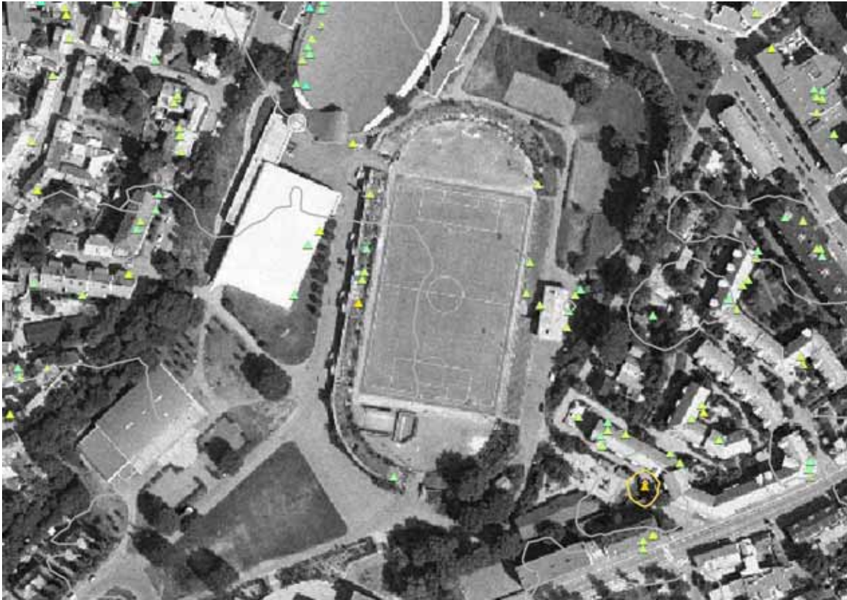
Figure 36. There is no evidence of subsidence in the area around Jordal Amfi.
