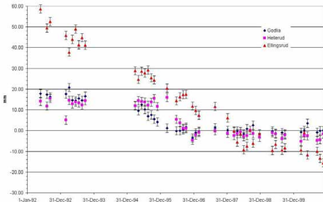
Figure 3. Displacement-time series for selected houses along the trace of the Romeriksporten tunnel. Accelerated subsidence in Hellerud and Godlia coincides with the time of tunnel construction in those areas. The subsidence in Ellingsrud shows no acceleration.
