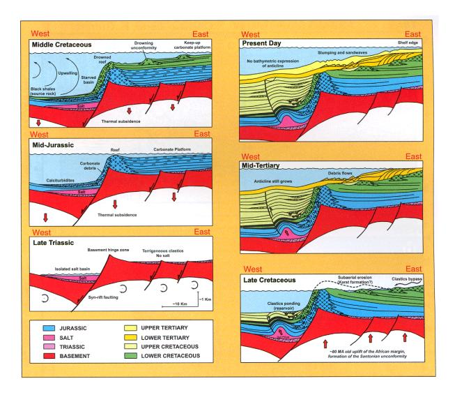
Fig. 4.4. Sequential restoration of a regional seismic profile (transect 7a in Fig. 4.2). Salt was deposited west of the basment hinge zone in Late Triassic – Early Jurassic time, and deformed in Santonian time during uplift and erosion east of the hinge zone. From Tari et al. (2003).
