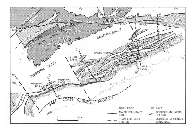
Fig. 3.3 Structural elements map of the Nova Scotia margin. Salt basins are marked with hatchured pattern. From Welsink, Dwyer & Knight, 1989.
