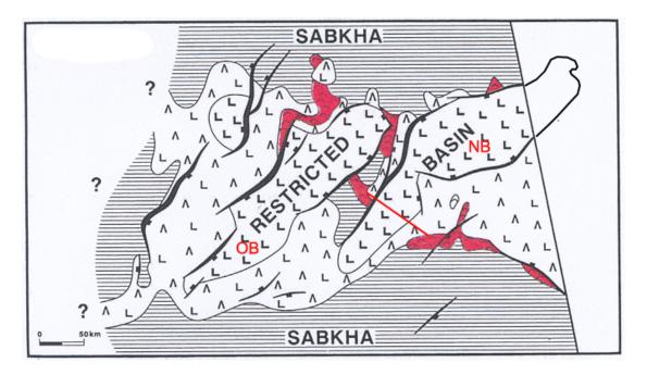
Fig. 1.1 Distribution of the main evaporite facies in the SW Barents Sea. L-symbol = halite, ^ = anhydrite. NB= Nordkapp Basin, OB = Olga Basin. The red line marks the position of a geoseismic profile, shown in Fig. 1.3. Red areas are local carbonate build-ups, generally interpreted as bioherms/reefs. (From Gérard & Buhrig, 1990).
