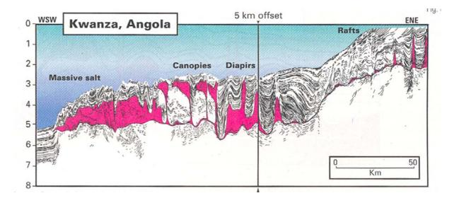
Fig. 5.4. Geoseismic section from the Kwanza Basin, Angola, illustrating the typical domains of salt structuring observed along the West Africa margin. Extensional structures, including large rafts, characterize the updip portion of the margin, while complementary compressional structures mark the lower part of the margin. Salt has been displaced basinward during buildup of the post-salt succession. See Fig. 5.2 for profile location (Transect C). From Tari et al. (2003).
