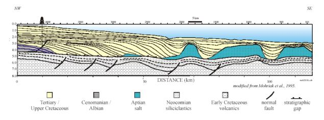
Fig. 5.3. Geoseismic profile from the Santos Basin, Brasil, illustrating how prograding sediments progressively have pushed the salt basinward. From Mohriak et al., (1995).
