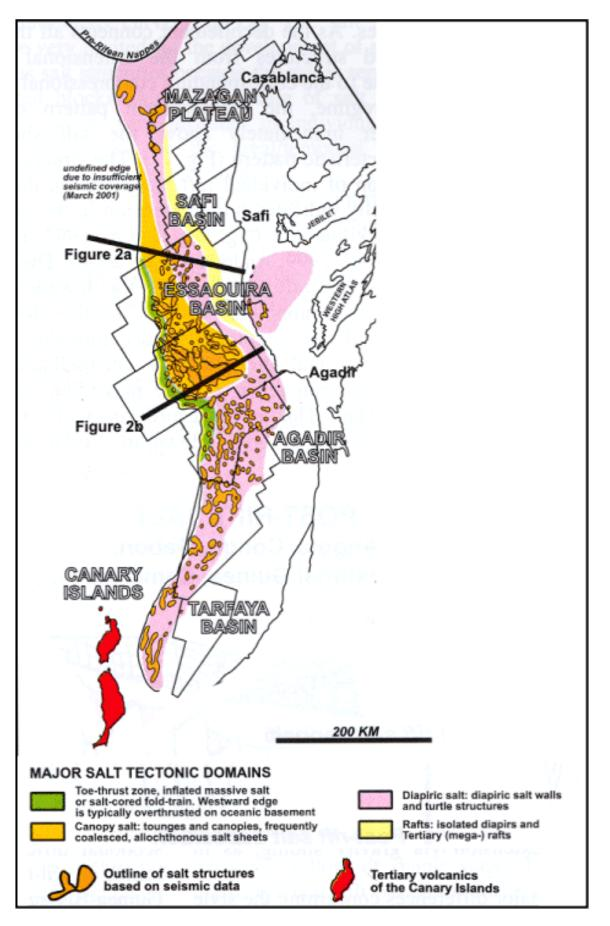
Fig. 4.1 Map of salt distribution and styles of salt deformation off Morocco. From Tari et al. (2003).
