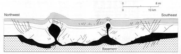
Fig. 1.3 Geoseismic profile across SW Nordkapp subbasin. Note the drop-shaped diapirs. From Nielsen et al (1995).
