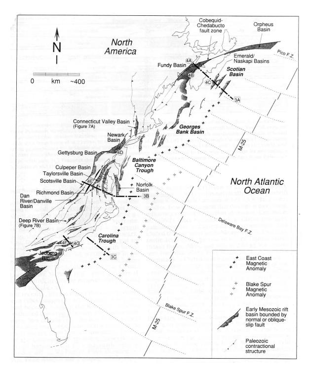
Fig. 3.4 Tectonic features map of eastern US and maritime Canada highlighting major Palaeozoic compressional structures and Mesozoic extensional structures. The heavy + symbols signify the East Coast Magnetic Anomaly, which correlate will the seaward-dipping reflector sequence (Holbrook & Keleman, 1993).
