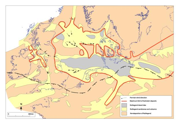
Fig. 2.1 Map of extent of Permian evaporite basin in southern North Sea (red line). Gray area is Rotliegend desert lake, yellow sandstones and volcanics, and light brown areas of no Rotliegend deposition. From Glennie et al. (2003).
