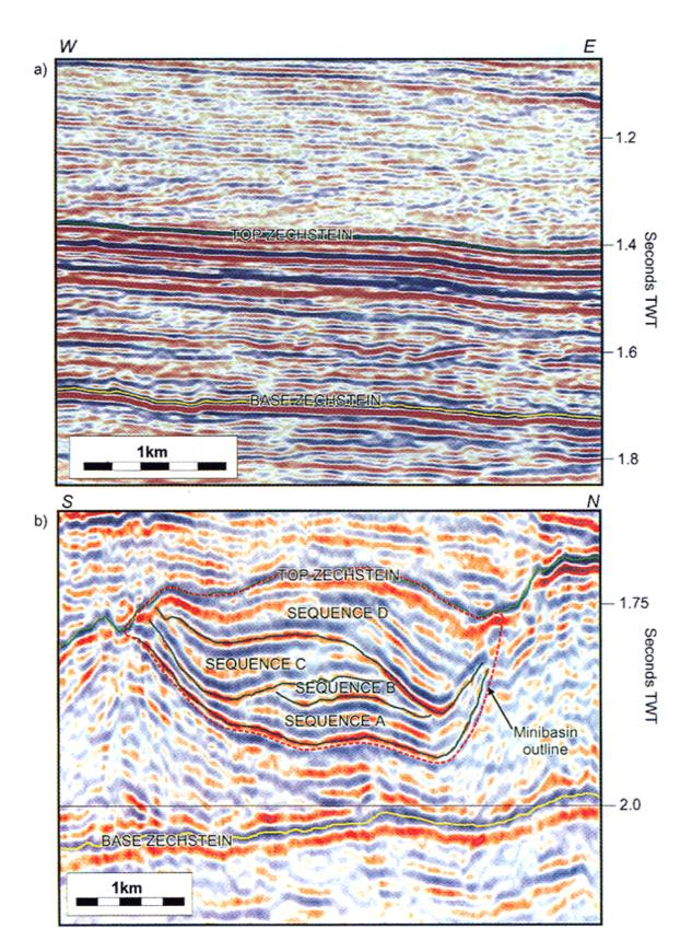
Fig. 2.5. Top section = undeformed example of the Zechstein succession. Lower section = Permian mini-basin. From Stewart & Clark (1999).
