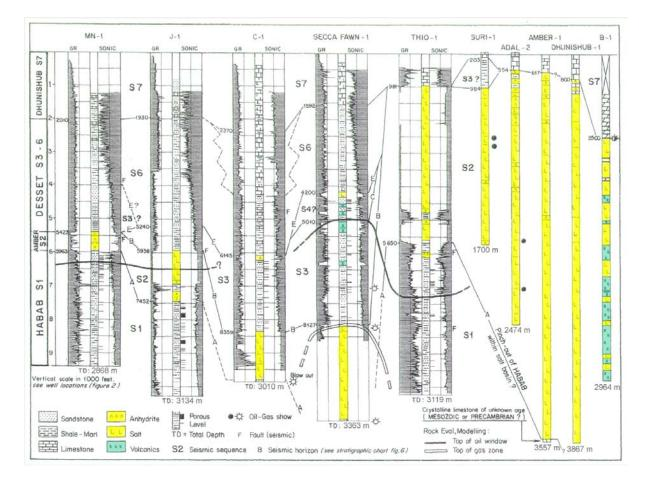
Fig. 6.3. Well logs from the southern Red Sea showing thickness and depth of evaporites (yellow) and volcanics (green). From Savoyat et al. (1989).
