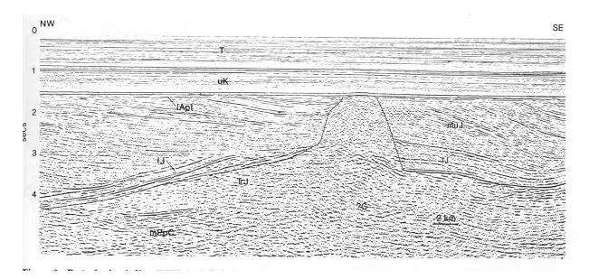
Fig. 3.6 Seismic section across part of the Whale Basin, Grand Banks. TrJ=Argo salt, IJ= Early Jurassic carbonates, Iapt=sub-Aptian unconformity. Note the pronounced rotation of strata below the sub-Aptian unconformity, the truncation of the salt diapir, and the undeformed horizontally bedded Upper Cretaceous and Tertiary strata. From Balkwill & Legall (1989).
