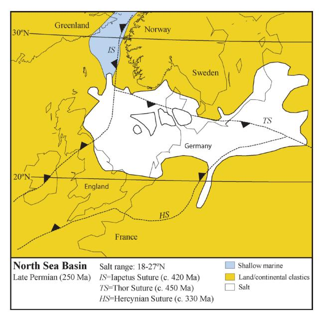
Fig. 2.7 Late Permian (250 Ma) palaeomagnetically constrained plate reconstruction showing the di stribution of Z echstein salt de posits ( $18-27^{\circ}N$ ) and the location of older c ollisional sutures.
