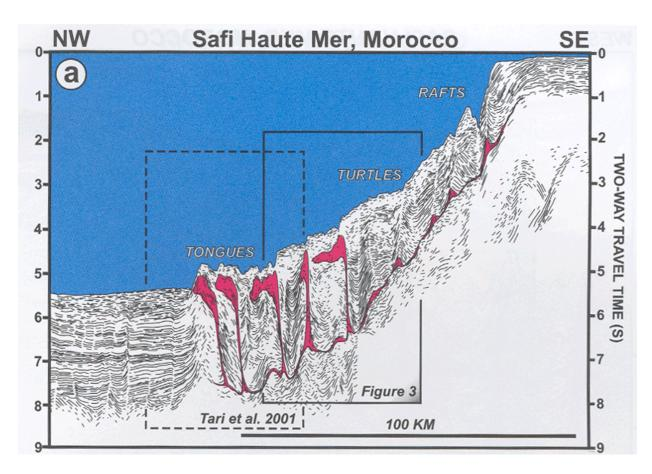
Fig. 4.5 Geoseismic profile across the Safi Haute Mer area offshore Morocco. See Fig. 4.1 for profile location (profile 2a). The profile shows a linked system of post-salt deformation, with updip extension and downdip compression. From Tari et al. (2003)
