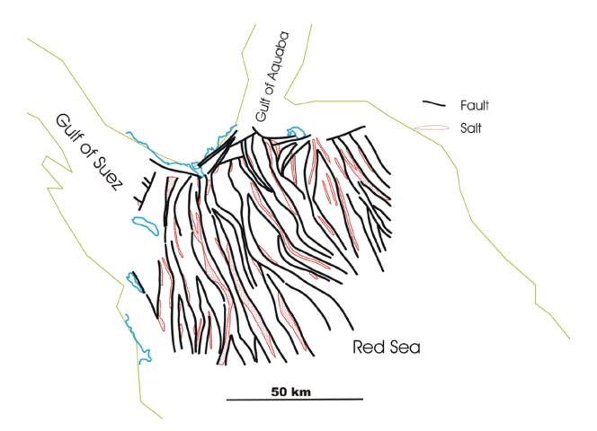
Fig. 6.5. Linear diapiric salt walls parallel to and closely associated with grabens and half grabens produced by ongoing extension in the northern Red Sea. After Mart & Ross (1987).
