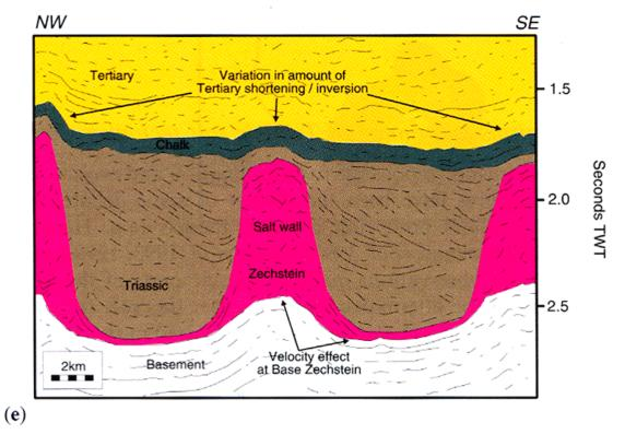
Fig 2.6. Seismic (top) and geoseismic section of Triassic mini-basin. From Stewart & Clark (1999).
